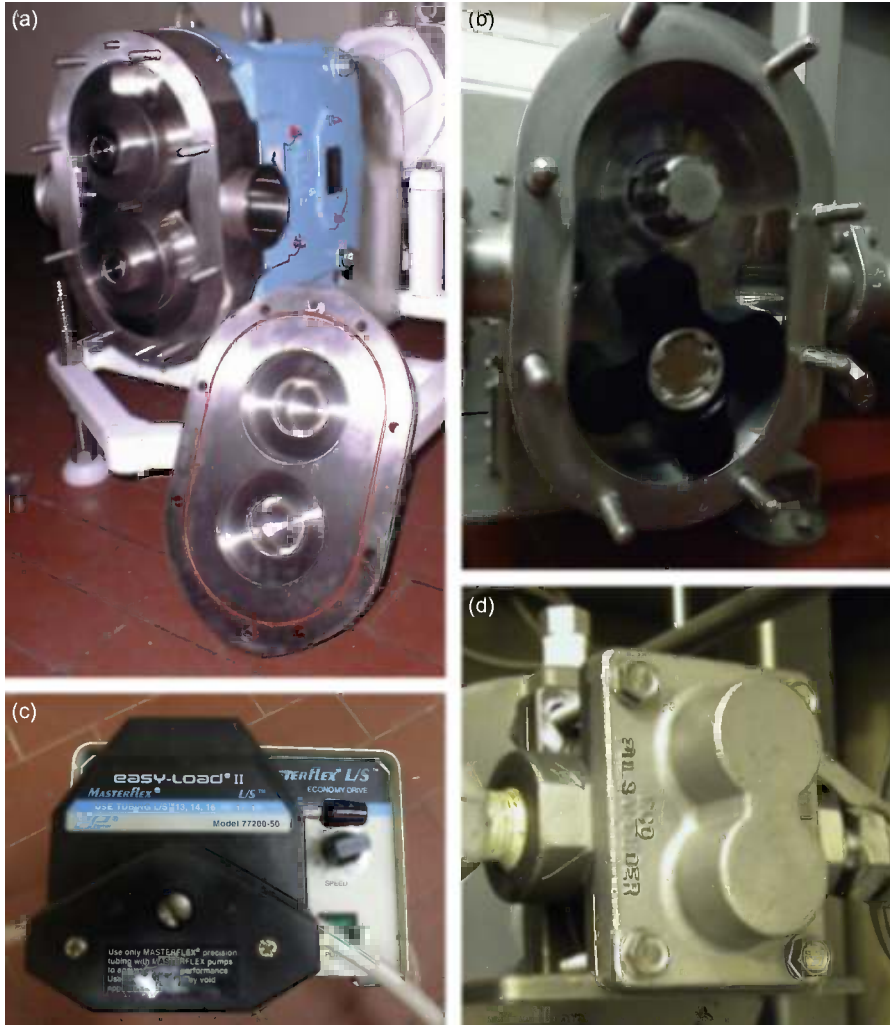
Figure 22.2 Positive displacement pumps (a) rotary piston, (b) rotary lobe, (c) tubing, (d) gear.
