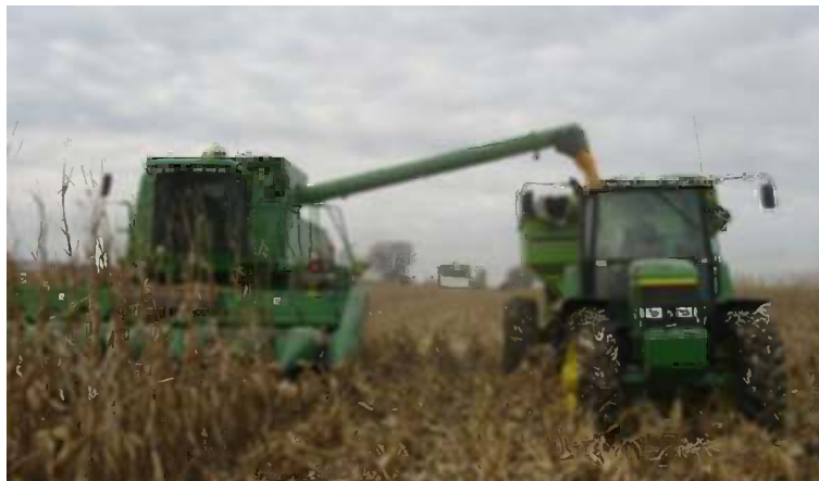
Figure 6.13 Unloading auger extending and moving grain to transport cart.
