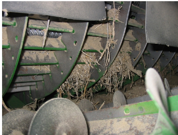
Figure 6.6 Rear of concave underneath cylinder (note clean grain augers underneath in foreground).
