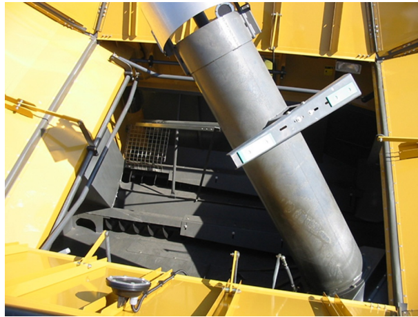
Figure 6.12 Large capacity grain tank with extensions on upper perimeter.
