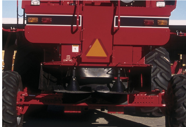
Figure 6.14 Rotary stalk spreaders on rear of combine. (Courtesy of CaselH)
