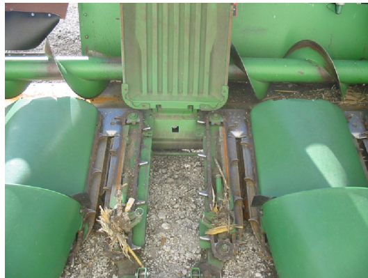
Figure 6.3 Gathering chains and stripper plates over stalk rolls (middle snout is raised).
