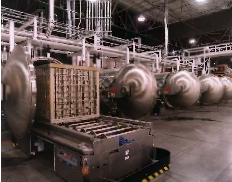
Figure 17.23 Automated guided vehicle in process of retort loading/unloading. (Photo courtesy of JBT FoodTech, formerly FMC FoodTech, Madera, CA)
