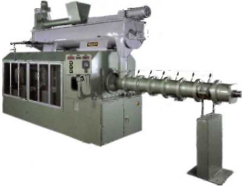
Figure 16.3 Dry extruder with preconditioner.
