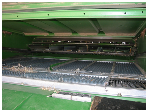
Figure 6.10 Top sieve (chaffer) in cleaning shoe as viewed from rear of combine.
