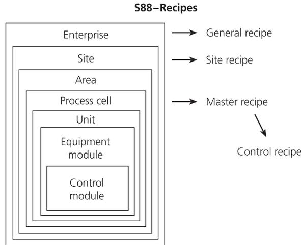
**Fig. 10.4** Illustration of a structure for recipes on enterprise and control levels according to ANSI/ISA-S88 standard. By permission of Tetra Pak processing system AB, Lund, Sweden.
