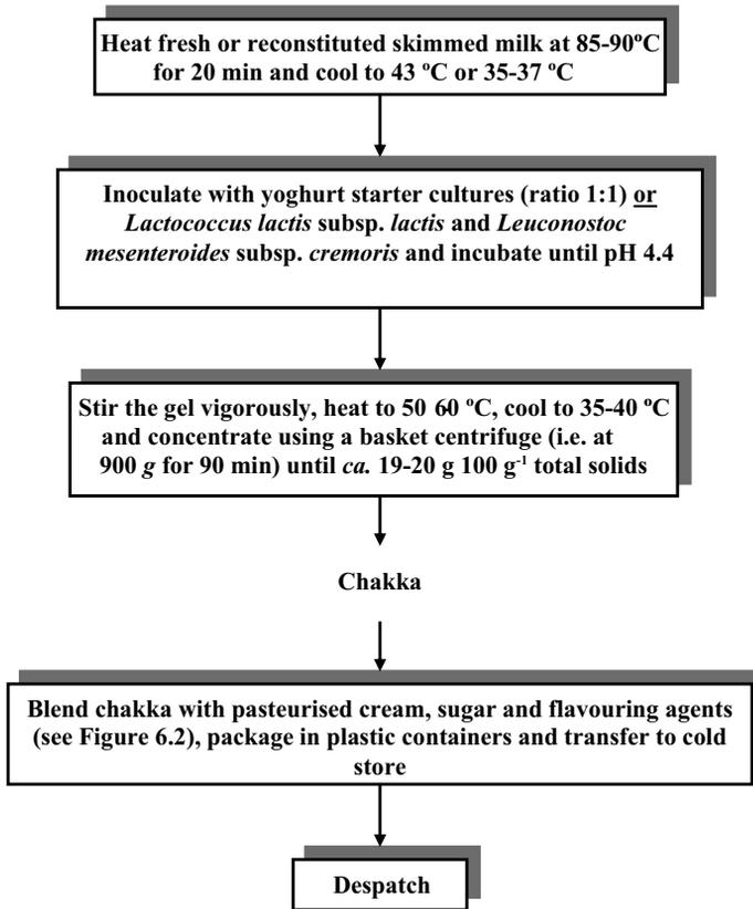
**Fig. 6.7** Production line for shrikhand using basket centrifuge.
