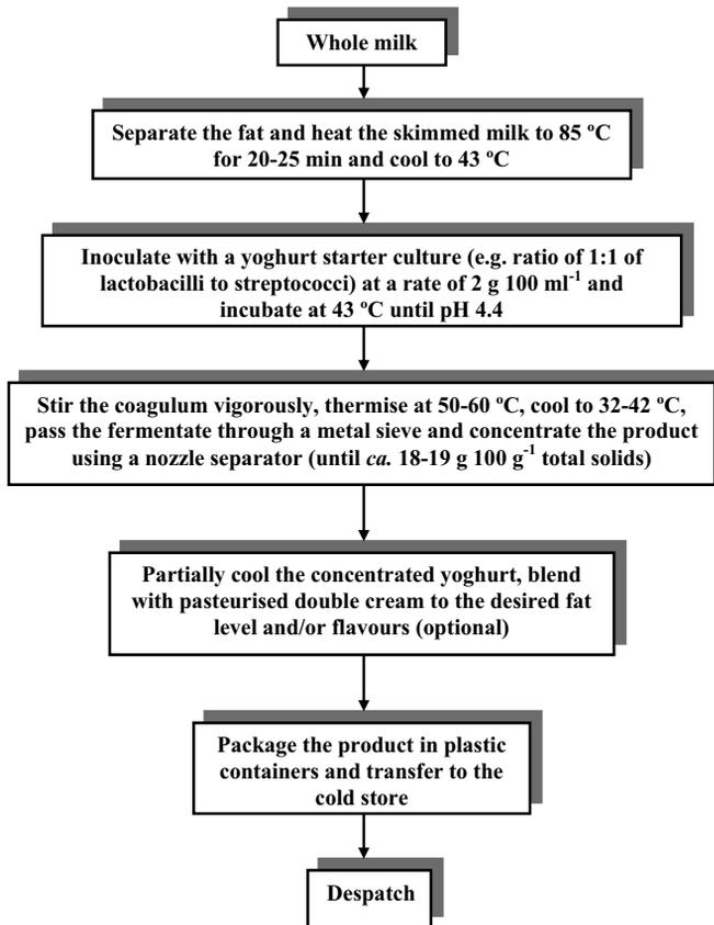
**Fig. 6.3** Production of concentrated yoghurt using the nozzle separator method.
