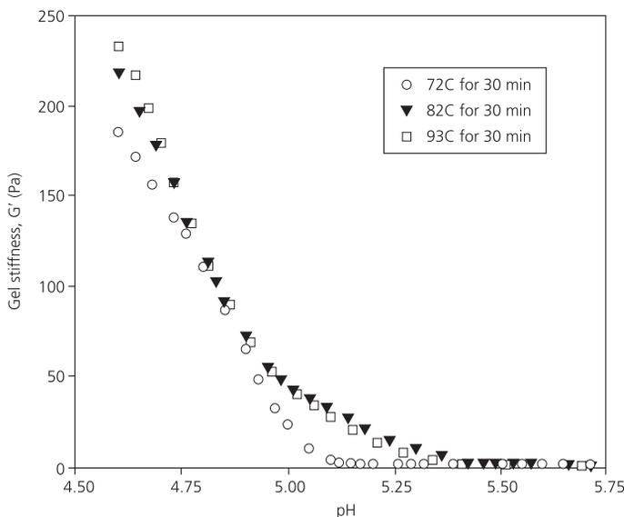
**Fig. 3.10** Effect of different heating temperatures of milk for 30 min on the firmness of yoghurt gels. Reproduced with permission from Lee, W. & Lucey, J.A. (2003) *Journal of Texture Studies*, **34**, 515–536.
