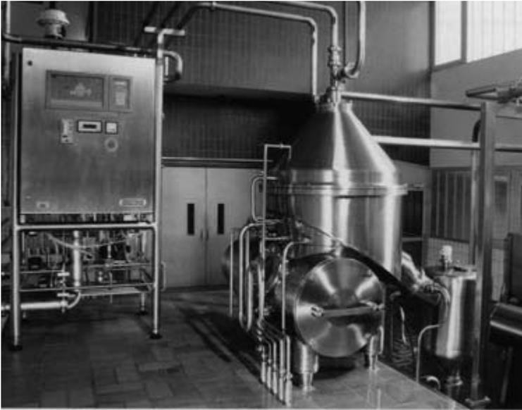
**Fig. 6.5** Production line for thermo-soft cheese showing a nozzle separator type KDB 30. By permission of GEA-Westfalia Separator AG, Oelde, Germany.
