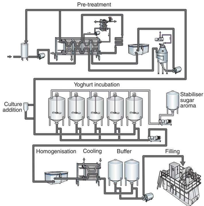
**Fig. 5.5** Production of stabilised fresh drinking yoghurt for storage at 5°C. By permission of Tetra Pak AB, Lund, Sweden.
