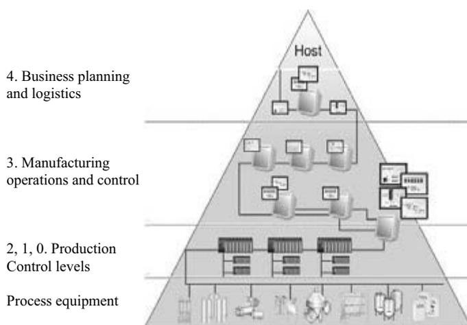
**Fig. 10.1** Overview of the different levels of automation in a yoghurt/food production line. By permission of Tetra Pak processing system AB, Lund, Sweden.
