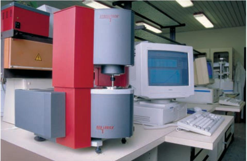
**Plate 5** Stresstech CS rheometer for controlled stress viscosity measurement. With permission of Danisco A/S, Brabrand, Denmark, and Reologica, Sweden.
