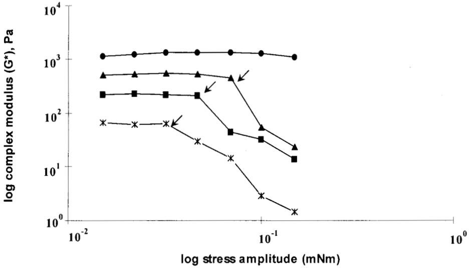
**Fig. 6.12** Effect of the protein concentration on the complex moduli ( $G^*$ ). Protein levels ( $\text{g } 100 \text{ g}^{-1}$ ): \* = 3, ■ = 5, ▲ = 7, ● = 9. Arrows indicate the complex modulus ( $G^*$ ) after the gel structure degraded (i.e. outside the linear viscoelastic region). Reproduced with permission from Özer, B.H., Stenning, R., Grandison, A.S. & Robinson, R.K. (1999b) *Journal of Dairy Science*, **82**, 682–689.
