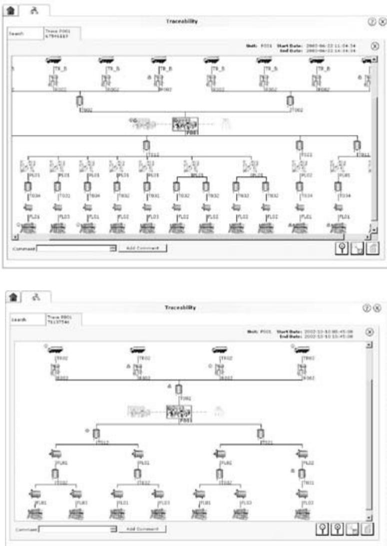
**Fig. 10.8** Two different levels of resolution in traceability, focusing on the pasteuriser. By permission of Tetra Pak processing system AB, Lund, Sweden.
