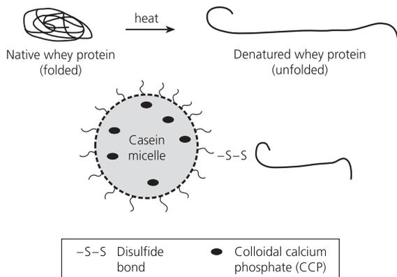
**Fig. 3.6** Schematic diagram of the interaction of whey proteins with caseins due to milk heat treatment (not to scale as  $\beta$ -lactoglobulin is only 2 nm while the average size of casein micelles is  $\sim 150$  nm).
