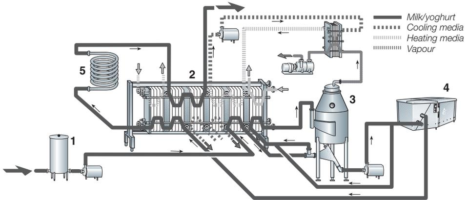
**Fig. 3.2** Flow diagram of general pre-treatment of milk for the manufacture of set and stirred yoghurt. 1, Balance tank; 2, plate heat exchanger (PHE); 3, evaporator; 4, homogeniser; 5, holding tube. By permission of Tetra Pak AB, Lund, Sweden.
