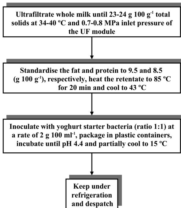
Fig. 6.8 Production of labneh from UF whole-milk retentates.
