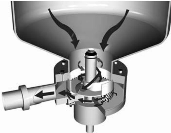
**Fig. 5.6** High shear mixing unit (Tetra Almix) with rotor and stator positioned underneath a water/milk-filled vessel. By permission of Tetra Pak AB, Lund, Sweden.
