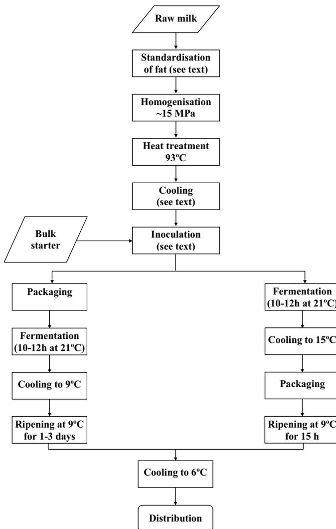
**Fig. 8.9** Generalised scheme for the industrial production of kefir using kefir 'wash' or fermentate as a starter culture.
