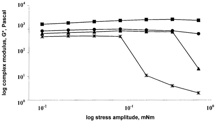
**Fig. 6.11** Complex modulus (G\*) of different types of labneh as a function of amplitude sweep. Total solids contents of all the labnehs averaged 23 g 100 g<sup>-1</sup>. Traditional method (■), ultrafiltration of warm yoghurt (●), fermentation of UF retentate (▲) and direct reconstitution of whole milk powder (\*). Reproduced with permission from Özer, B.H., Stenning, R., Grandison, A.S. & Robinson, R.K. (1999b) *Journal of Dairy Science*, **82**, 682–689.
