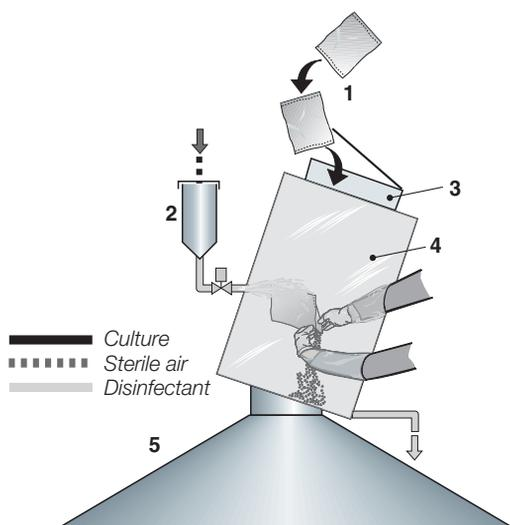
**Fig. 2.10** Hygienic inoculation system fitted on top of a fermentation or bulk starter culture tank. 1, Starter culture package; 2, disinfectant container; 3, sight glass; 4, inoculation 'box'; 5, incubation or bulk starter culture tank. By permission of Tetra Pak AB, Lund, Sweden.
