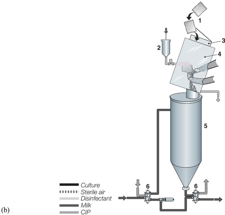
**Fig. 2.9** In-line inoculation system using concentrated freeze-dried or frozen cultures. (a) – 1, Starter culture package; 2, Mixing container; 3, Mix-proof valves. (b) – 1, Starter culture package; 2, Disinfectant container; 3, Sight glass; 4, Inoculation ‘box’; 5, Mixing container; 6, Mix-proof valves. By permission of Tetra Pak AB, Lund, Sweden.
