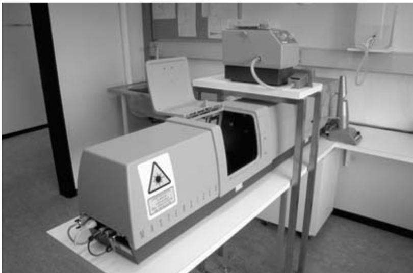
**Fig. 5.15** The Malvern Mastersizer for measuring of particle size distribution. With permission of Danisco A/S, Brabrand, Denmark. Reproduced in colour as Plate 4, after page 110.
