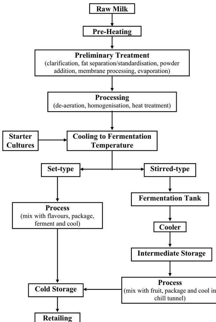
Fig. 1.1 Flow diagram showing the manufacturing stages of fermented milk products.
