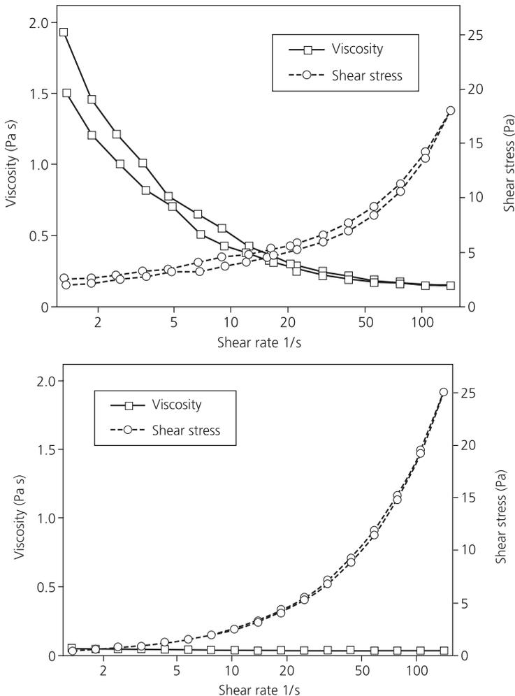
**Fig. 5.17** Flow data of drinking yoghurt (a) with highly shear thinning properties and (b) with nearly Newtonian behaviour. With permission of Danisco A/S, Brabrand, Denmark.
