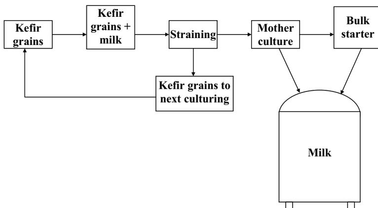
**Fig. 8.7** Production stages for kefir grain preparation and the manufacture of kefir.
