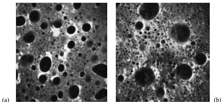
**Fig. 9.4** Confocal laser scanning micrographs of moustes made with Grindsted® mono- and diglycerides (a) and Grindsted® Lactem (b) (lactic acid ester of mono- and diglycerides). The protein structure (i.e. the serum phase) is shown in green and the fat in red and yellow (see coloured plate), while the dark circular patches show the air bubbles. By permission of Danisco A/S, Brabrand, Denmark. Reproduced in colour as Plate 7, after page 110.
