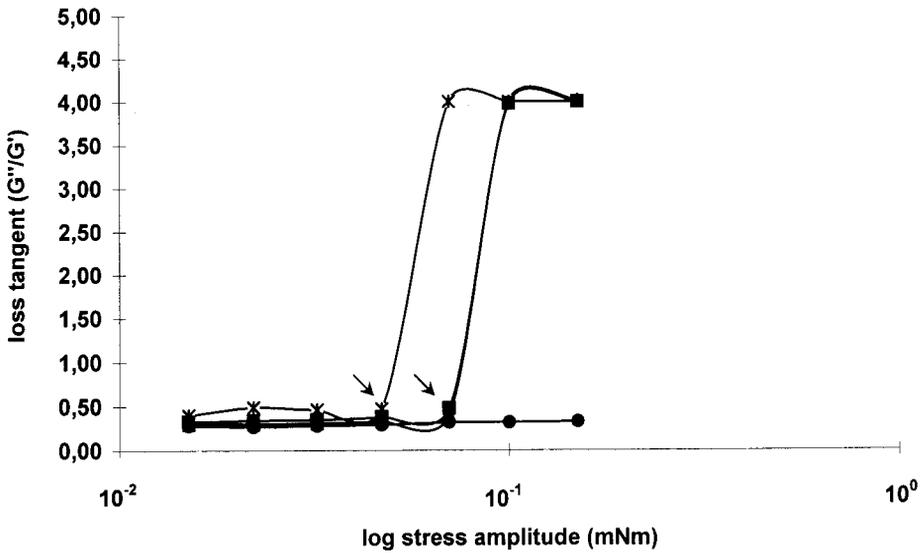
**Fig. 6.13** Effect of the protein concentration on the loss tangent ( $\tan \delta = G''/G'$ ). Protein levels ( $\text{g } 100 \text{ g}^{-1}$ ): \* = 3, ■ = 5, ▲ = 7, ● = 9. Arrows indicate the complex modulus ( $G^*$ ) after the gel structure degraded (i.e. outside the linear viscoelastic region). Reproduced with permission from Özer, B.H., Stenning, R., Grandison, A.S. & Robinson, R.K. (1999b) *Journal of Dairy Science*, **82**, 682–689.
