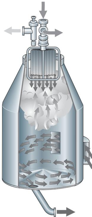
**Fig. 5.8** Flow of milk and air in the vacuum deaerator with built-in condenser. By permission of Tetra Pak AB, Lund, Sweden.
