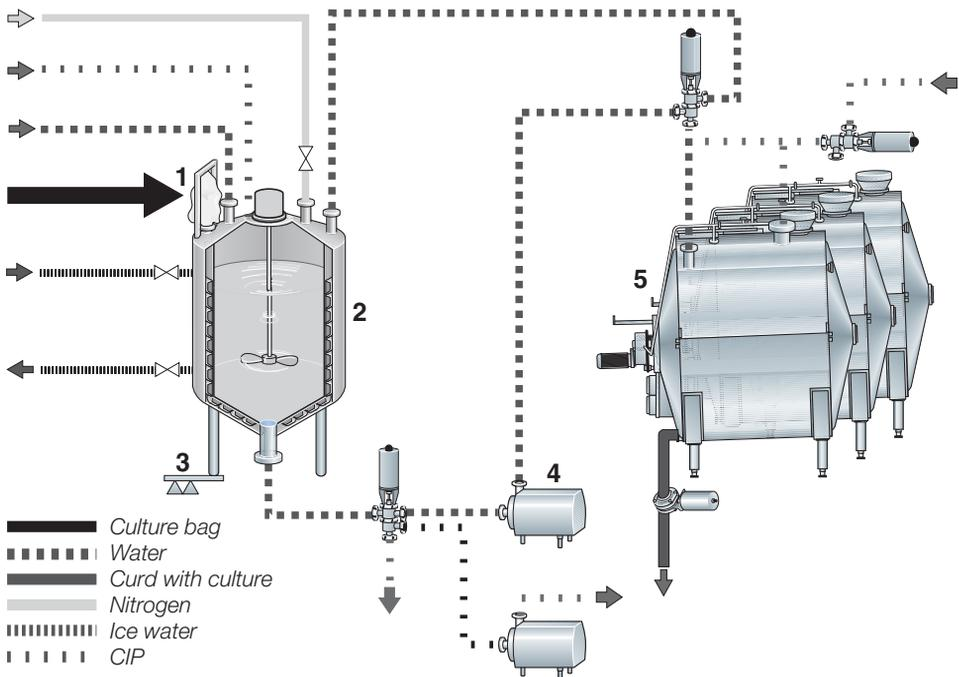
**Fig. 2.11** An illustration of the automatic inoculation system (AISY). 1, Starter culture package; 2, mixing tank; 3, weighing cell; 4, feed pump; 5, fermented milk or cheesemaking tank. By permission of Tetra Pak AB, Lund, Sweden.
