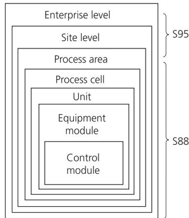
**Fig. 10.2** Illustration of the structure used to model an enterprise according to specific standards (ANSI/ISA-S88 and ANSI/ISA-S95). By permission of Tetra Pak processing system AB, Lund, Sweden.
