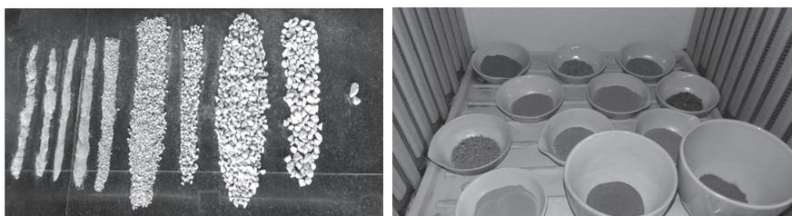
**Figure 4.** Crushed size distribution of the recycled concrete aggregate from a pavement.
