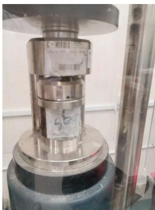
**Figure 1.** Compressive strength test setup.
