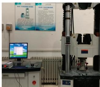
**Figure 5.** Universal testing machine.
