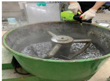
Figure 3. Spray coating RCAs.
