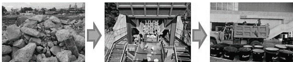
**Figure 3.** Crushing processes to obtain the RCA.
