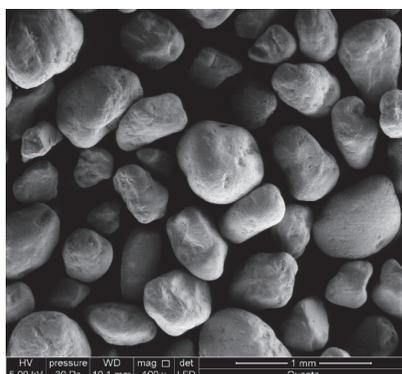
**Figure 1.** Grains of quartz sand.
