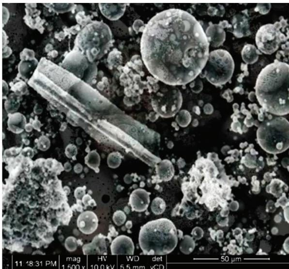
Figure 7. Morphology of calcareous fly ash grains batch B (magnification of 1500 times).
