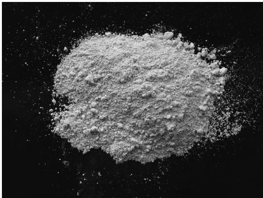
Figure 4.5. General View of High-reactivity Metakaolin.
