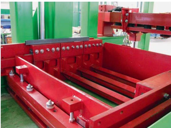
Fig. 3.11: Core-mix feed box with vibrating grate and scraper [3.2]
