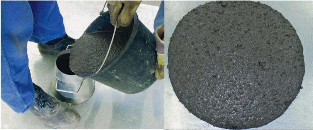
Fig. 1.33: Slump test in accordance with DIN EN 12350-5:2000-06 [1.35]
