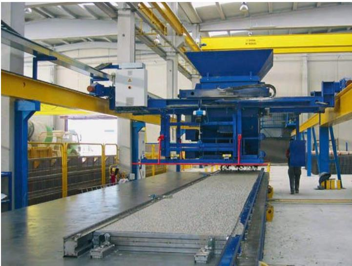
Fig. 1.4: Spatial coupling of process elements: concrete mix spreader above the pallet
