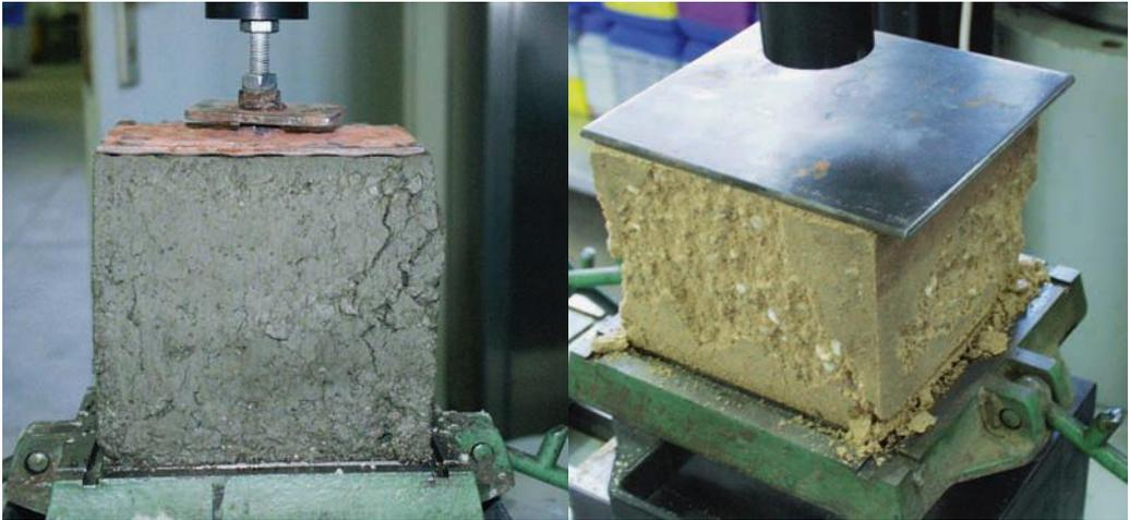
Fig. 1.32: Test specimen after measurement of its green compressive strength
