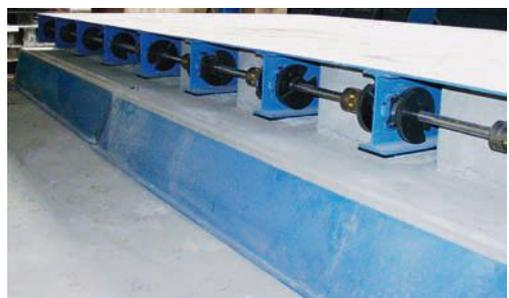
Fig. 5.49: Undulating table in the concrete plant
