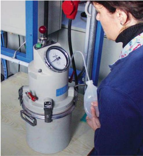
Fig. 1.35: Determination of the air void content of fresh concrete
