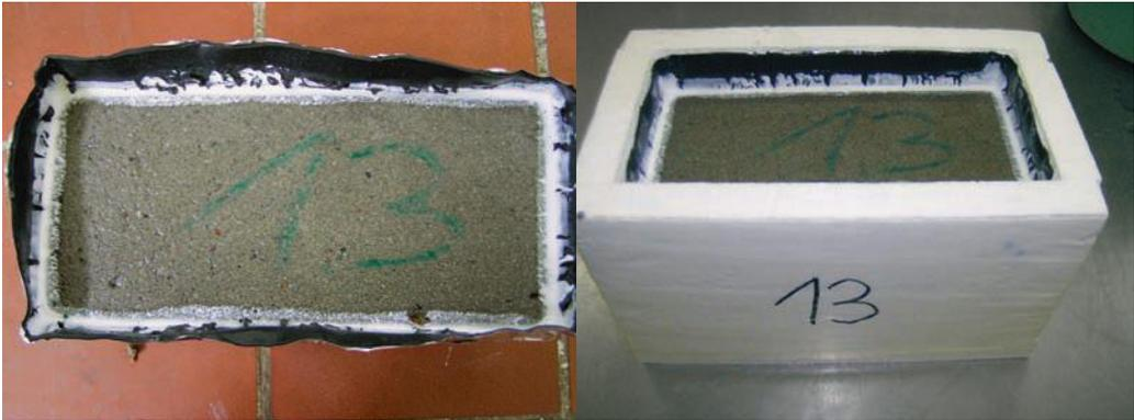
Fig. 1.52: Freeze-thaw resistance test (paving block prior to and after frost test)
