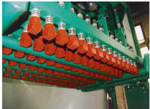
Fig. 3.64: Machine equipped with pointing hammers
