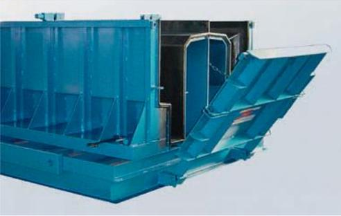
Fig. 5.17: Single mould with a fixed bottom
