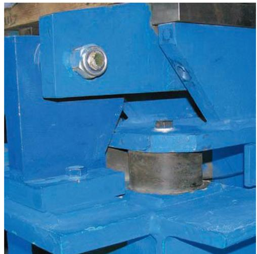
Fig. 3.30: Rubber spring on a vibrating table of a block machine
