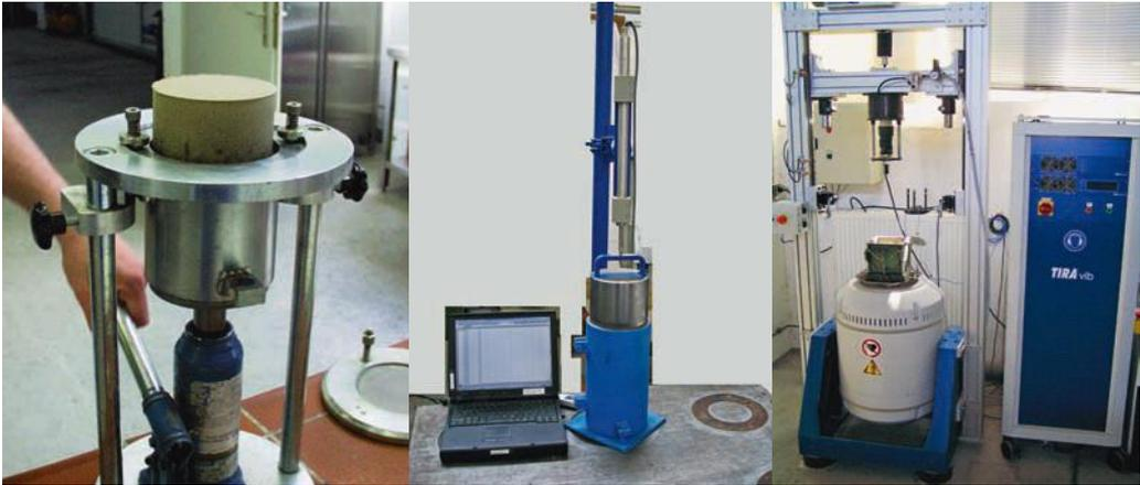
Fig. 1.30: Test equipment to determine the workability characteristics of very stiff concrete mixes (left: Proctor device according to DIN 18127, centre: “vibratory press compaction” set-up according to [1.41], right: electrodynamic TIRA vib vibration test rig at IFF Weimar e. V.)
