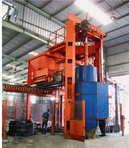
Fig. 4.17: Pipe machine with a rising core
