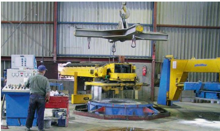
Fig. 4.14: Production line for freshly demoulded large pipes
