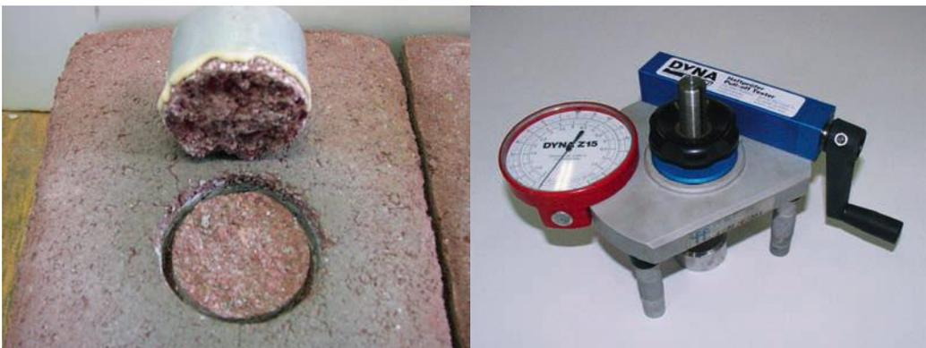
Fig. 1.37: Specimen after the adhesive tensile test and a pull-off tester
