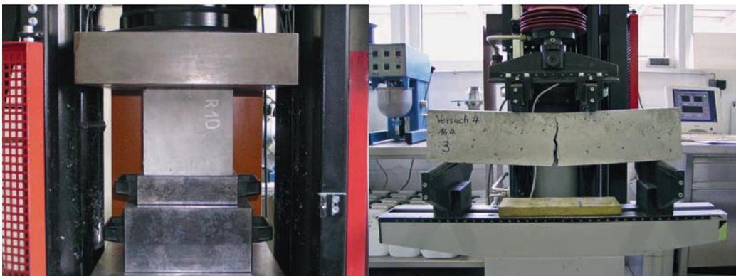
Fig. 1.36: Examples of compressive strength and tensile bending strength testing
