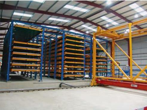
Fig. 5.40: Heated curing chamber with automatic storage and retrieval unit
