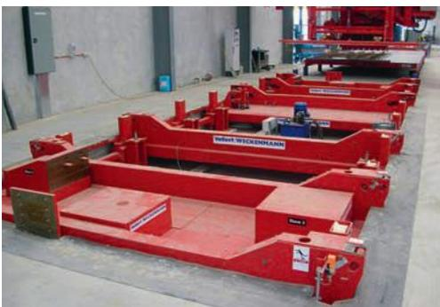
Fig. 5.12: Shaking table in a pallet circulation system
