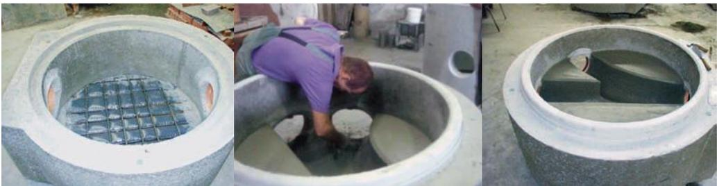
Fig. 4.29: Manual production of the channel
