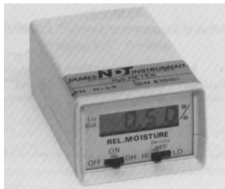
FIGURE 10.12 Meter designed to measure moisture content of solids based on capacitance. (Courtesy of NDT James Instruments Inc.)
