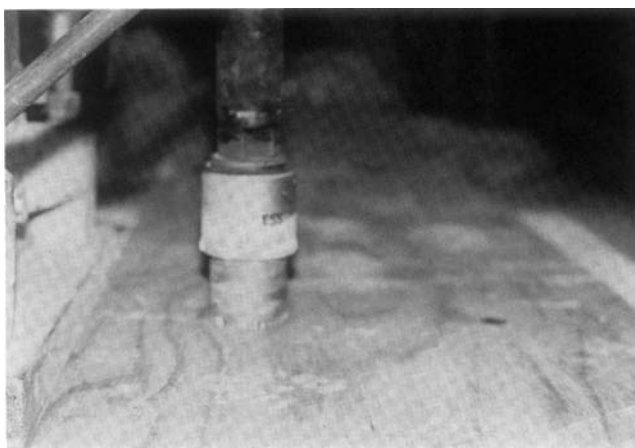
FIGURE 4.2 Core drill bit for drilling a core for BO testing of existing concrete element.
