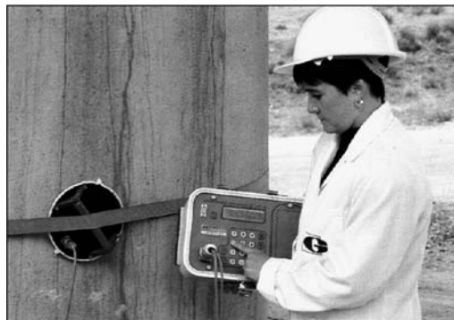
FIGURE 11.17 Example of linear polarization apparatus. (Courtesy of James Instruments, Inc.)
