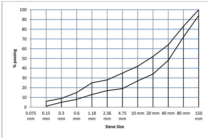
**Fig. 6.5** Recommended combined grading curve for MSA 150 mm
