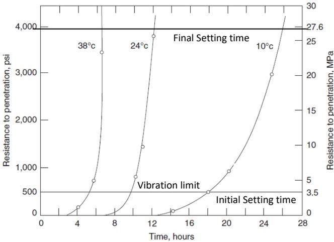
**Fig. 8.3** Effect of temperature on setting time of concrete
