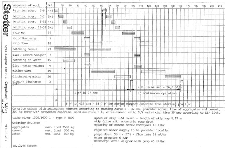
Fig. 9.3 Typical cycle time for Schwing Stetter plant of 60 cu.m./ hour capacity
