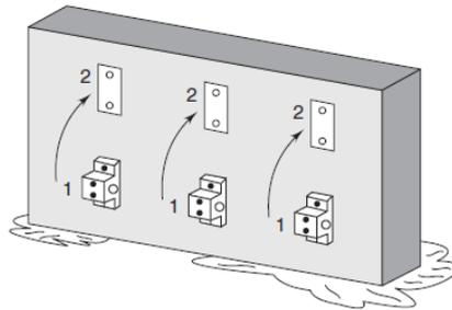
**Fig. 10.19** Sequence of external vibrator compaction
