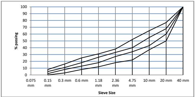
**Fig. 6.3** Recommended combined grading curve for MSA 40 mm
