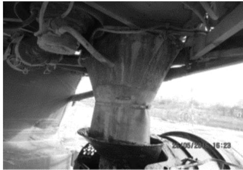
**Fig. 9.8** Enlarged entry hopper of TM
