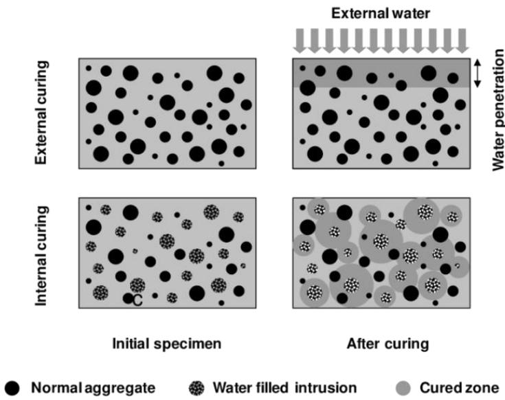
**Fig. 11.15** Concept of Self Curing Concrete with SAP or LWA
