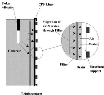
Fig. 12.14 Mechanism of CPF
