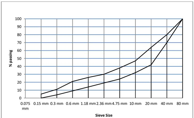
**Fig. 6.4** Recommended combined grading curve for MSA 80 mm
