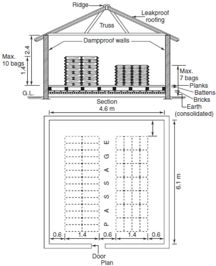
**Fig. 2.3** Typical arrangement of cement godown
