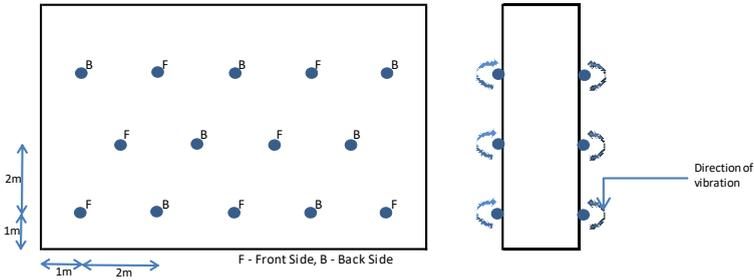
**Fig. 10.17** Placement of external vibrators for wall thickness less than 150 mm
