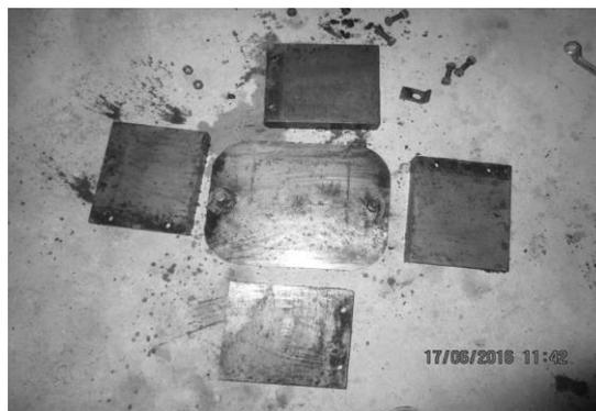
**Fig. 12.15** Lubricant properly applied on all inner surfaces on de-assembling the mould
