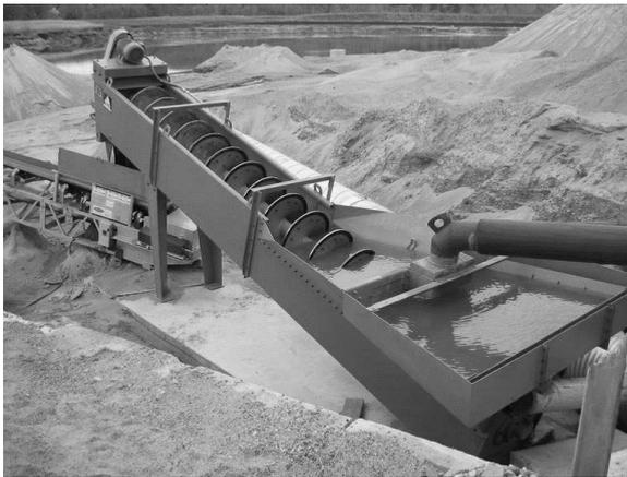
**Fig. 6.10** Typical screw classifier for washing sand
