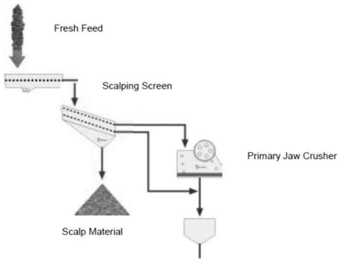
**Fig. 6.8** Scalping screen integrated in crushing plant
