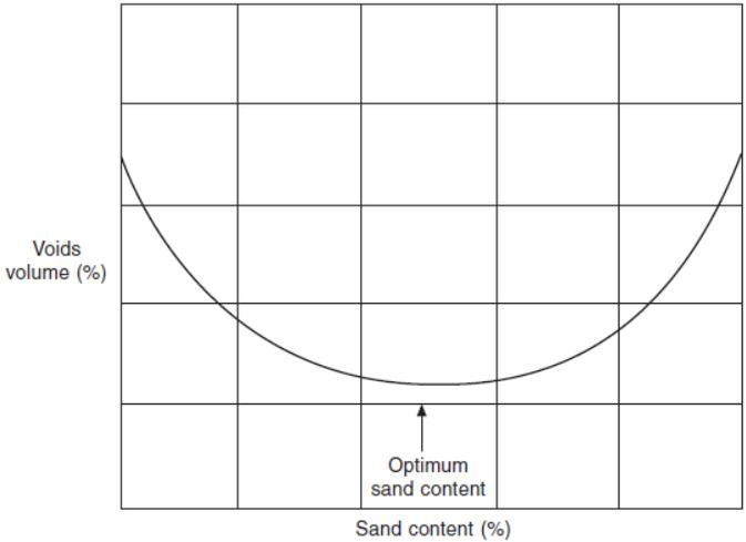
**Fig. 10.2** Relationship between voids content and sand content for determining optimum aggregate grading
