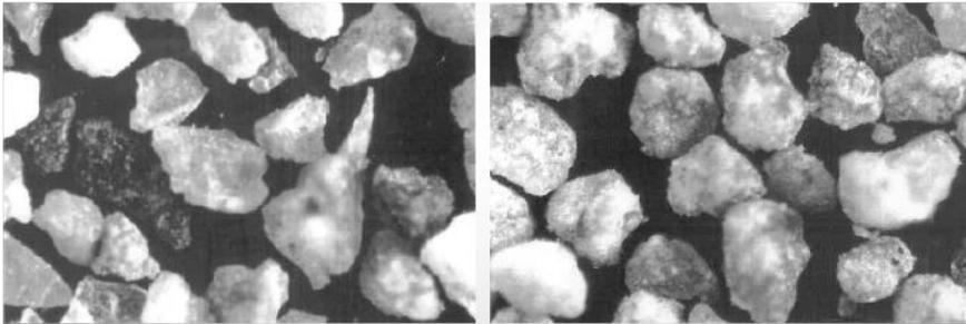
**Fig. 6.9** Comparison of 2.5 mm – 1.5 mm grains before and after VSI crusher
