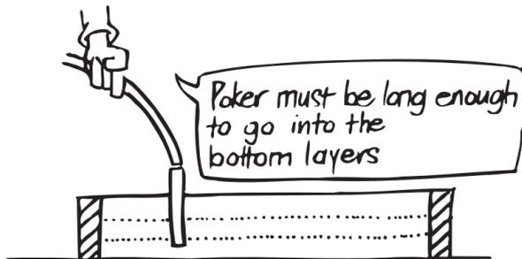
**Fig. 10.10** Vibrator must penetrate about 100 mm into previous layer during compaction
