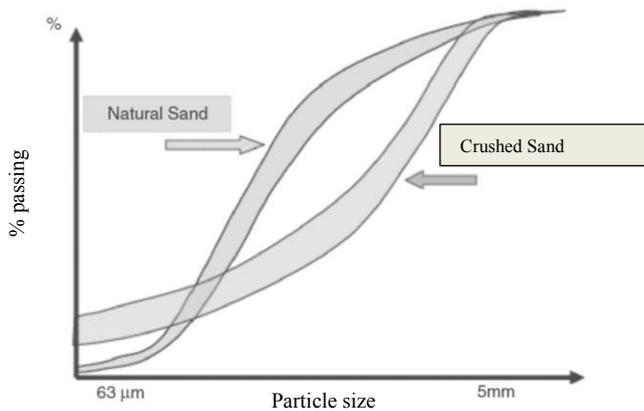
**Fig. 6.7** Typical grading curves for natural and crushed sand
