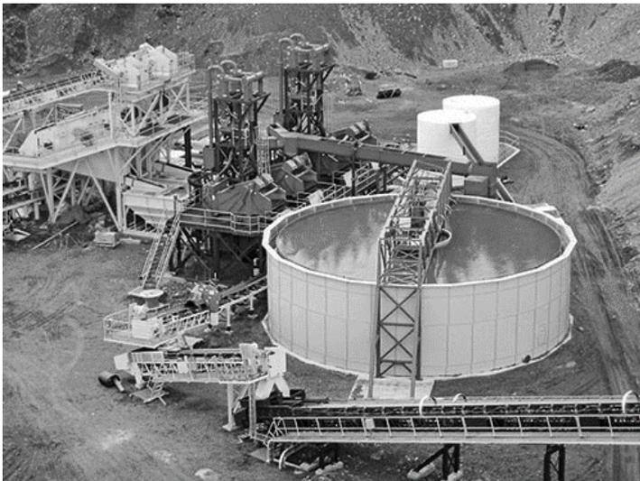
**Fig. 6.12** Typical layout of aggregate washing system integrated into crushing plant
