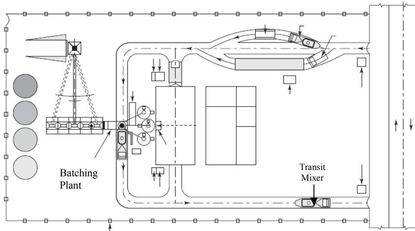
**Fig. 9.6** Proper layout of batching plant for easy movement of transit mixer
