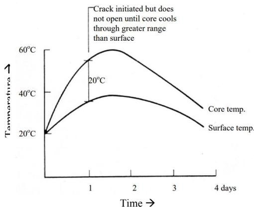
**Fig. 8.8** Internal thermal cracking
