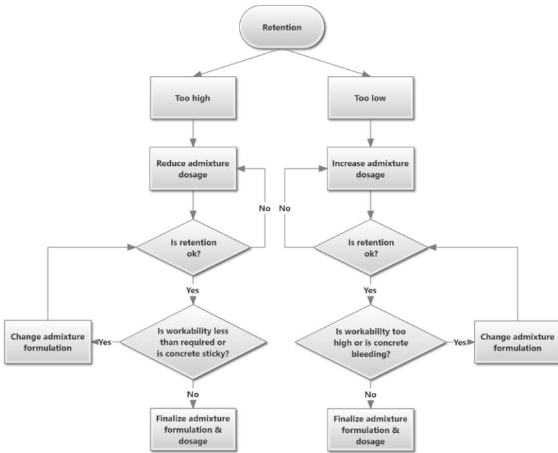
Fig. 7.4 Flow chart to achieve desired retention
