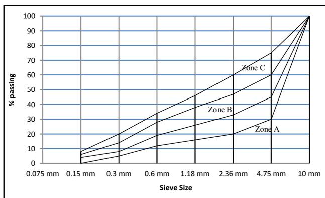
**Fig. 6.1** Recommended combined grading curve for MSA 10 mm
