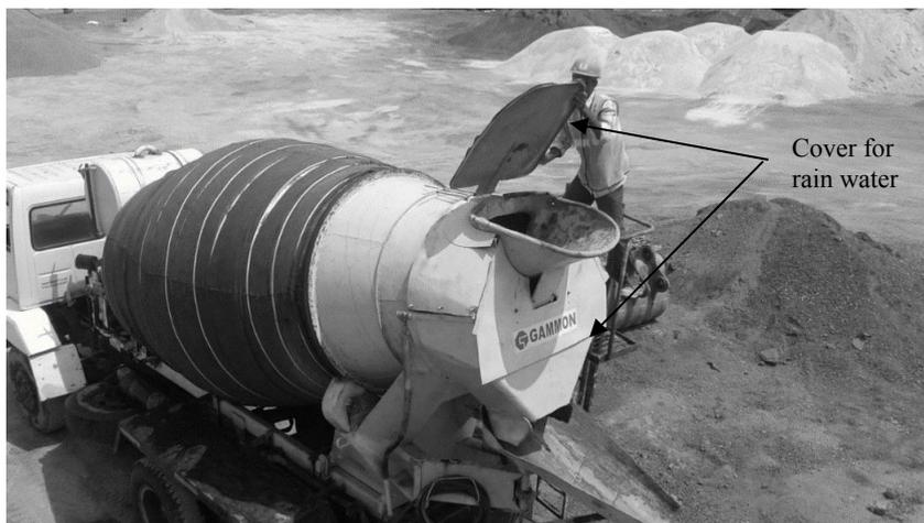
**Fig. 3.5** Arrangement for covering Transit Mixer Hopper (top and sides) for protection against rain water
