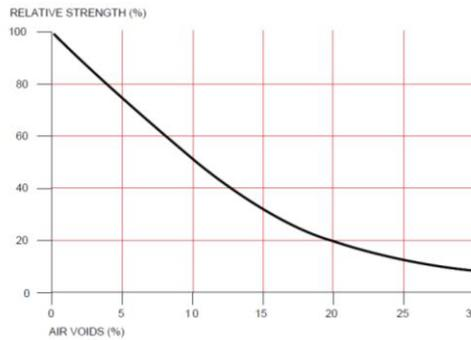
**Fig. 4.1** Typical relationship between loss of strength & air voids in concrete
