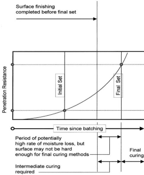
**Fig. 11.5** Surface finishing has been completed before the concrete surface has reached final set
