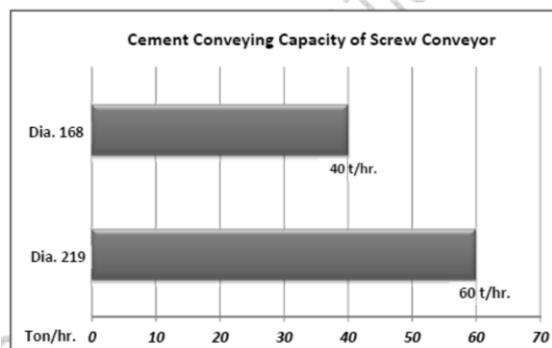
Fig. 9.4 Cement conveying capacity of screw conveyor
