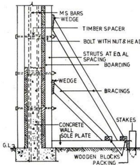
**Fig. 12.10** Formwork for walls
