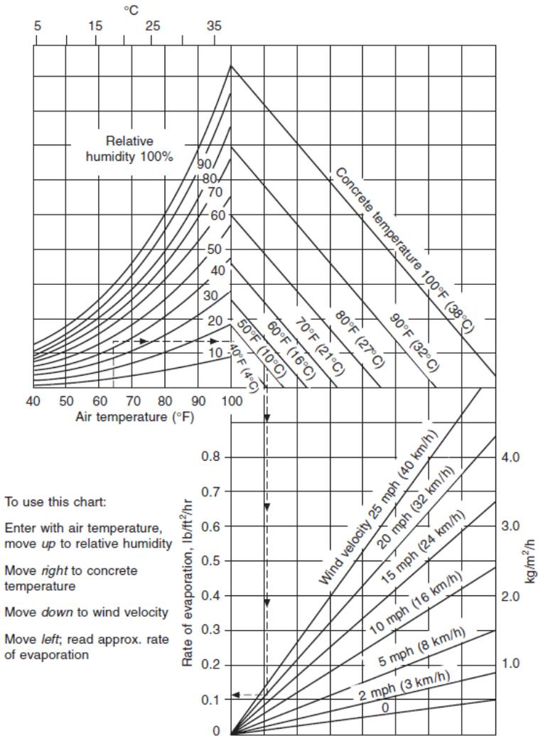
**Fig. 11.1** Calculation of rate of water evaporation from concrete surface
