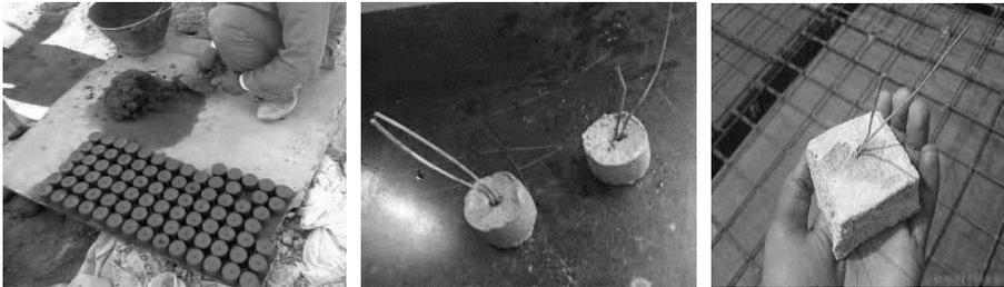
**Fig. 12.6** Cover blocks made at project site with use of vibratory table
