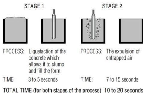
**Fig. 10.7** Stages of compaction of concrete
