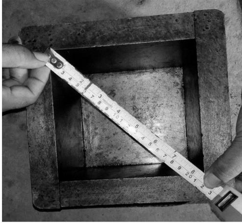
**Fig. 12.17** Measuring the diagonal of the cube mould
