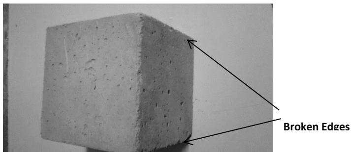
**Fig. 12.16** Concrete cube with broken edges and lot of air voids
