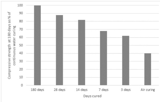
**Fig. 11.2** Effect of curing period on strength gain of concrete
