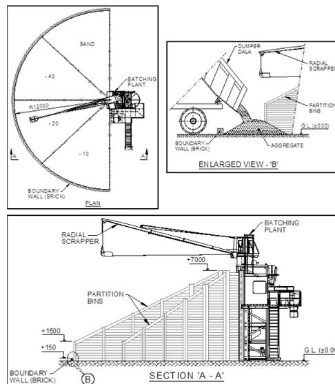
**Fig. 9.1** Protection on aggregate in star bins system
