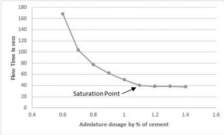
**Fig. 7.2** Determining saturation point of admixture
