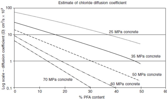
**Fig. 3.3** Rate of chloride ion diffusion value of fly ash concrete
