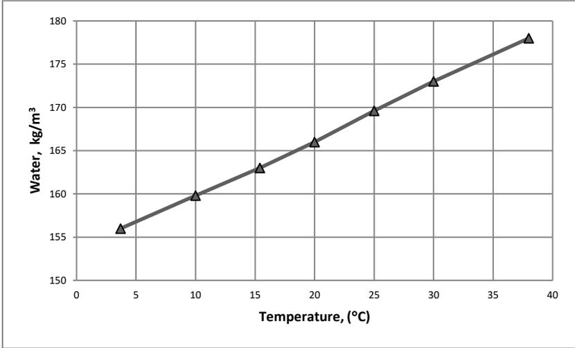
**Fig. 8.1** Effect of temperature on workability
