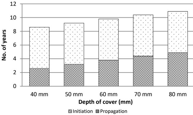
**Fig. 12.2** Effect of depth of cover on corrosion of reinforcement for concrete with w/b of 0.40
