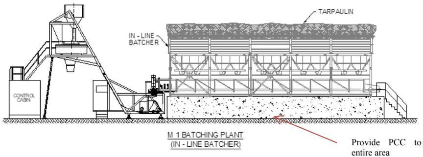
**Fig. 9.2** Protection on aggregate in inline bins system
