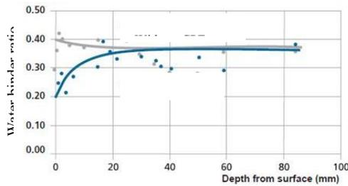
Fig. 12.12 Reduction in w/b ratio in cover concrete with use of CPF
