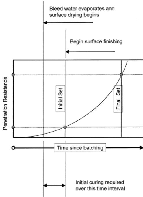
**Fig. 11.4** Bleed water disappears and surface drying commences at some time before beginning finishing. Initial curing is required to minimize moisture loss before and during finishing operations
