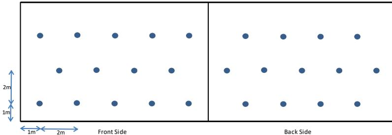
**Fig. 10.18** Placement of external vibrators for wall thickness more than 150 mm
