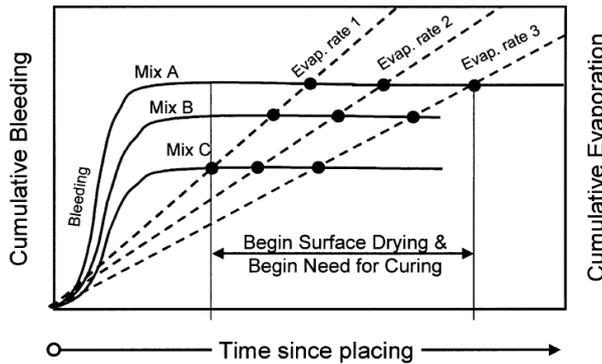
**Fig. 11.3** Schematic illustration showing combined influence of bleeding characteristics and evaporation in determining the time at which the surface of concrete begins to dry
