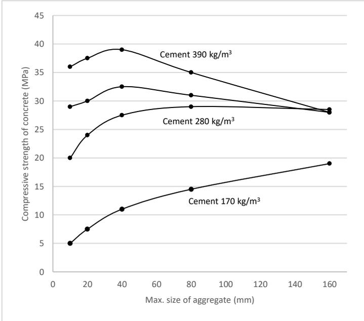
**Fig. 6.6** Relationship between MSA and compressive strength of concrete designed with varying cement contents
