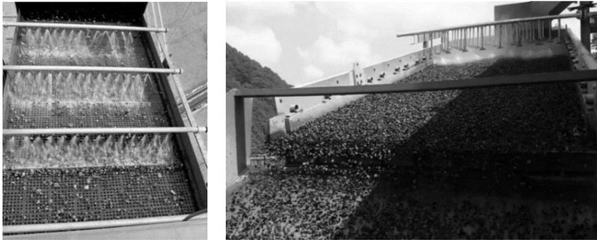
**Fig. 6.11** Aggregate material being washed as it passes over a screen deck
