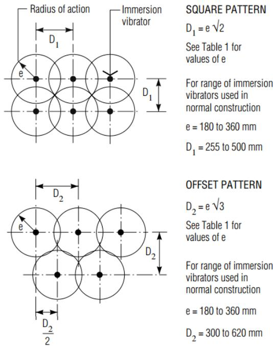
**Fig. 10.9** Alternative patterns for use of immersion vibrators
