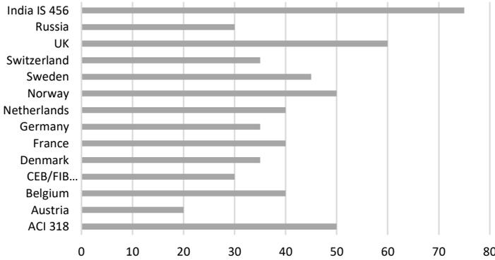
**Fig. 12.1** Minimum cover in mm for worst exposure condition in various codes / standards
