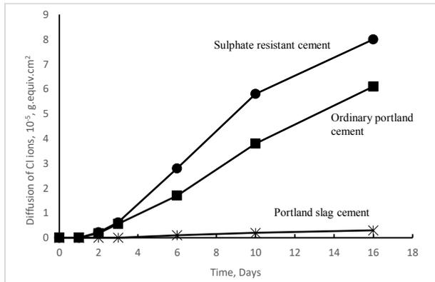
Fig. 2.1 Effect of type of cement on the rate of diffusion of chloride ions
