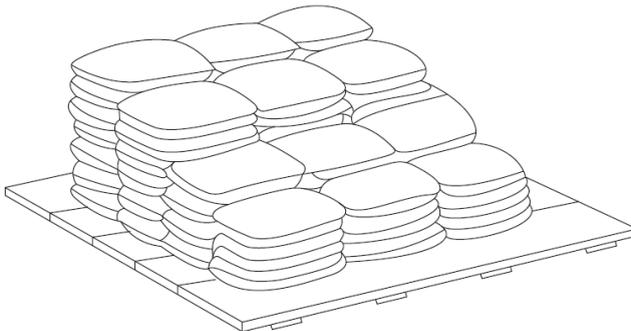
**Fig. 2.4** Stepping of tiers while removing cement bags
