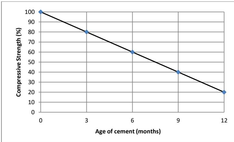
**Fig. 2.2** Approx. indication of deterioration of cement strength with age
