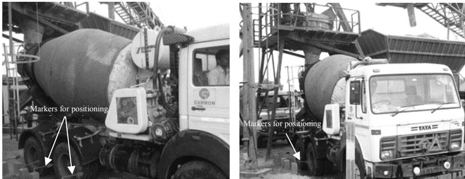
**Fig. 9.7** Providing indicators for proper positioning of TM under chute
