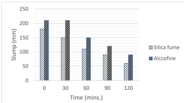
**Fig. 5.1** Comparison of UFS and SF on workability of concrete designed with same proportions
