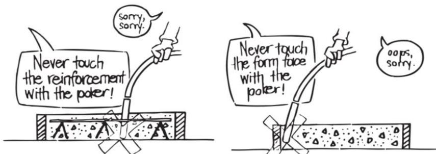
**Fig. 10.13** Do not touch reinforcement or formwork with vibrator
