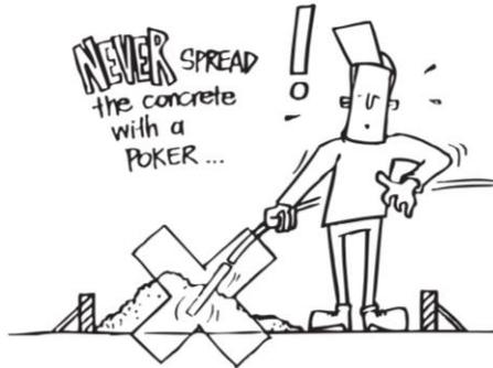
Fig. 10.14 Avoid spreading concrete with vibrator
