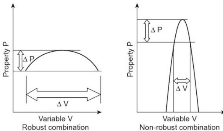
**Fig. 7.7** Robustness of concrete to variation in material properties
