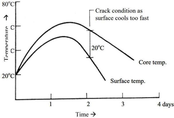
Fig. 8.5 External thermal cracking
