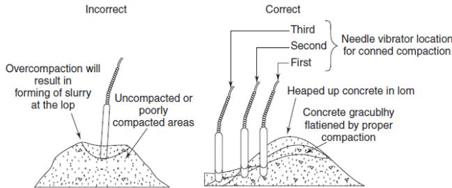
Fig. 10.15 Incorrect and correct method of compaction in a heaped concrete
