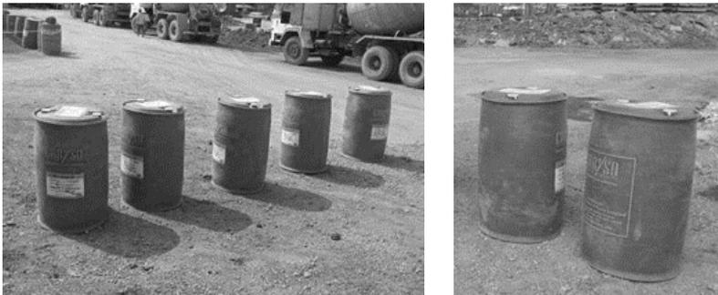
**Fig. 7.9** Bulging of sealed admixture drums kept exposed to direct sunlight
