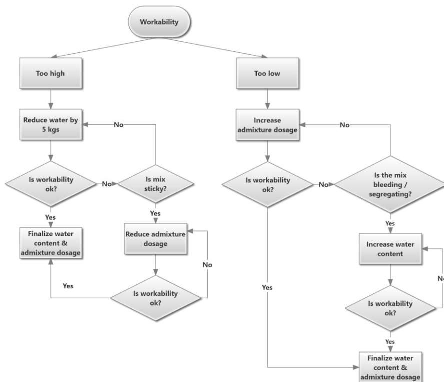
**Fig. 7.3** Flow chart for fine tuning mix to achieve desired workability
