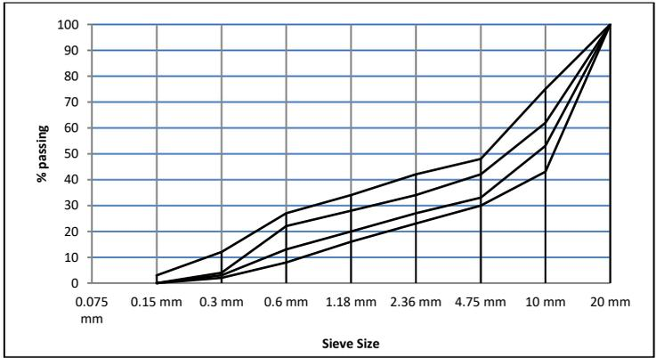
**Fig. 6.2** Recommended combined grading curve for MSA 20 mm
