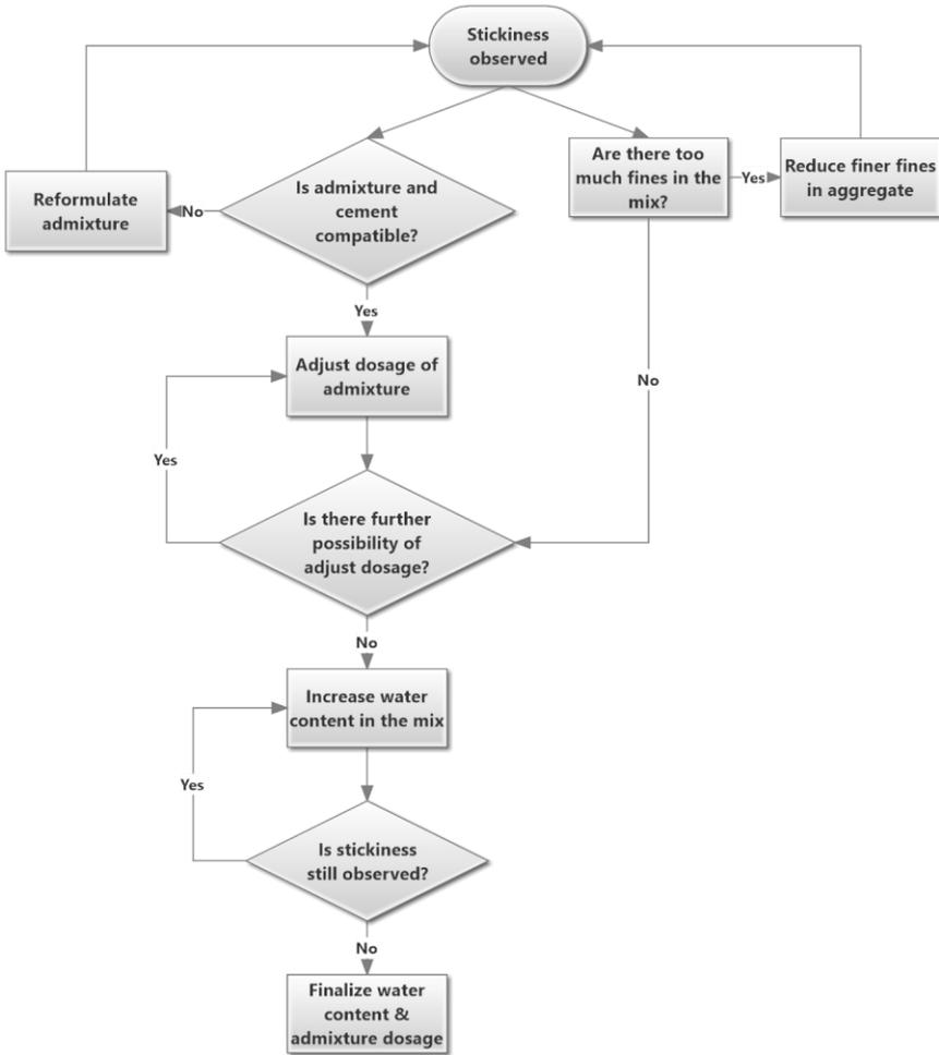
Fig. 7.6 Flow chart to control stickiness in concrete
