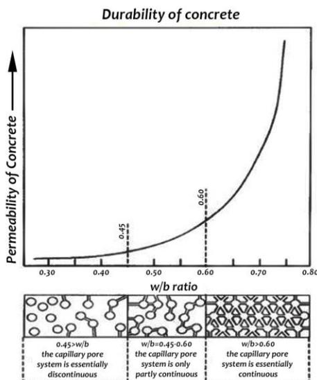
Fig. 3.2 Effect of w/b ratio on permeability of concrete
