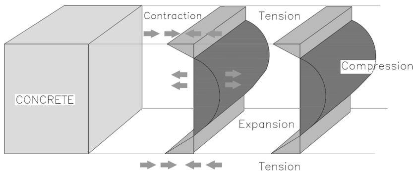
**Fig. 8.7** Development of tensile stresses due to temperature differential in thick concrete section
