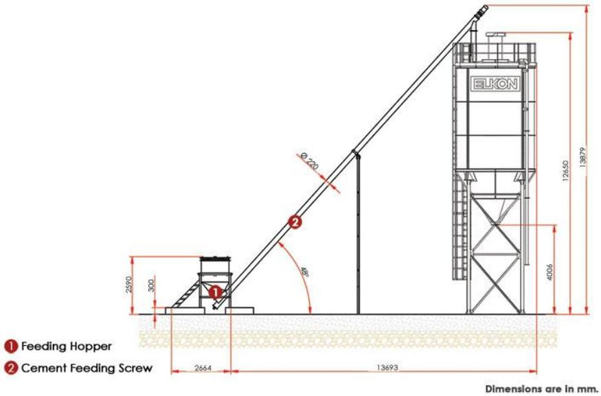
**Fig. 2.6** Typical bag cement feeding system
