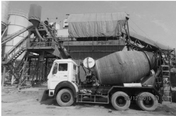
**Fig. 3.7** Providing cover over batching plant aggregate inline bins
