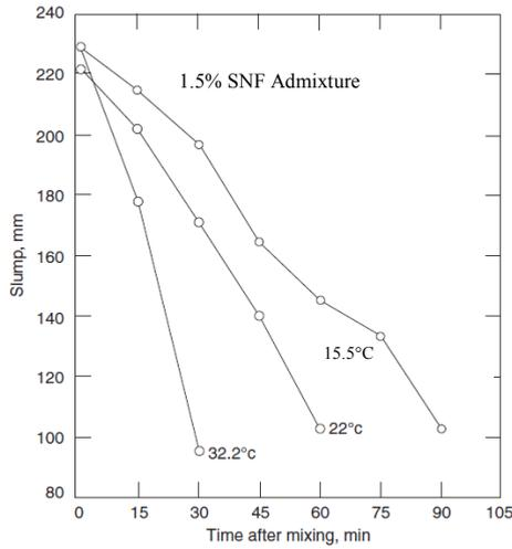
**Fig. 8.2** Effect of temperature on slump loss
