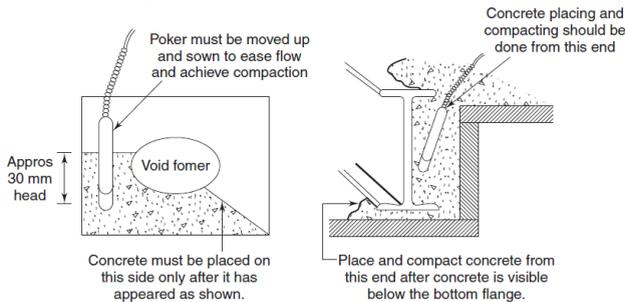
Fig. 10.16 Correct method of placing concrete below a circular or structural Void former
