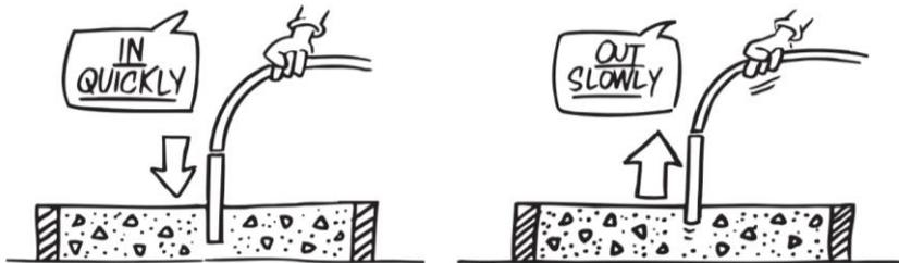
**Fig. 10.11** Method of inserting & withdrawal of vibrator in concrete
