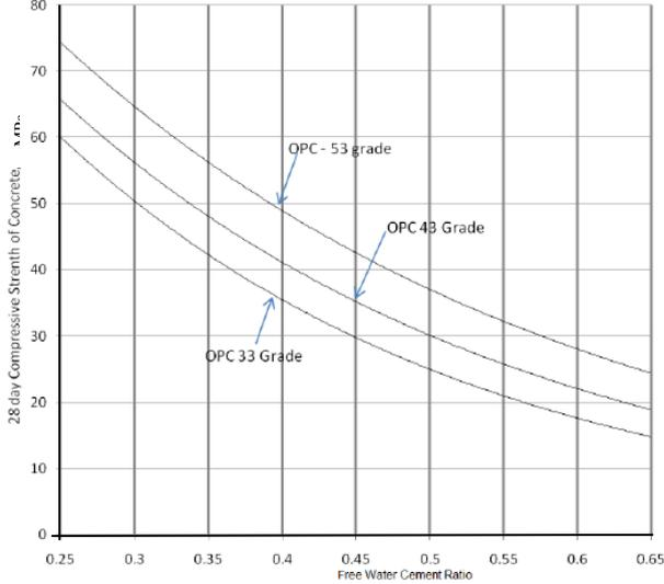
**Fig. 3.1** Relationship between water cement ratio and 28 days’ concrete compressive strength for different strengths of cement (IS 10262: 2017 - Draft)
