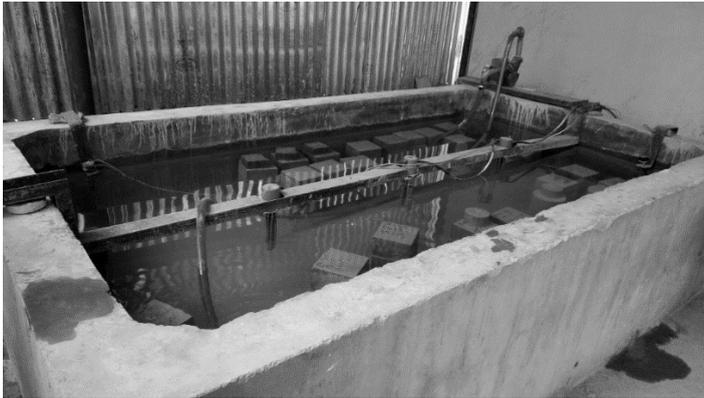
**Fig. 8.4** Controlling temperature of water in curing tank by immersion rods connected to thermostat
