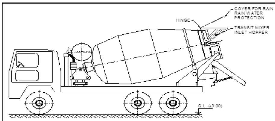
**Fig. 3.4** Arrangement for covering Transit Mixer Hopper (top and sides) for protection against rain water
