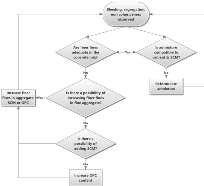
Fig. 7.5 Flow chart to control bleeding, segregation and non-cohesiveness
