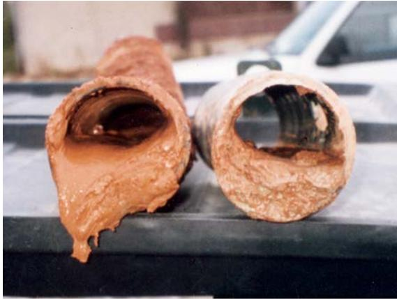
**CLOGGED FOOTING DRAINS CAN'T DO THE JOB.** Water draining into the pipe carries silt that eventually fills the pipe. To avoid replacing a clogged footing drain, the author surrounds the pipe with a layered filter that stops sediment.
