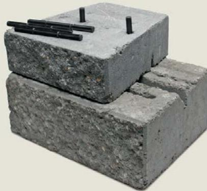
**VERSA-LOK® MOSAIC.** A top-down pinning system lets you push a pin through a hole in one course and into a groove in the course below ([www.versa-lok.com](http://www.versa-lok.com); 651-770-3166).
