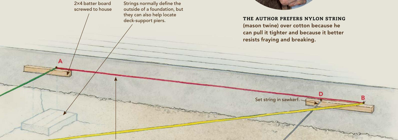
**Step 3:** Define the long leg of the triangle. Often a door, a window, or a wall dictates where a project begins. If not, pick a spot and call it point A. Measure 24 ft. to point B. Screw 2x4 batter boards to the house at points A and B.
