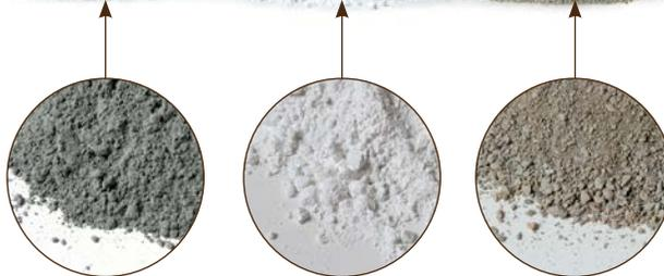
Portland cement + Hydrated lime + Sand = Mortar
