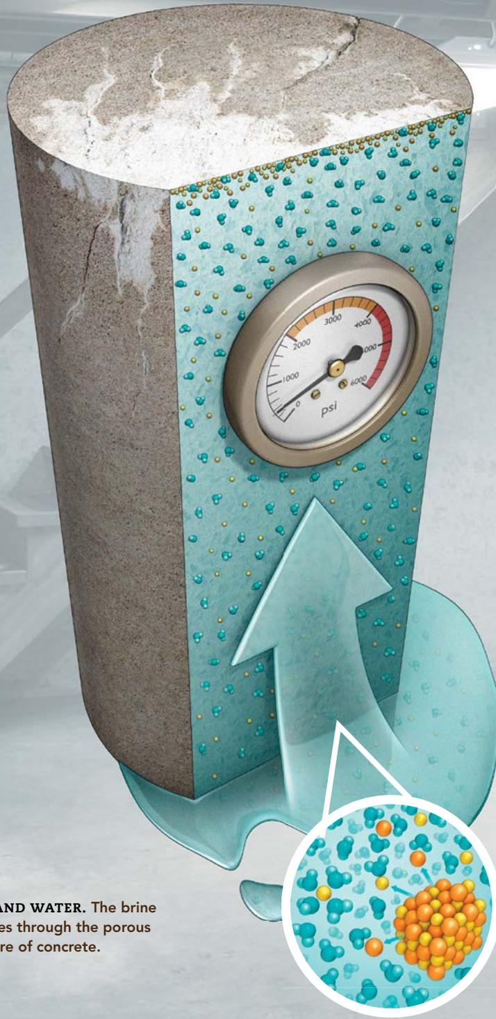
**SALT AND WATER.** The brine migrates through the porous structure of concrete.
