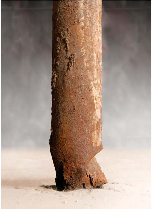
**SAGGING FLOORS** may be due to a failing column or the lack of a proper footing. In either case, you must temporarily support the beam and remove the old column.
