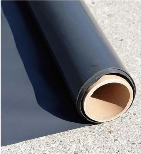
**A TOUGH VAPOR BARRIER KEEPS THE BASEMENT SLAB DRY.** Made of 2-ply high-density polyethylene, the vapor barrier can be installed under or over the gravel base and keeps moisture from wicking up through the slab.
