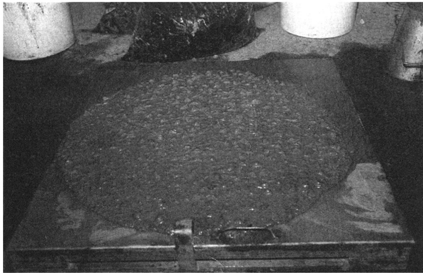
Figure 2.6 The flow table consists of a wooden board, faced with sheet metal, connected to a baseboard. (a) Diagram of the apparatus. (b) Flow table test. (Photo courtesy of Tilcon Ltd).
