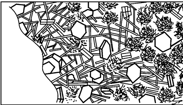
Figure 7.9 Model of transition zone of the ordinary concrete.
