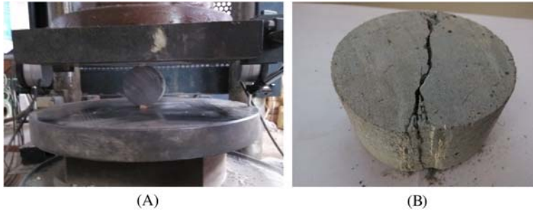
Figure 2.10 Split tensile tests. (A) Test setup. (B) Failure specimen.
