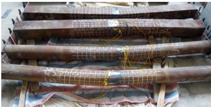
Figure 5.9 Overall deformed shapes after residual capacity test.
