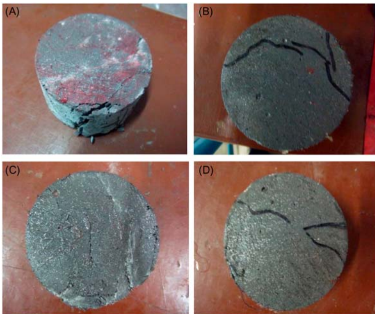
Figure 2.14 Failure patterns of specimens with different nanomaterials. (A) 3% NC. (B) 3% NS. (C) 3% NA. (D) 3% NT.
