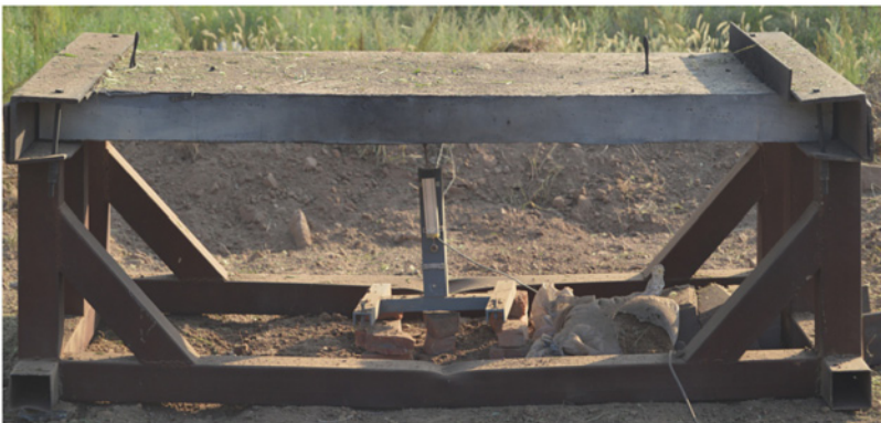
Figure 3.84 UHMWPE-1 fiber-reinforced concrete slab after 6 kg TNT from 1.5 m standoff.
