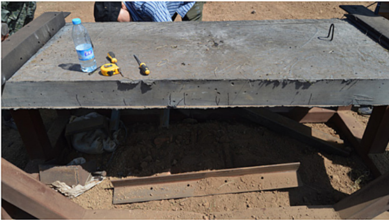
Figure 3.88 Hybrid-1 fiber-reinforced concrete slab after 6 kg TNT detonation from 1.5 m standoff distance.
