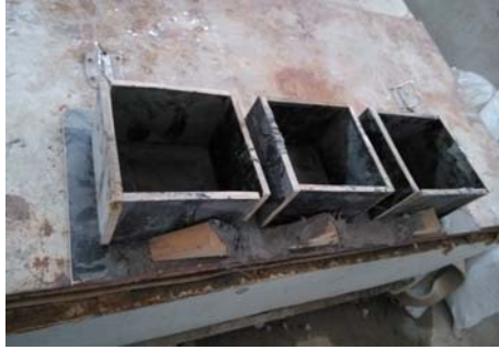
Figure 2.25 Concrete wooden molds.
