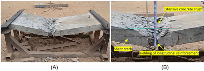
Figure 3.92 Plain concrete slab after 8 kg TNT detonation from 1.5 m standoff distance: (A) slab failure and (B) residual deflection.
