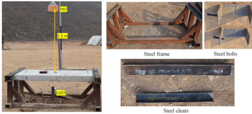
Figure 3.82 Close-in detonation setup and clamping system.
