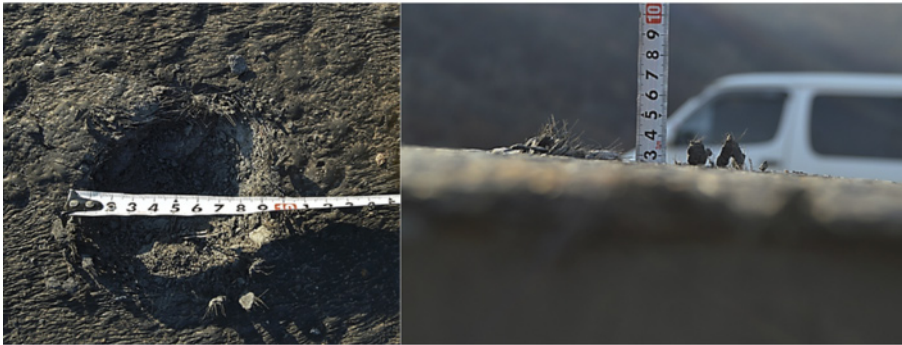
Top surface concrete crater diameter and depth
