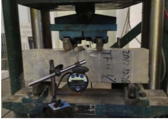
Figure 2.3 Setup of the flexural tests.
