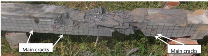
H8A specimen with 1000 kN axial load under 24 kg charge weight loading
