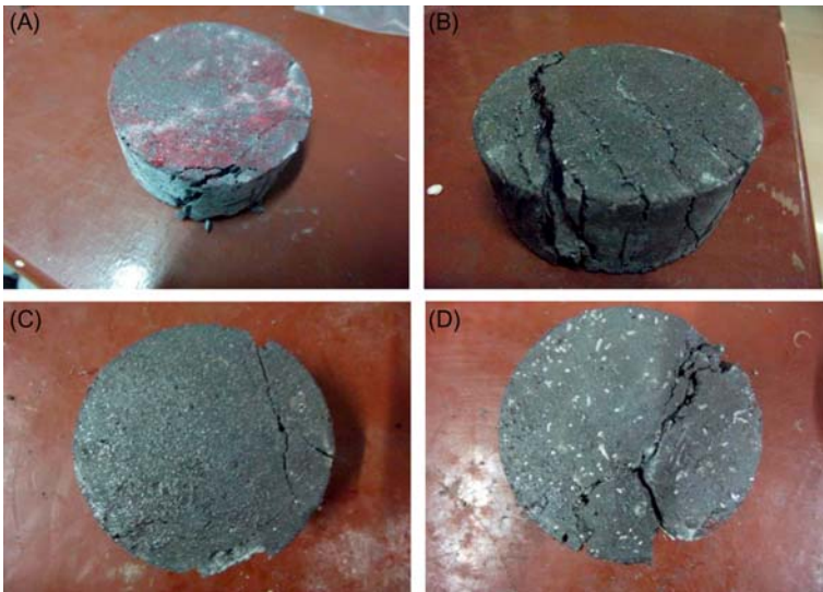
Figure 2.31 : Failure patterns of different types of fiber. (A) 2.5% MF15, (B) 2.5% MF06, (C) 2.5% TF03, and (D) 2.5% TF05.
