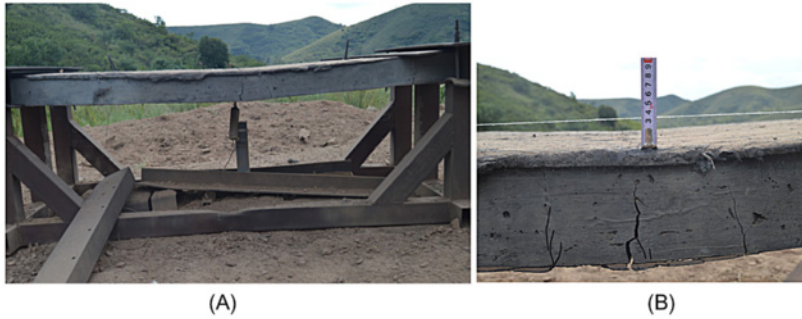
Figure 3.89 Hybrid-2 fiber-reinforced concrete slab after 12 kg TNT detonation from 1.5 m standoff distance: (A) slab flexural crack and (B) residual deflection.
