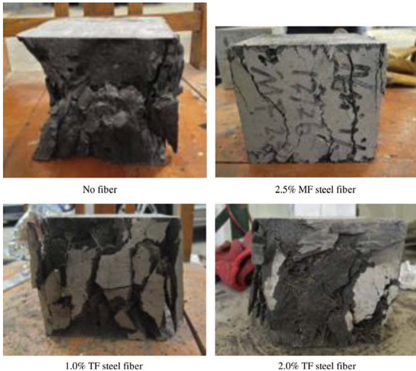
Figure 2.4 Failure of specimens from the compression tests.
