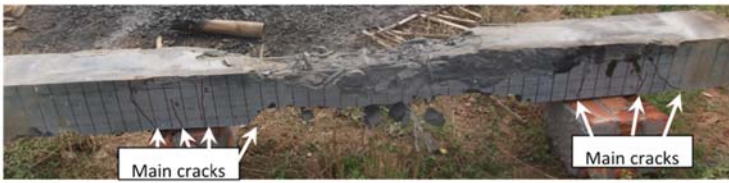
H7A specimen with no axial load axial load under 24 kg charge weight loading
