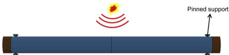
Figure 5.86 Model setup of circular column with pinned support.
