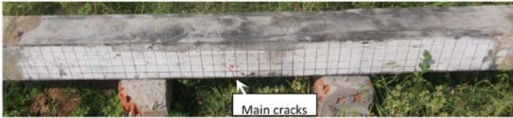
U6B specimen with 1000 kN axial load under 24 kg charge weight loading
