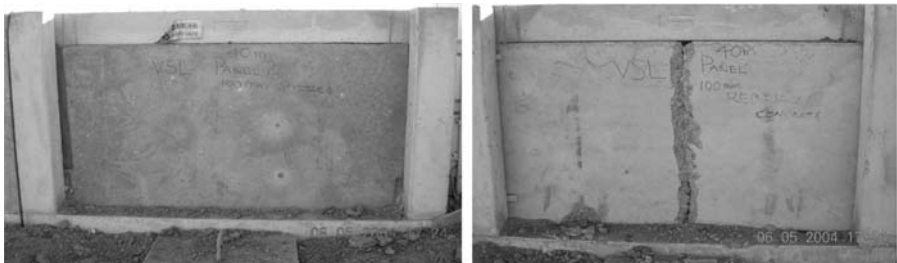
Figure 1.7 UHPC slab versus NSC slab under 5 ton Hexolite-RDX/TNT detonation at 40 m standoff distance.
