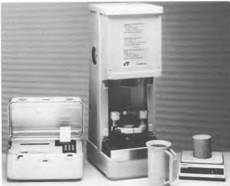
Fig. 9 Intensive Compaction Tester /8/.
