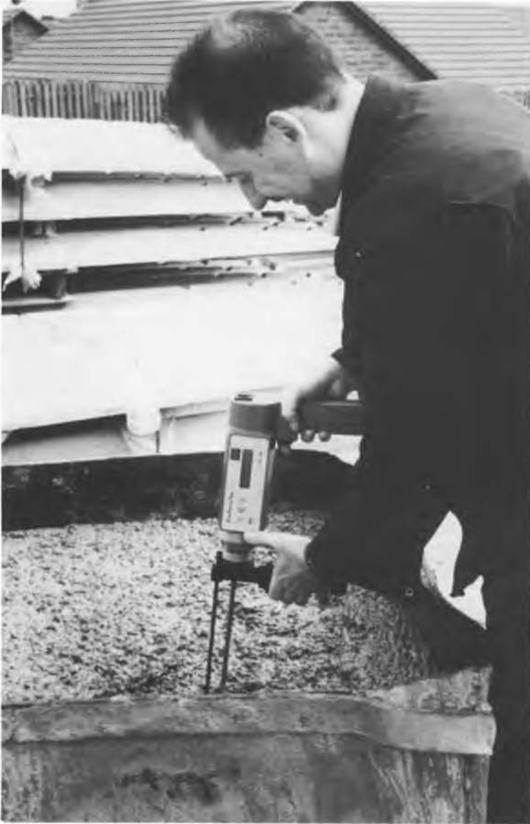
Fig. 1 . Assessment of workability of a fresh mix using the FCT 101 tester.
