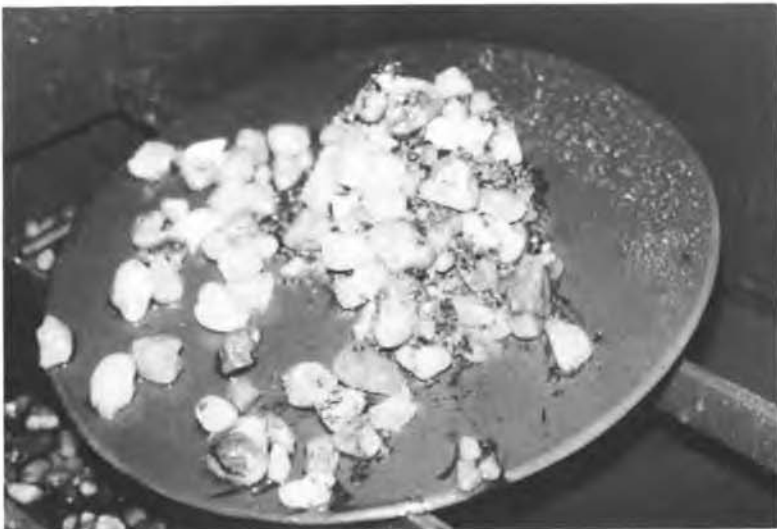
Fig. 15. Visual assessment of the concrete sample after the MC-1 washout test procedure
