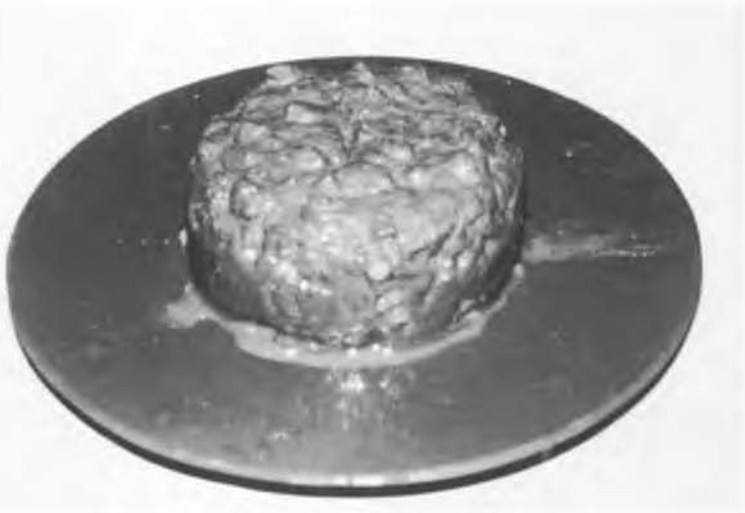
Fig. 4. Baseplate and a concrete sample before the test procedure
