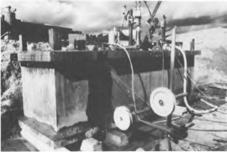
Fig. 8: Cutting the test specimen with a diamond saw
