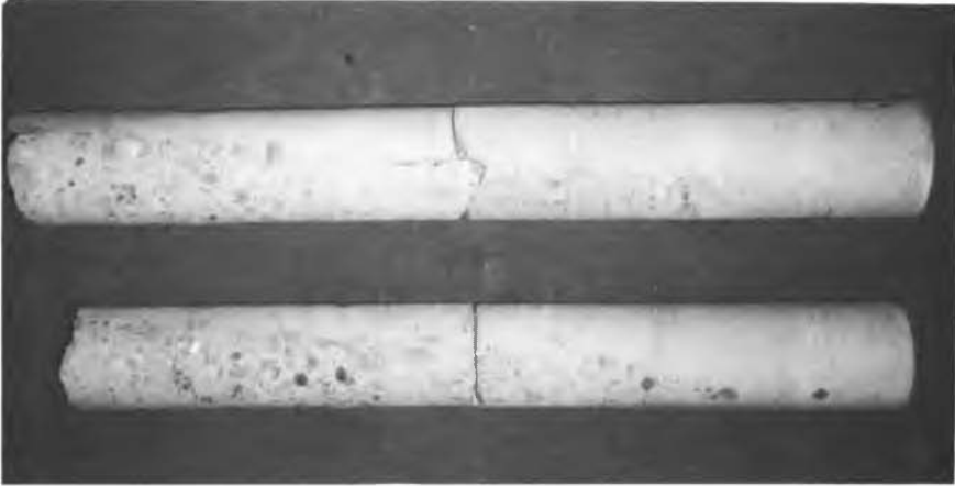
Fig. 4 Cores taken into trial repair
