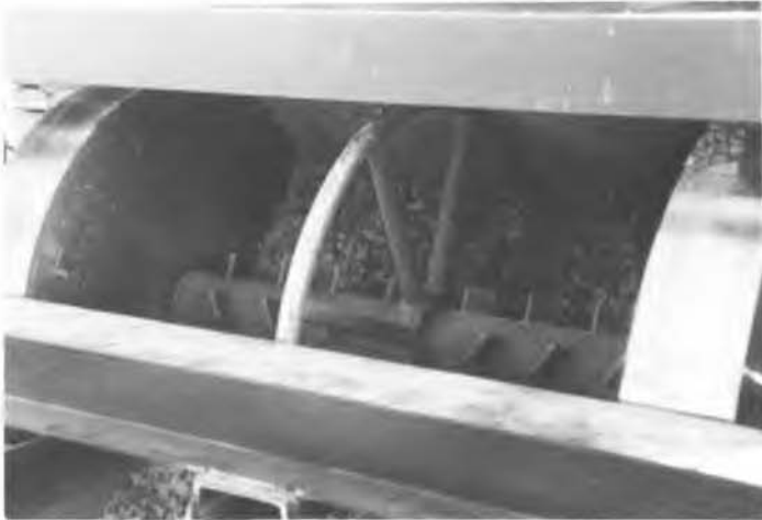
Fig. 8 Photo showing the kneading condition of core-blend in kneading mixer
