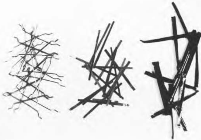
Fig. 2. Fibres used in these tests, from left to right they are :- Dramix ZL 30/.50, Fibra-flex FF30L6 and Harex SF 32.01.
