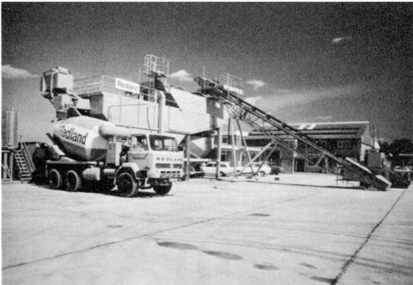
Figure 8.3 Low-level batching plant with truckmixer. Courtesy Redland Readymix Ltd
