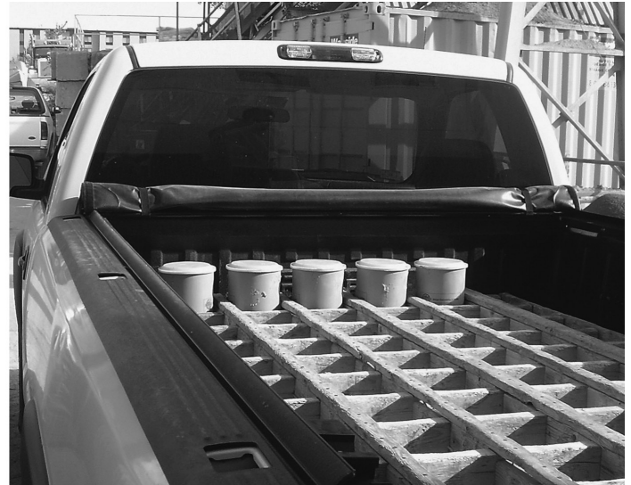
Figure 9.4 Transportation boxes (right) can significantly reduce the chances specimens will be damaged during transportation. Courtesy of CTLGroup.
