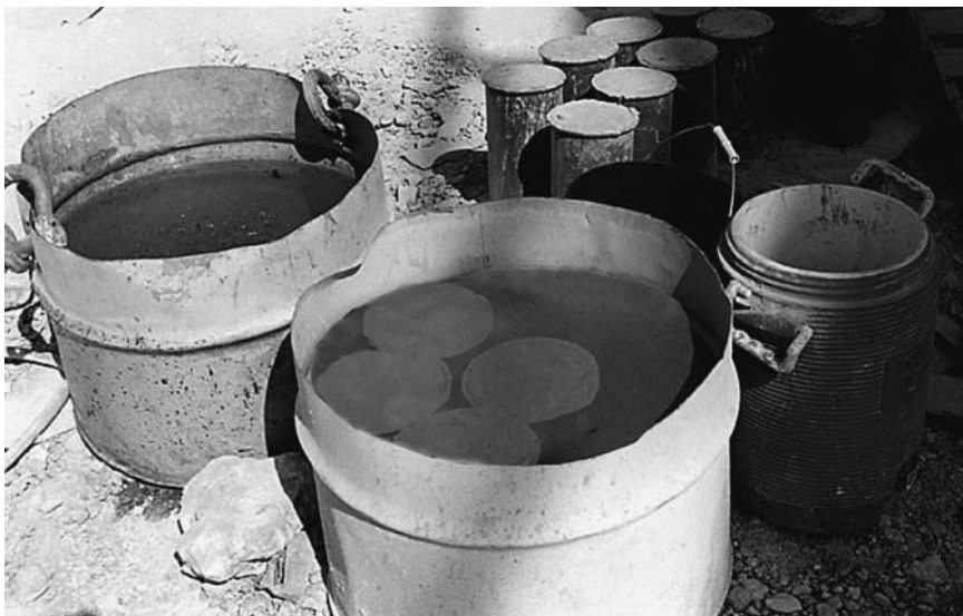
Figure 9.2 Initial jobsite curing by immersion in lime-saturated water. Courtesy of CTLGroup.
