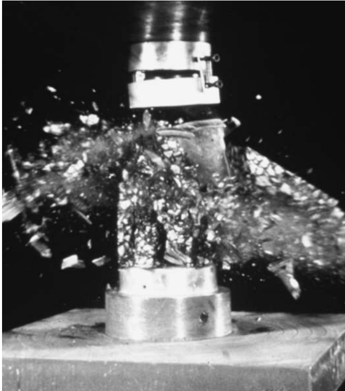
Figure 4.2 As compressive strength increases, failure takes on an increasingly explosive mode. Courtesy of CTLGroup.
