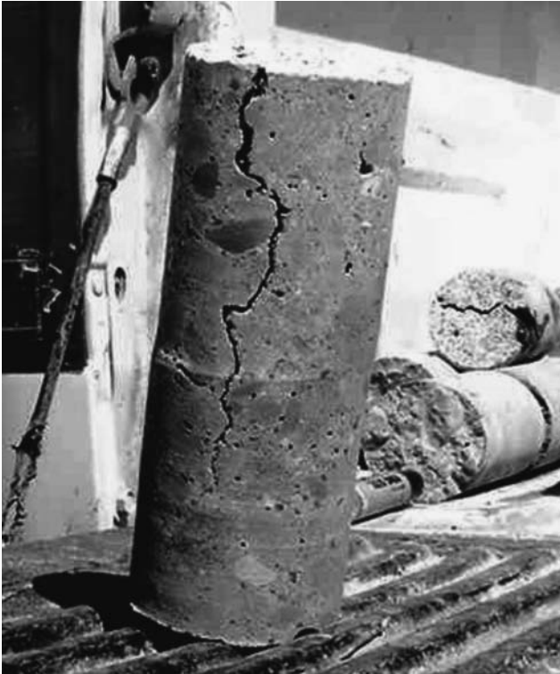
Figure 8.1 Severe plastic shrinkage cracking caused by ineffective interim curing. Cracks of this nature start out relatively shallow, but subsequently are capable of behaving as contraction joints, causing the cracks to propagate deeper into the section. Courtesy of CTL Group.
