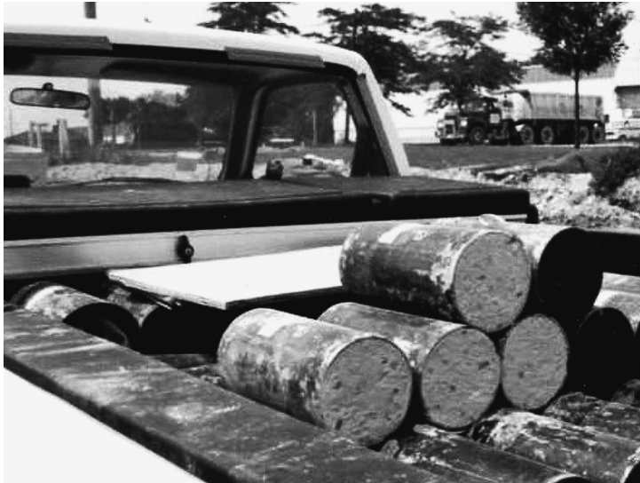
Figure 9.4 Transportation boxes (right) can significantly reduce the chances specimens will be damaged during transportation. Courtesy of CTLGroup.
