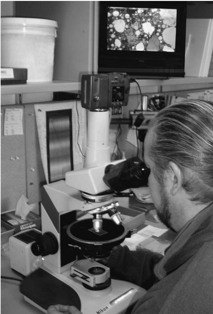
Figure 10.8 Examination of thin sections using a polarized-light microscope at magnifications up to 400 \times . Courtesy of CTLGroup.
