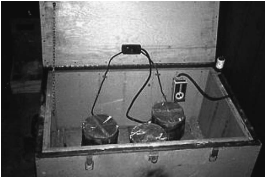
Figure 9.3 Temperature controlled jobsite-curing box. Courtesy of CTLGroup.
