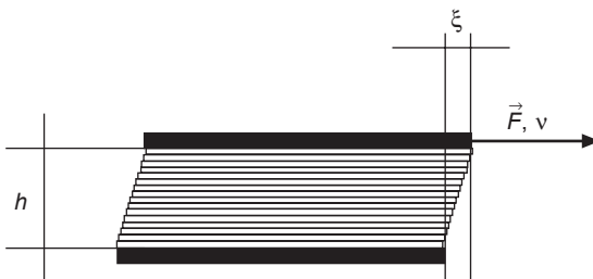
Figure 6.10 Two-Plates-Model of viscosity.
