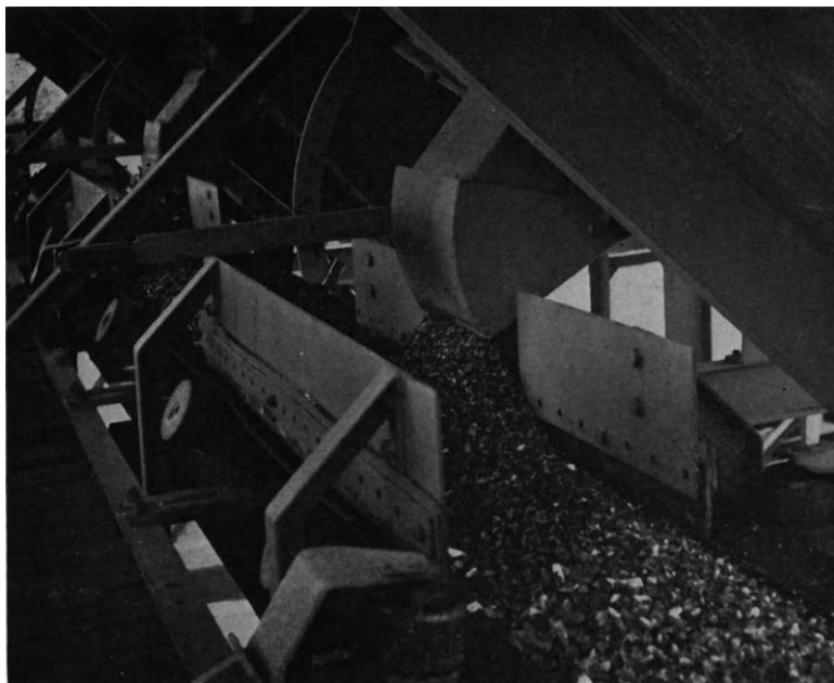
Plate 5. Regrading aggregates by re-combining single-size material.
