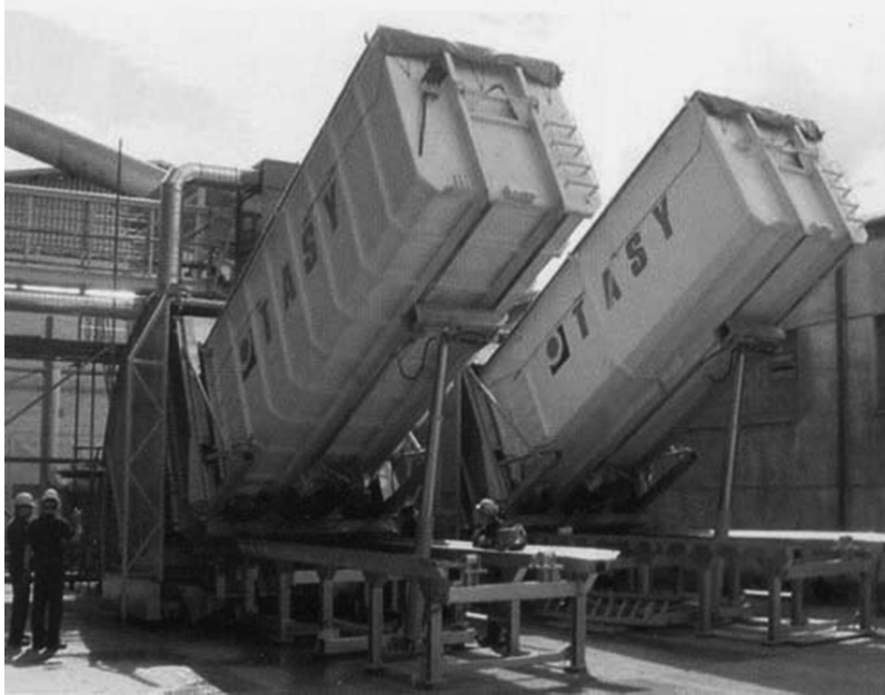
FIGURE 4.5 Docking system with walking floor container. (Reproduced from Cement International, Storing, metering and conveying solid secondary fuel—Design basis and equipment, Cement International , Vol. 5, 6/2007. 43–53. With permission from Cement International and Schenck Process GmbH.)
