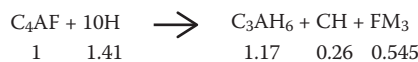
FIGURE 7.6 Cement hydration reactions at a glance. (Note: Numbers below reactions indicate volume stoichiometry.)
