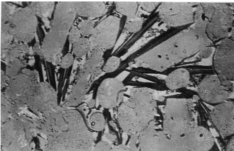
FIGURE 6.5 Clinker microstructure showing well differentiated matrix of ferrite and aluminates.
