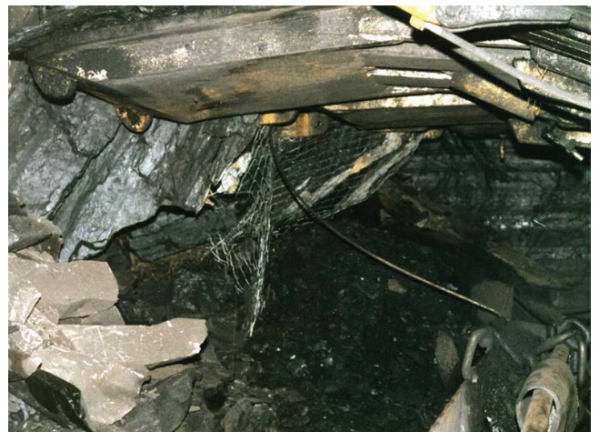
Figure 13. One of the less pleasant aspects of longwalling: a face break
