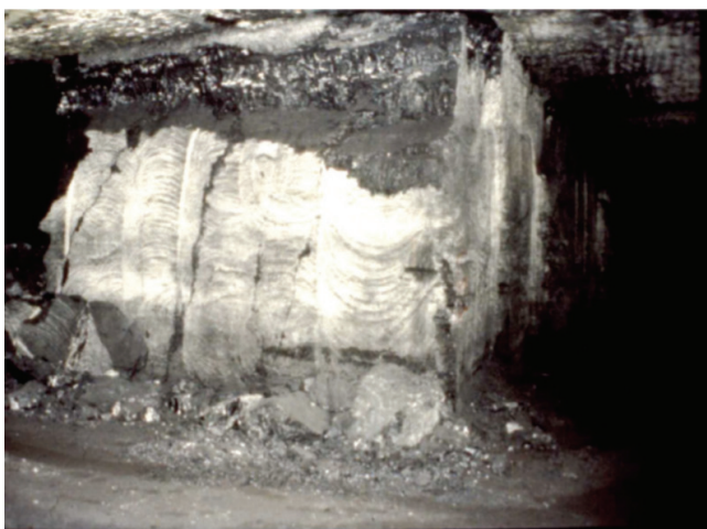
Figure 13. The fender on the left has a safety factor of around 1.0 and can be expected to be stable for a few days. The snook on the right has a very low safety factor, in the region of 0.3, and is failing. Note that in this case, the strong overhanging roof can protect the snook until the roof beam fails
