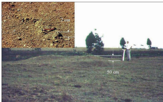
Figure 12. Examples of compression ridges. The large one would correspond to Subsidence Class D or E and the small one in the inset with Class B
