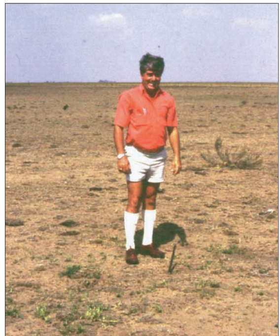
Figure 16. There are no visible signs on the surface of the sub-surface cavity on top of which the man in the pictures is standing. The 1.8 m long steel rod has all but disappeared into the hole
