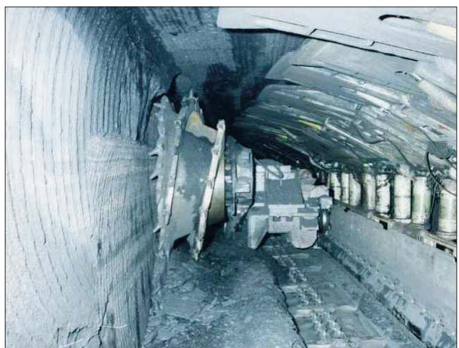
Figure 7. The contrast in the face conditions shown in these two photographs illustrate the effects of a remnant in the upper seam on longwalling on the lower seam
