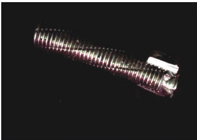
Figure 18. The remainder of the shear pin can be seen between the nut that has been cut away and the bolt. Note how the thread has been destroyed. This problem has three negative consequences: firstly, the bolt could not be properly tensioned; secondly, the excessive torque caused micro fractures in the steel body of the bolt; and thirdly, the thread/nut contact distance is greatly reduced
