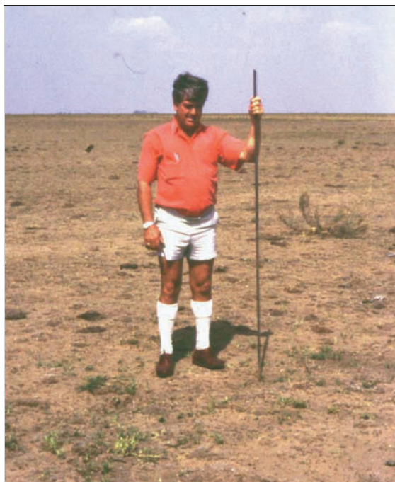
Figure 16. There are no visible signs on the surface of the sub-surface cavity on top of which the man in the pictures is standing. The 1.8 m long steel rod has all but disappeared into the hole
