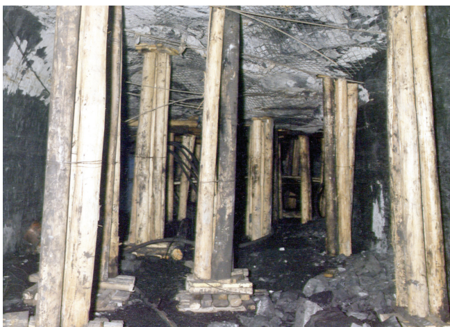
Figure 9. Timber supports in a split ahead of a longwall face where the inter panel pillars are mined
