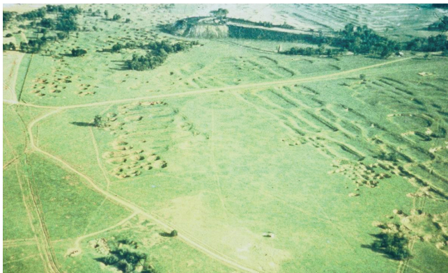
Figure 10. Intersection collapse at shallow depth
