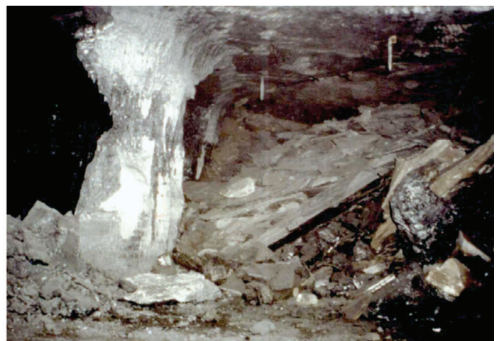
Figure 13. The fender on the left has a safety factor of around 1.0 and can be expected to be stable for a few days. The snook on the right has a very low safety factor, in the region of 0.3, and is failing. Note that in this case, the strong overhanging roof can protect the snook until the roof beam fails
