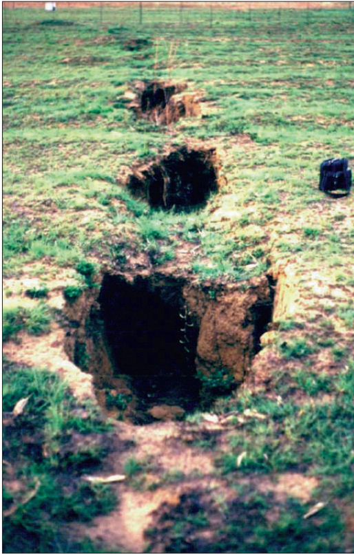
Figure 19. Mature sub-surface erosion, showing the surface holes and details of the connecting tunnel between the individual holes. In time, the holes will join to form a long trench
