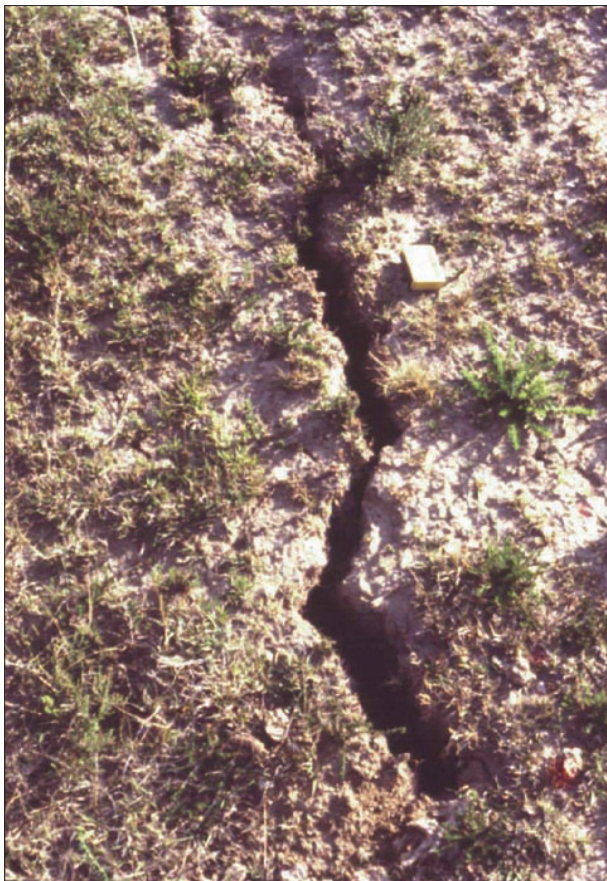
Figure 11. Illustrations of cracks caused by tensile strain. The crack on the left is about 2 cm wide and would correspond to Subsidence Class B. The 50 cm wide one on the right corresponds with Class D or E
