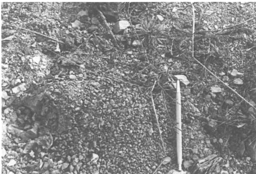
Fig. 6. Example of natural weathering of minestone /from Sośnica mine/ on the surface of embankment slope after about 4 years.
