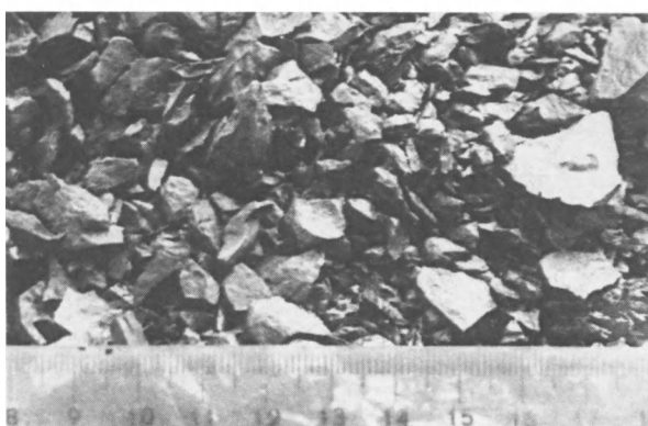
Fig. 1. Model weathering of claystones; a/ original material, b/ after 1 month, c/ after 9.5 months.
