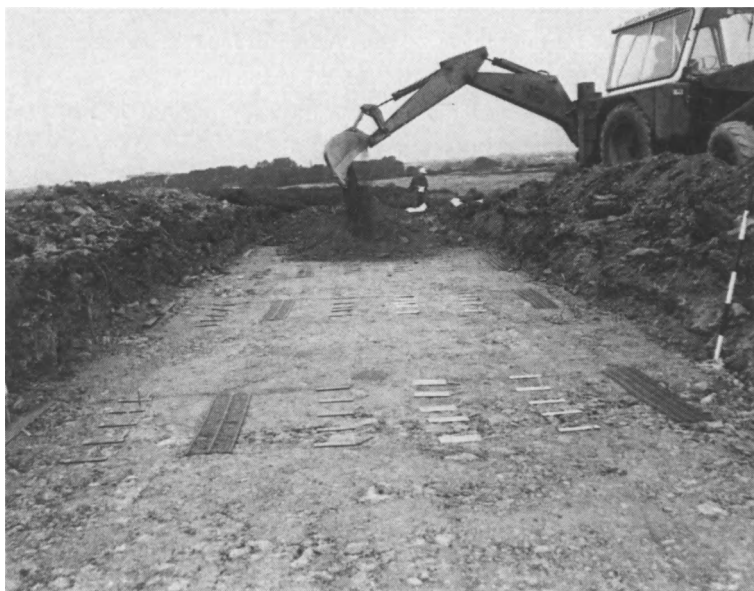
Fig. 2 Specimens being buried in the field trial
