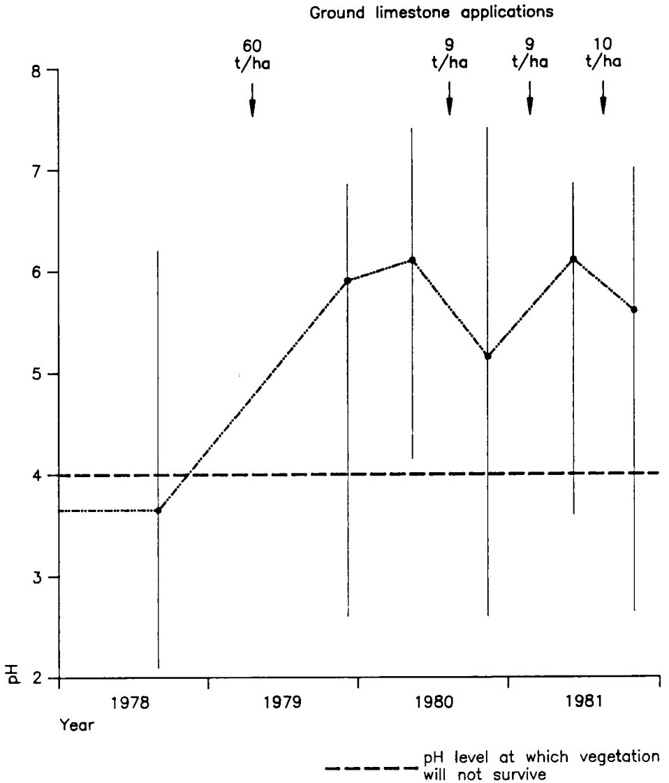
Figure 14.7: The effect of liming on mean pH and range on a pyritic colliery spoil heap. Even with repeated lime applications, the pH of parts of the site is too low to support plant growth
