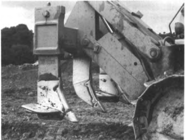
Photograph 14.5: Winged-tine ripper suitable for heavily compacted colliery spoil (source: the Forest Authority)
