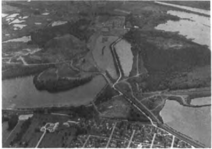
Photograph 13.5: Subsidence of the ground surface following deep mining can lead to the formation of new water bodies. The lake in the right foreground is used for fishing and other recreational activities (source: EPF)
