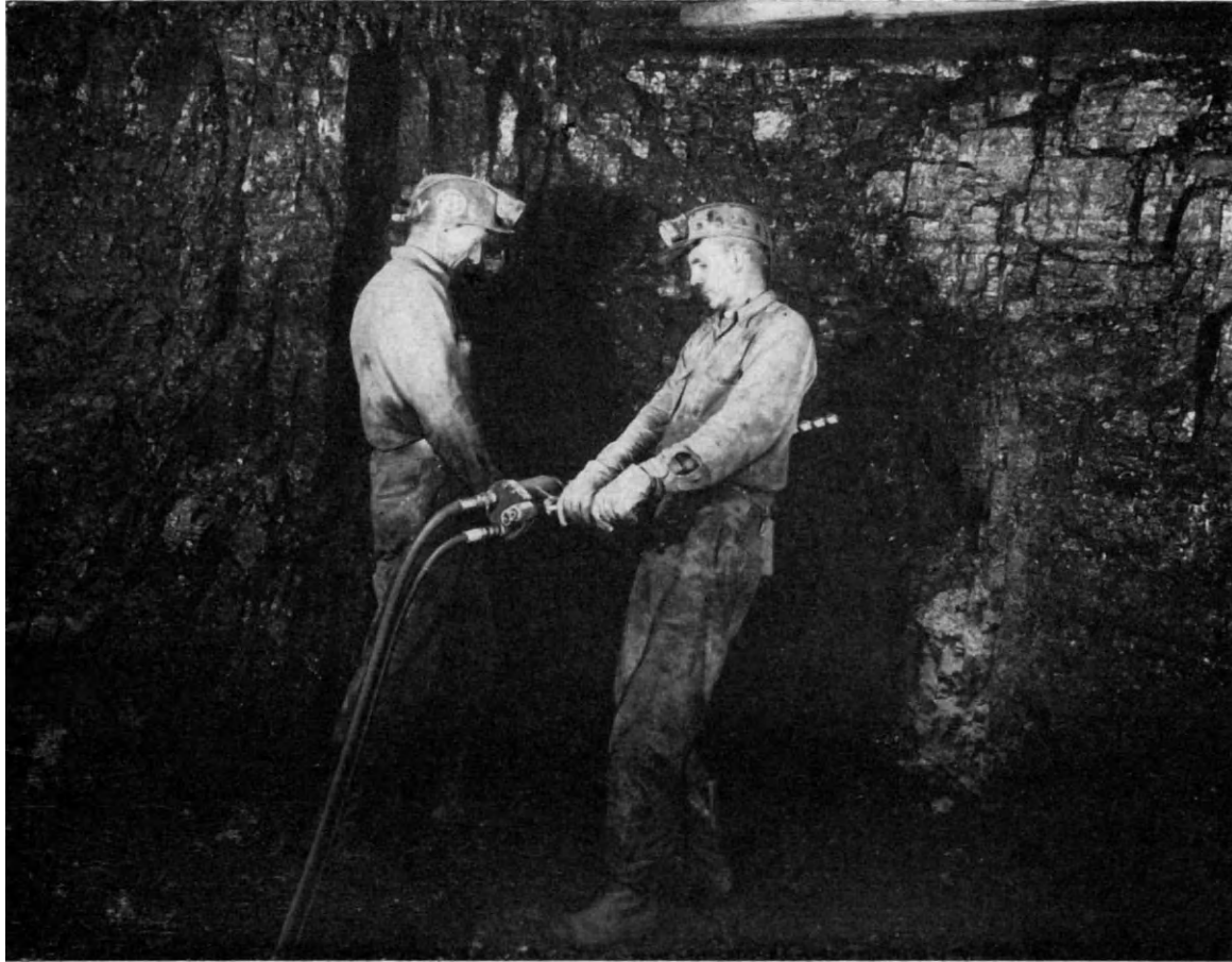
FIG. 9. Drilling the face. (Jeffrey Manufacturing Co.)
