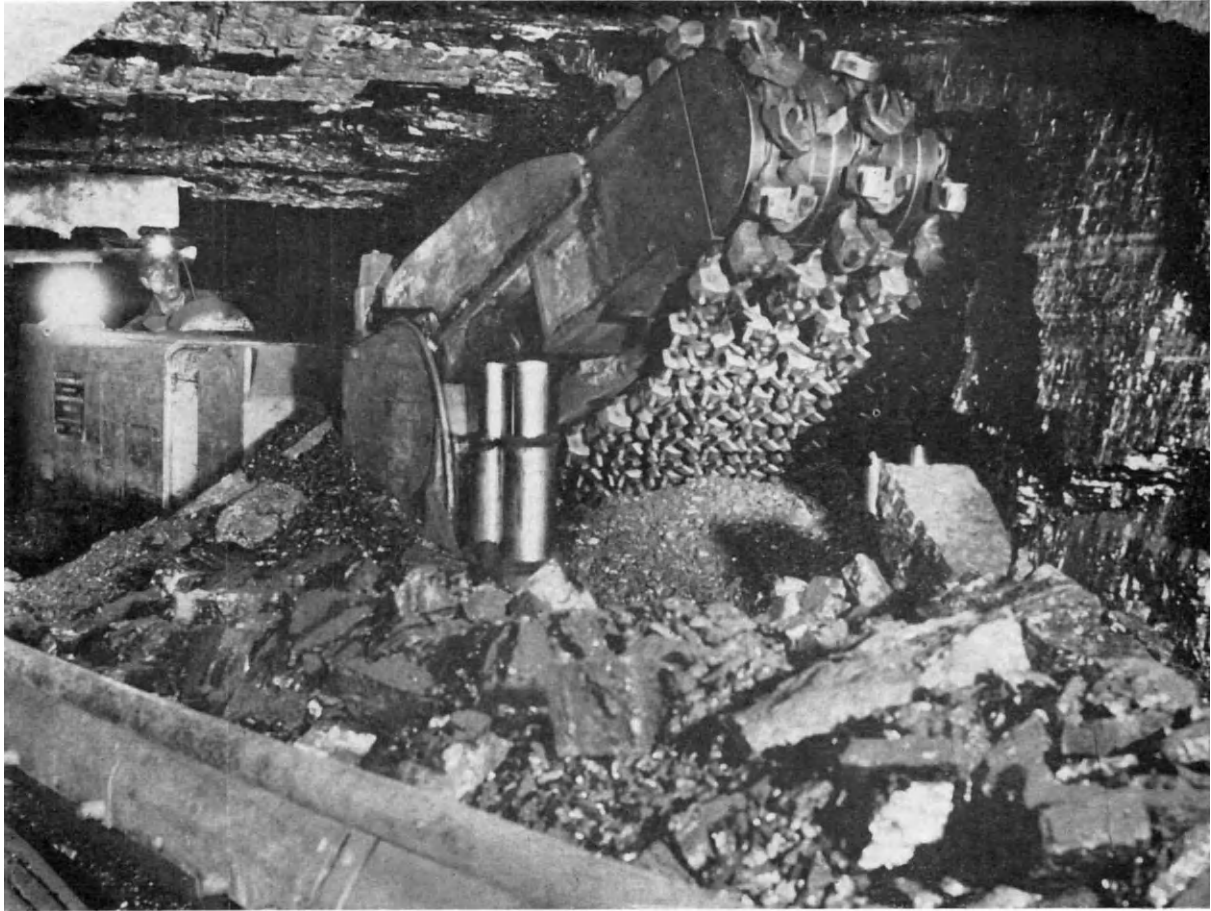
FIG. 16. Dosco Miner at work at the face. (Dominion Steel and Coal Corp., Ltd.)
