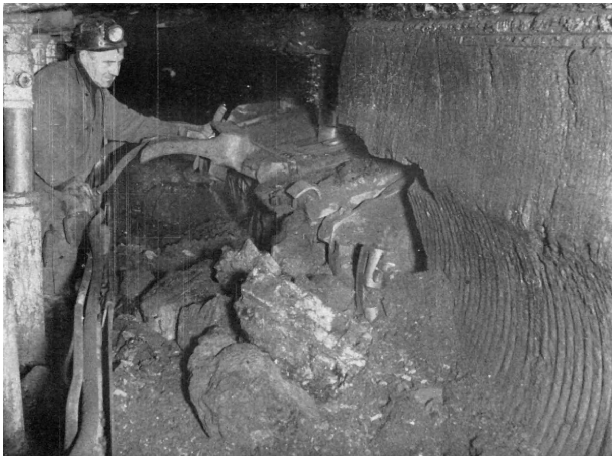
FIG. 5. A. B. trepanner at work underground. (Anderson, Boyes & Co., Ltd.)
