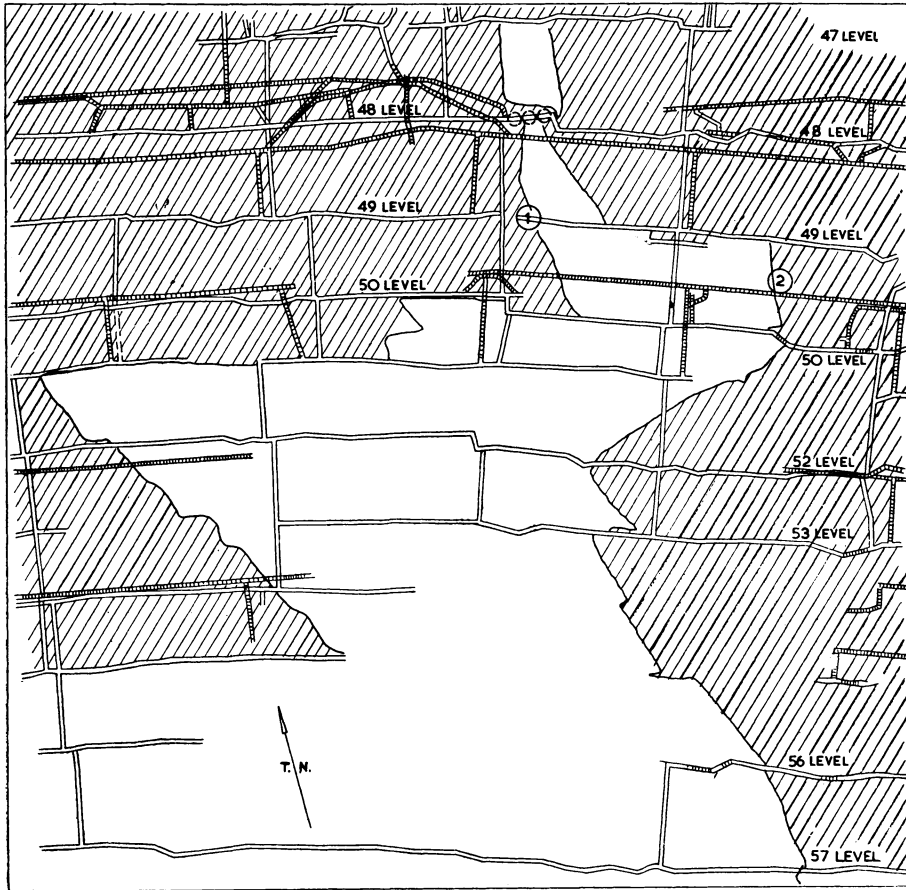
FIG. 12. East Rand Proprietary Mines, Ltd., plan showing localities of rock bursts ① and ② in stopes 49/50 E6E of the Angelo and 50W3W of the Hercules Section. (12)
