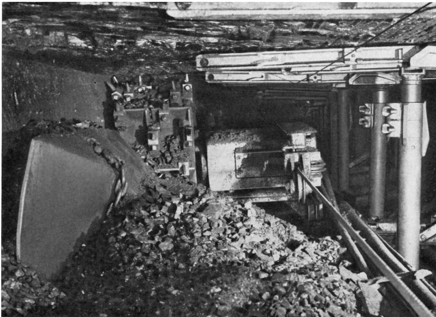
FIG. 2. B.J.D. 150 h.p. Anderton shearer with magnamatic control. (British Jeffrey-Diamond, Ltd.)
