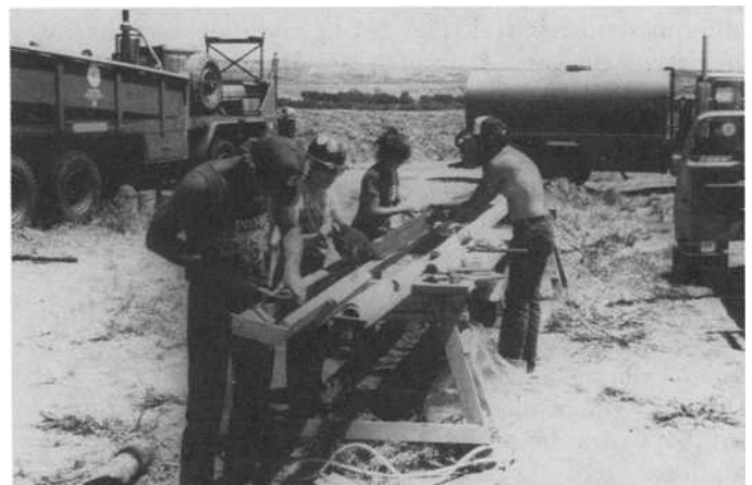
FIG. 12—Core tray on sawhorse with PVC tubes on drill site in Wyoming (coal core is covered with dampened cloth to inhibit moisture loss).
