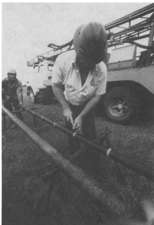
FIG. 13—Removing filament tape wrappings of split-tube core barrel after coring.
