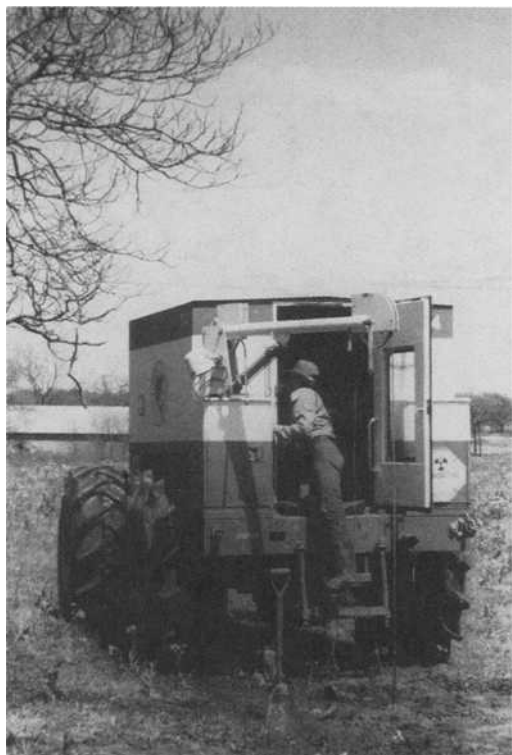
FIG. 9—Geophysical logging unit showing extended probe boom which has lowered probe down borehole.
