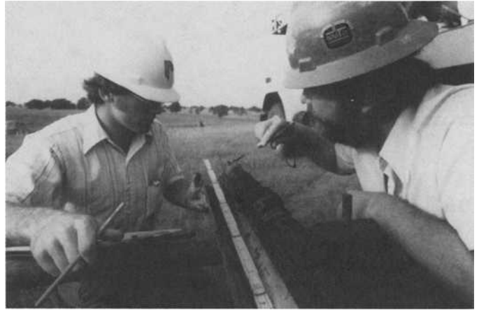
FIG. 16—Describing core to determine coal/rock contacts and core recovery using a split-tube core barrel.
