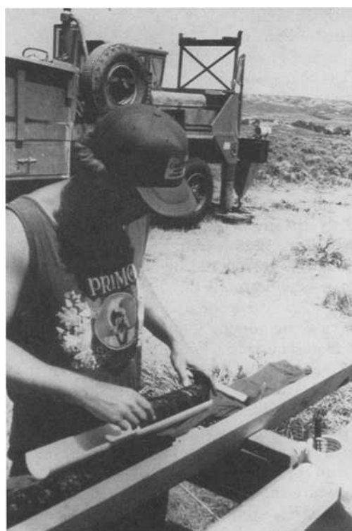
FIG. 22—Transferring coal core from tray to PVC tube half.
