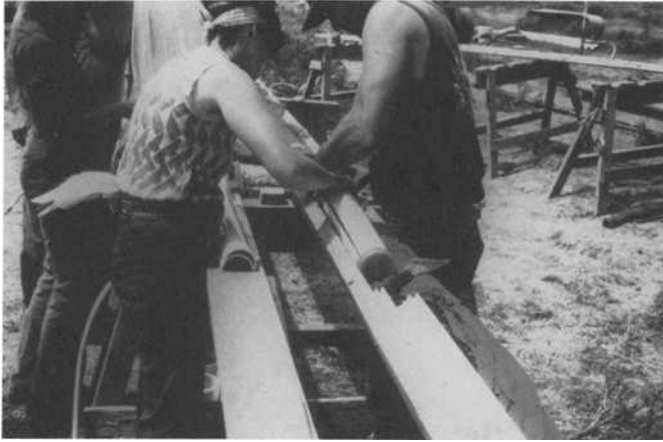
FIG. 23—Placing of second half of PVC tube on core sample.
