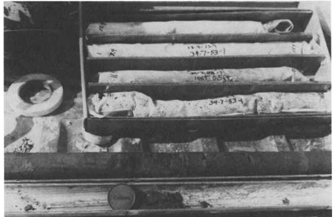
FIG. 25—Coal core packaged in plastic sleeves and arranged in vertical book fashion in core box.
