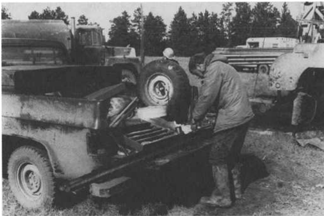
FIG. 24—Transferring of coal from split-tube barrel into plastic sleeves and placed into core box.
