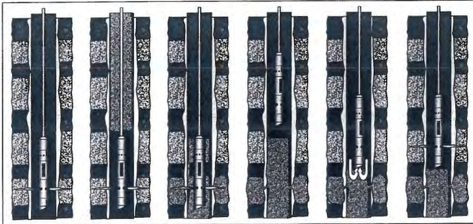
Fig. 7.18—CT string performing jet perforation and initiating fractures.
