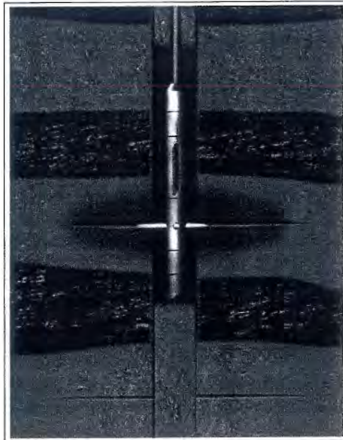
Fig. 7.19—Jet-perforating tool being lowered into the next interval to be treated.
