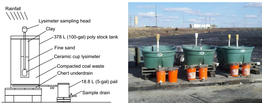
Fig. 13.2 Schematic and photograph of field-scale kinetic test columns [2].
