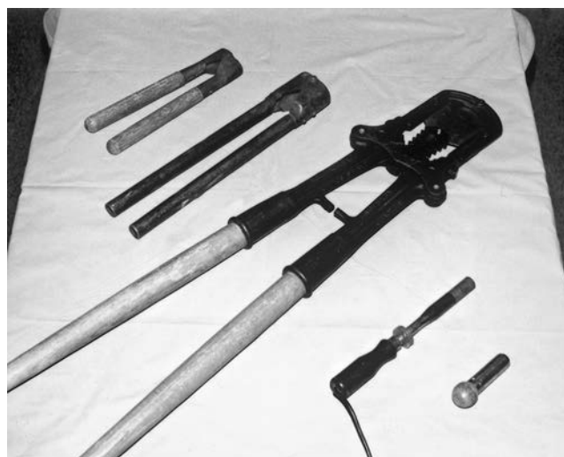
• Fig. 2.33 A variety of common dehorning instruments. From top to bottom: a small Barnes gouge, large Barnes gouge, Keystone dehorner, electric dehorner, and tube or Roberts dehorner.
