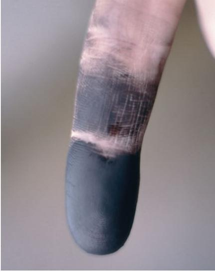
**Plate 5.24.** Black deposits from rubber parts indicate too high a level of hypochlorite resulting in rubber corrosion.
