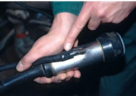
**Plate 5.31.** Hole in the short air tube.
