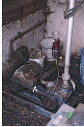
**Plate 5.1.** The vacuum pump shown has no belt guard to protect against injury and leaves staff at risk of becoming entangled in the belts (A).
