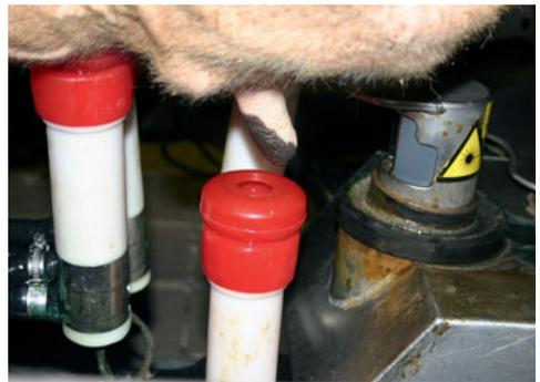
**Plate 5.15.** A robotic milking machine attaching a teat cup.
