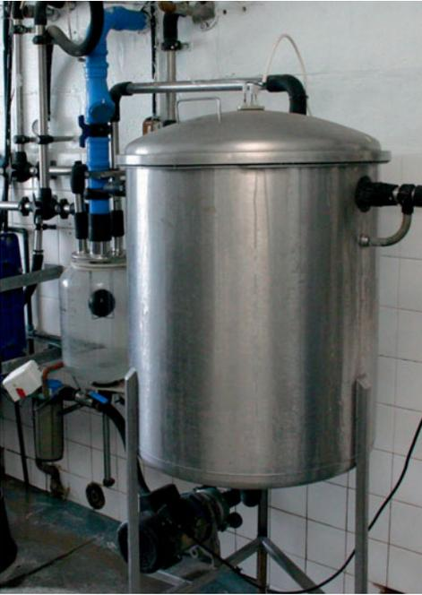
**Plate 5.8.** A stainless steel receiver vessel is resistant to breakage but difficult to inspect.
