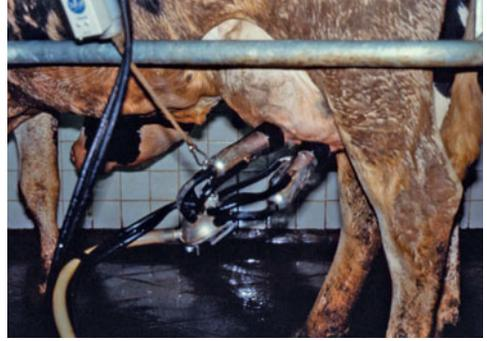
**Plate 5.11.** ACRs shut off the vacuum to the cluster at the end of milking. To prevent the unit falling on the floor and becoming contaminated, a cord is activated, which gently lifts the cluster off the cow.
