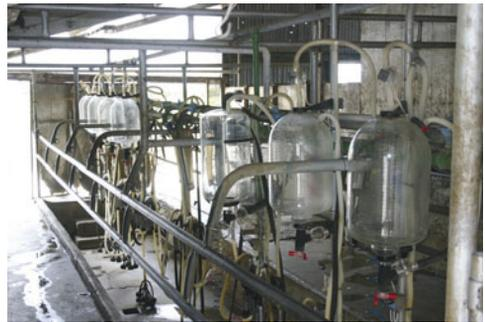
**Plate 5.29.** A combination of a recorder jar and direct to line parlour, which had a very poor milking performance.
