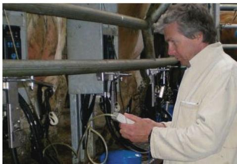
**Plate 5.16.** A dynamic test recording the vacuum levels and fluctuation during milking.
