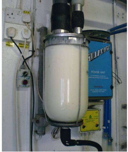
**Plate 5.36.** A flooded sanitary trap due to a faulty milk pump, which could not remove milk from the receiver vessel.
