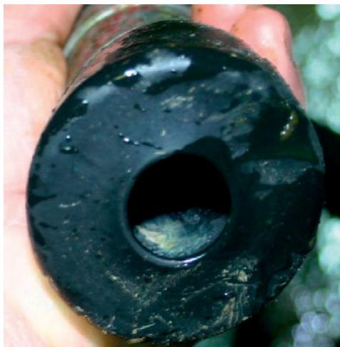
**Plate 6.24.** The liner of a dump bucket that has not been cleaned correctly. You can see the crud and the deposits inside the liner.
