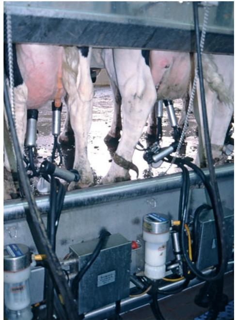
**Plate 5.10a.** Low line system, where the milk transfer line is below the level of the udder.
