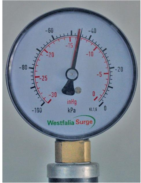
**Plate 5.7.** The vacuum gauge must be easy to read and visible throughout milking.
