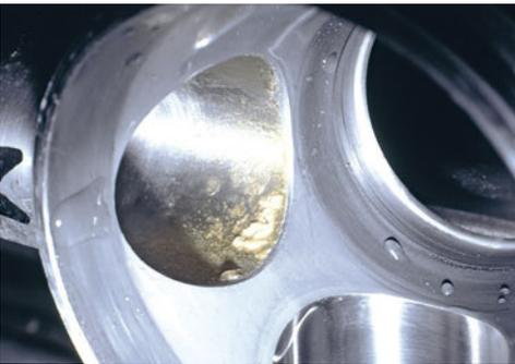
**Plate 5.26.** If there is insufficient turbulence or flow of wash solutions, cleaning may be ineffective, as shown.
