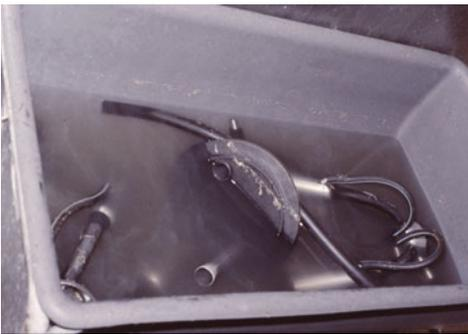
**Plate 5.28.** Cleaning will be ineffective as there is insufficient detergent solution to come into contact with all parts of the cluster.
