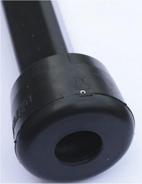
**Plate 5.12.** An air bleed at the top of the liner is claimed to give better milkout and smoother ACR function.
