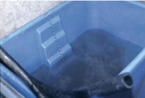
**Plate 5.25.** High levels of hypochlorite in the disinfection solution strip away rubber.
