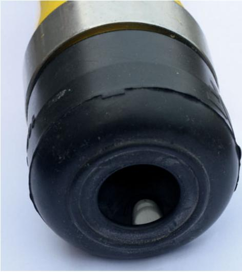
**Plate 6.25.** The flush solution is emitted from a small nozzle inside the mouth of the liner to minimize cross-contamination.
