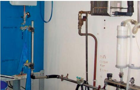
**Plate 5.27.** Acid boiling wash (ABW) relies on heat and acid for cleaning. Acid is put into the reservoir and released with the boiling water to run around the plant to waste.
