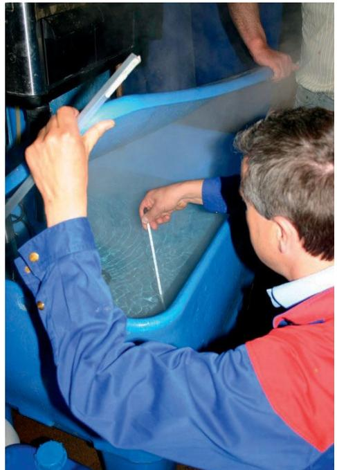
**Plate 5.22.** Checking the temperature of the hot wash solutions.
