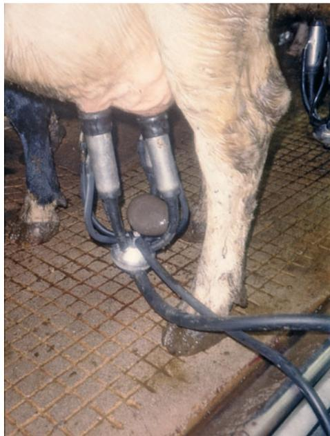
**Plate 6.20.** Milkers have been known to place stones or bricks on top of the clawpiece to try and speed up a slow milker. This is not recommended.
