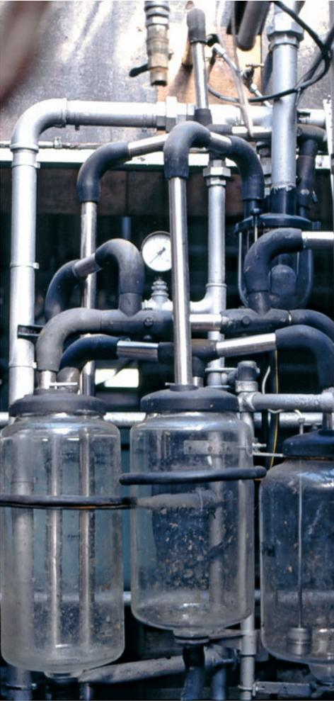
**Plate 5.30.** Excess bends in pipelines.
