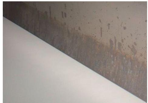
**Plate 10.3.** Soil, as shown in the dark line just above the milk, allows psychrotrophic bacteria to grow.
