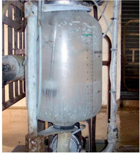
**Plate 10.2.** A dirty receiver vessel will increase the Bactoscan.
