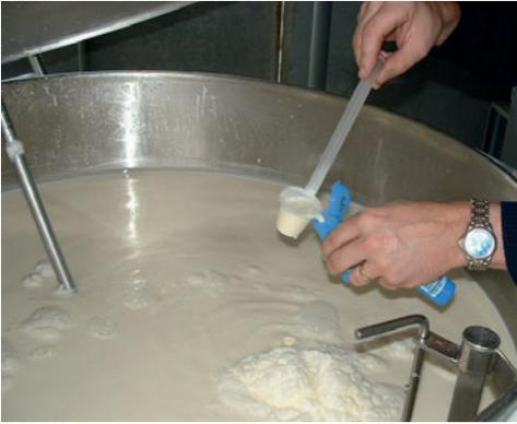
**Plate 10.5.** Milk samples must be collected from a well-agitated bulk tank and kept cold until they reach the lab.
