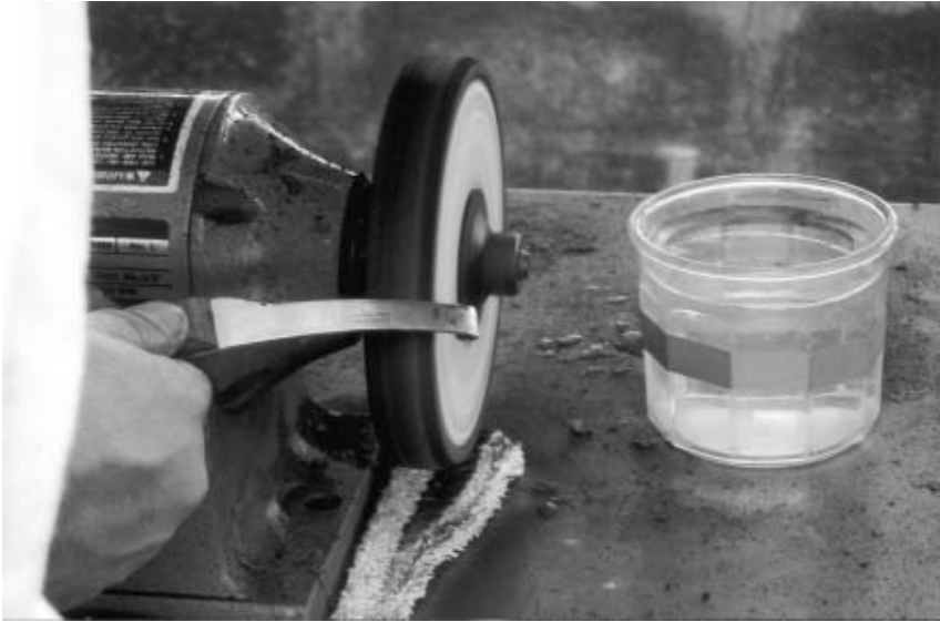
Figure 10.7. The cutting edge of the knife is placed at a 25°–30° angle against the grinding surface of the wheel and drawn across the full length of the cutting edge.
