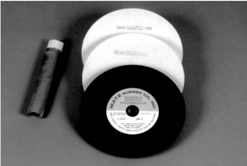
Figure 10.8. Rubberized and felt-type sharpening and buffing wheels.
