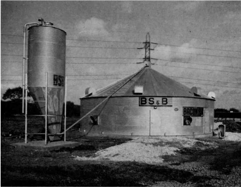
FIG. 10. Bacon Bin . The BSB 'Bacon Bin' has over 3000 sq. ft. of floor area with capacity for 46 sows and 437 other pigs of market weight. It is 48 ft. in diameter, has a fully controlled environment including automatic watering and feeding systems which complete the latter chore in 3\frac{1}{2} min. The 3000 gallon manure trench can be flushed into a liquid manure tank in 4 min. The 10 ft. high walls are constructed of galvanised steel, insulated with Styrofoam. Internally the 'Bin' is constructed in two levels, each floor housing 23 pens averaging 60 sq. ft. It has 3 heating units including an electric unit heater with an output of 80,000 B.t.u./hr.; and to provide warm creep areas in the lower pens at farrowing time a hot water system is provided in the concrete floor. In the upper pens radiant heat lamps are used. Ventilation is by 5 \times 24 in. exhaust fans each with an output of 27,000 c.f.m. The cost of the bin is between £9000 and £10,000 depending upon such local factors as preparation of foundations, site, etc.
