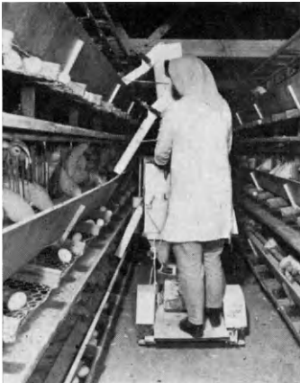
FIG. 36. A 4\frac{1}{2} cwt. electrically operated feed truck which travels down a 100 ft. length of Grossmith static cages, filling three feed troughs on the way down and the others on the return journey.
