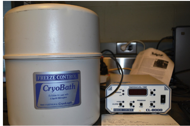
Figure 71.3 Programmable freezers for semen straws as well as embryos.
