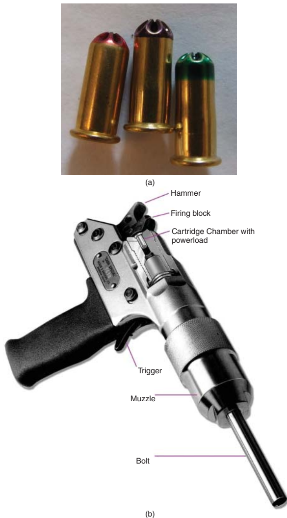
Figure 26.3 A CASH Special captive bolt gun (Reproduced courtesy of Accles & Shelvocke). (b) The bolt is shown extended for demonstration purposes. The inset (a) shows captive bolt cartridges in three power charges (from left to right: pink for calves, purple for heavy animals, green for bulls and very heavy animals).
