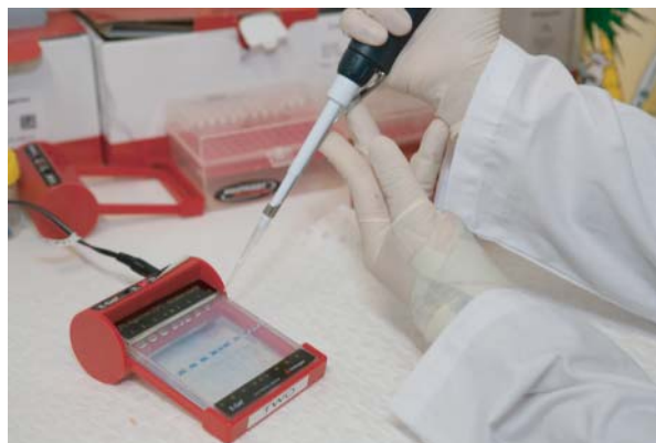
Figure 17.30 Loading a polyacrilamide gel with the product of the polymerase chain reaction.
