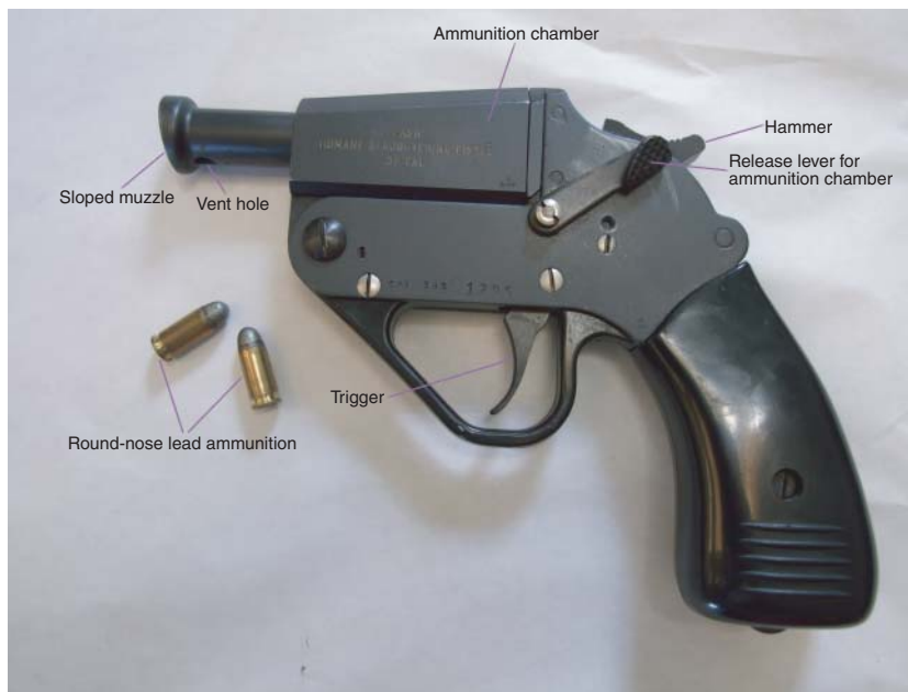
Figure 26.2 A single-shot, 0.32 calibre pistol, adapted for veterinary euthanasia, to be used with round-nose lead ammunition. Note the muzzle slope and vent hole in the barrel.
