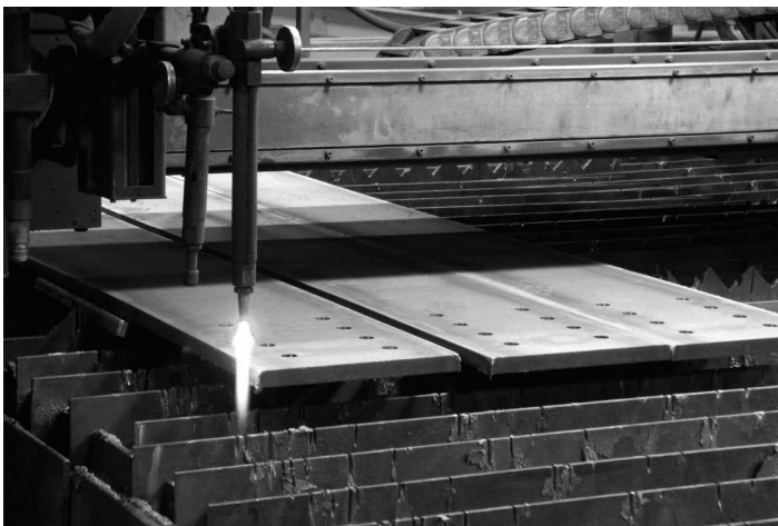
FIGURE 10.4 Controlled automatic cutting. (Courtesy of Y. Martin, Canam Bridges Inc., St. Foy, Qc, Canada. With Permission.)
