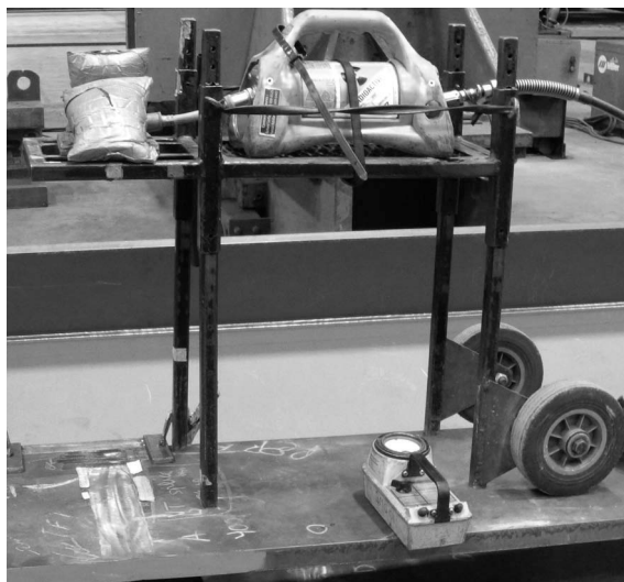
FIGURE 10.27 RT of weld. (Courtesy of Y. Martin, Canam Bridges Inc., St. Foy, QC, Canada. With permission.)
