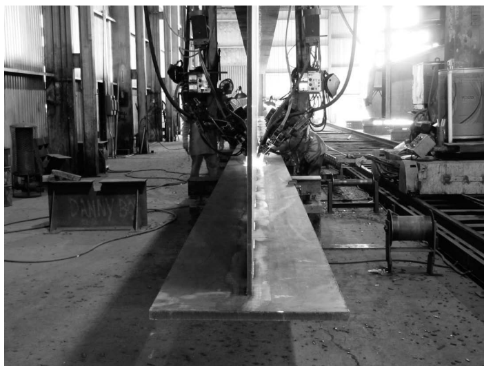
FIGURE 10.13 Balanced SAW welding of girder flange to web. (Courtesy of Dr. Frank, Hirschfeld Industries, Austin, TX, USA. With permission.)
