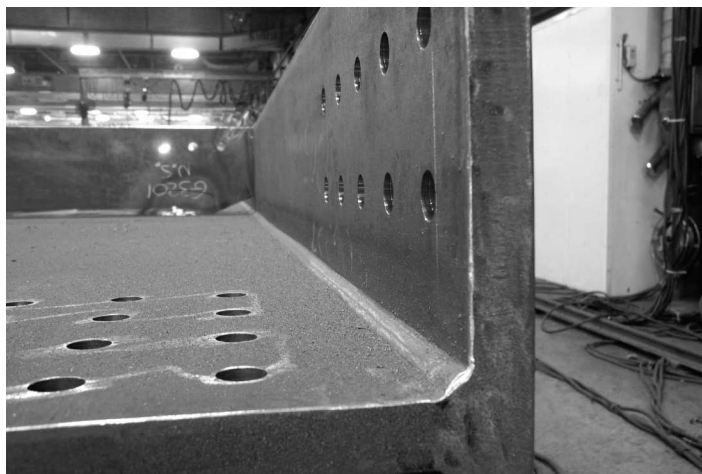
FIGURE 10.19 Plate girder flange-to-web fillet weld. (Courtesy of Y. Martin, Canam Bridges Inc., St. Foy, QC, Canada. With permission.)
