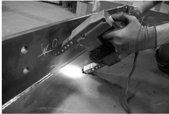
FIGURE 10.25 MPT of weld. (Courtesy of Y. Martin, Canam Bridges Inc., St. Foy, QC, Canada. With permission.)
