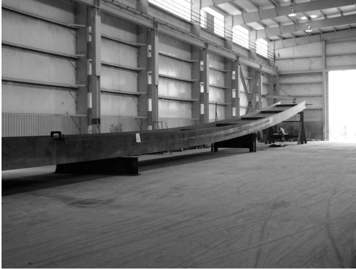
FIGURE 10.7 Weak direction curvature of a plate girder. (Courtesy of Dr. K. Frank, Hirschfeld Industries, Austin, TX, USA. With permission.)
