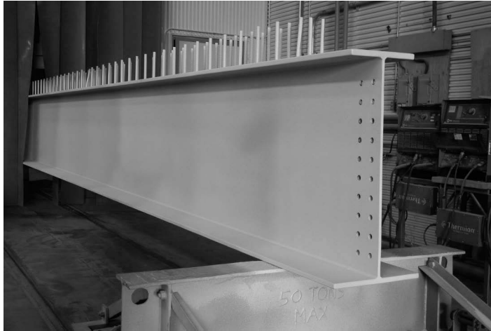
FIGURE 10.24 Shop painted beam. (Courtesy of Y. Martin, Canam Bridges Inc., St. Foy, QC, Canada. With permission.)
