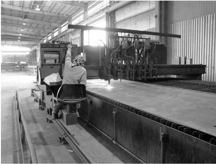
FIGURE 10.5 Flame cutting girder flange plates. (Courtesy of Dr. K. Frank, Hirschfeld Industries, Austin, TX, USA. With permission.)
