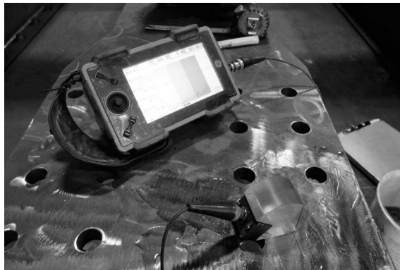
FIGURE 10.26 Ultrasonic testing of weld. (Courtesy of Y. Martin, Canam Bridges Inc., St. Foy, QC, Canada. With permission.)
