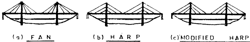
FIG. 17.13 CABLE ARRANGEMENTS FOR CABLE-STAYED BRIDGES
