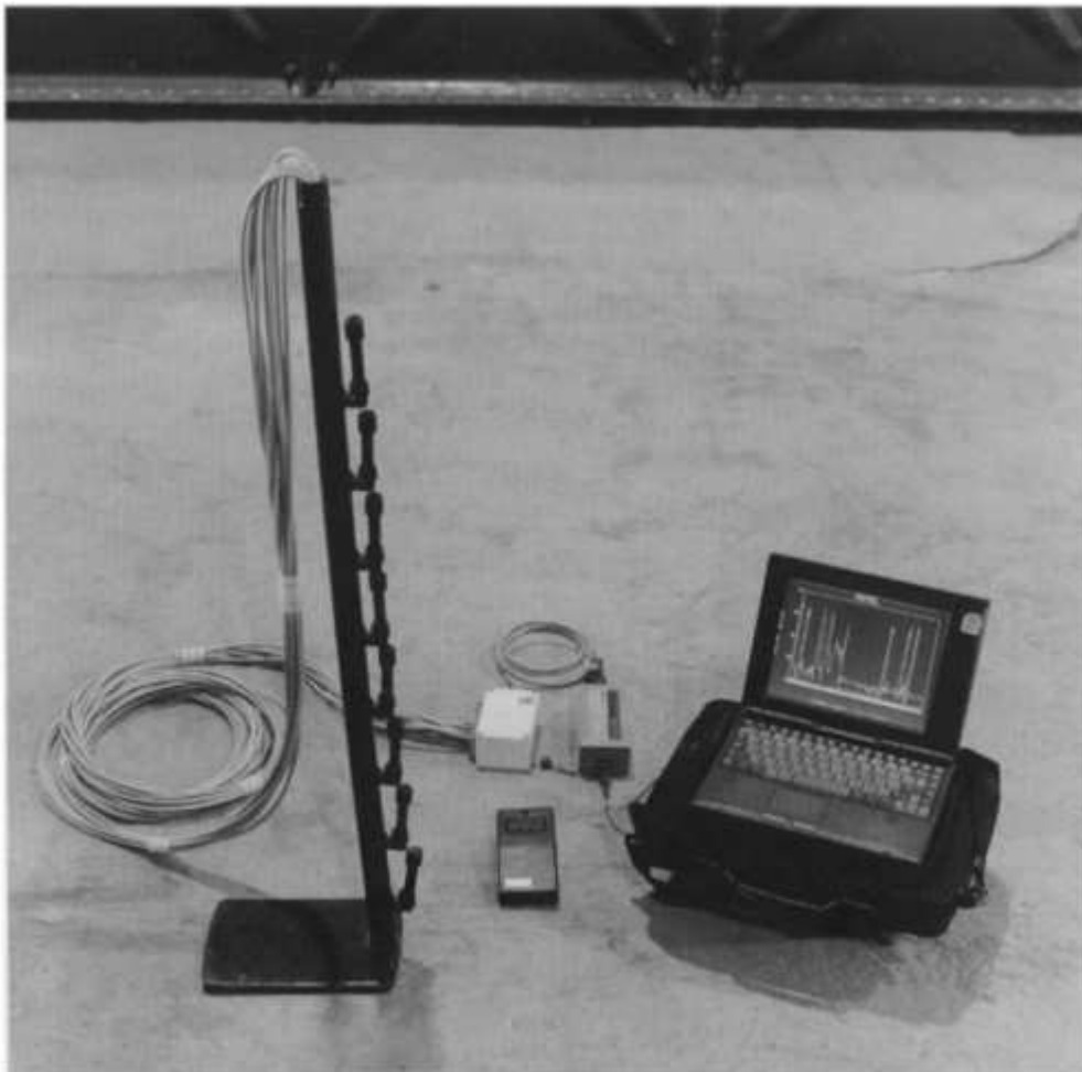
Fig. 8.3 The HR Wallingford 'Tell-Tail' scour monitoring system. One or more motion sensors are buried at different levels within the river bed, adjacent to the structure. Under normal conditions a buried sensor does not move, but when exposed by scour it begins to oscillate in the flow, triggering an alarm at the surface. The system also allows a real-time assessment of scour depth, and indicates whether scour hole refill has occurred. (Reproduced by permission of HR Wallingford Ltd)
