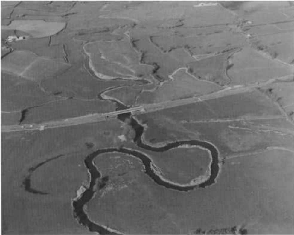
Fig. 1.13 Axe Bridge, Colyford, Devon, illustrating the problem of lateral shifting of the channel and route selection. The meander (bottom centre) looks as though it will be cut off at some time, possibly within the life of the bridge. When this happens the reduced channel length could increase velocities and cause degradation (see Fig. 8.8 ). An old ox-bow can be seen on the left. (Reproduced by permission of Devon Library Service)
