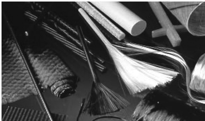
FIGURE 16.1 Available shapes of FRP products. (From ISIS, Design Manual 3: Reinforcing Concrete Structures with Fibre Reinforced Polymers . ISIS Canada, Intelligent Sensing for Innovative Structures, A Canadian Network of Centres of Excellence, University of Manitoba, Winnipeg, Manitoba, Canada, 2007a. With permission.)
