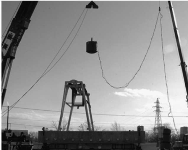
FIGURE. 21.19 Pictorial view of falling-weight impact test of full-scale RC girder.
