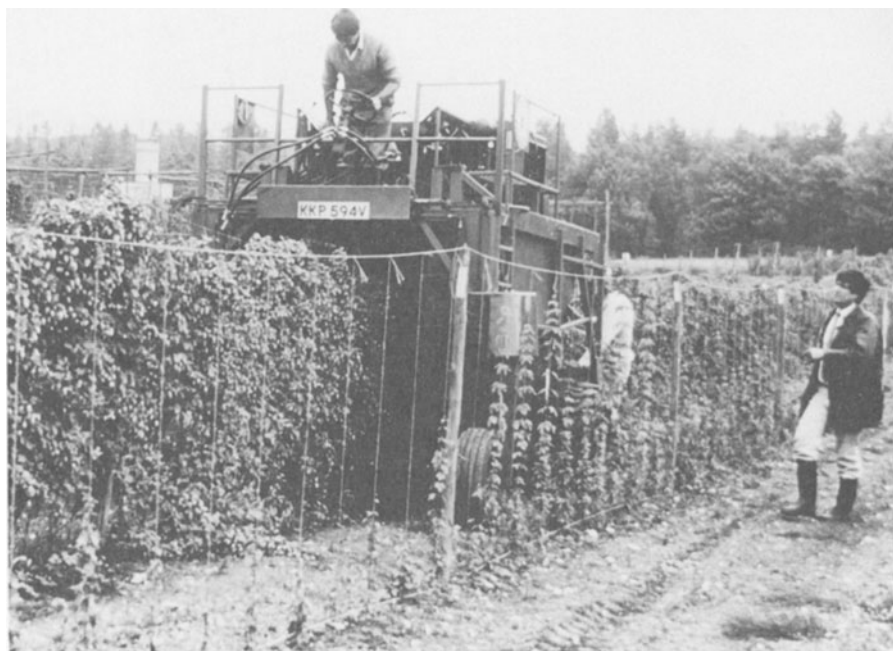
Figure 3.9 Prototype harvester picking dwarf hops on 2m high wirework (IHR, Wye).
