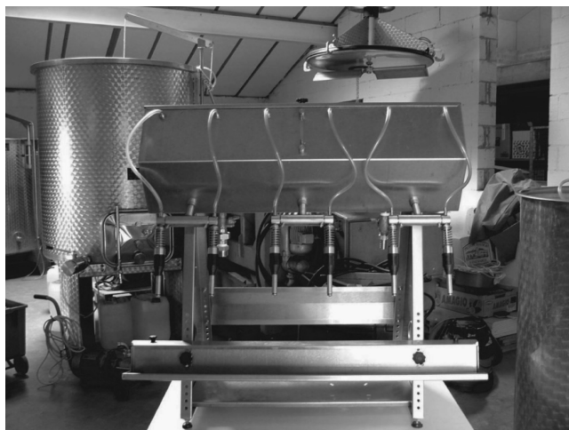
Figure 2.9.12 A six head wine bottle filler, typical of those used in small wineries. Photograph used by courtesy of Derek Pritchard, Dunkery Vineyard, UK
