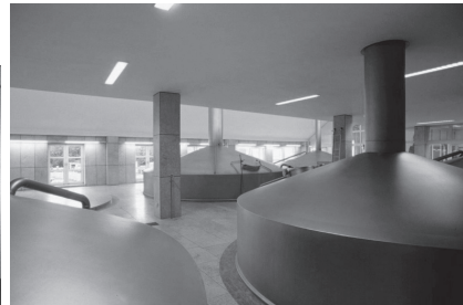
Closed kettles with stacks at Schneider Brewery, Kelheim, Germany. Photo courtesy of G. Schneider & Sohn GmbH.
