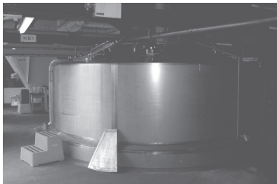
Hop back at Hardy's and Hanson's brewery (Kimberley, UK). The copper is directly above.
