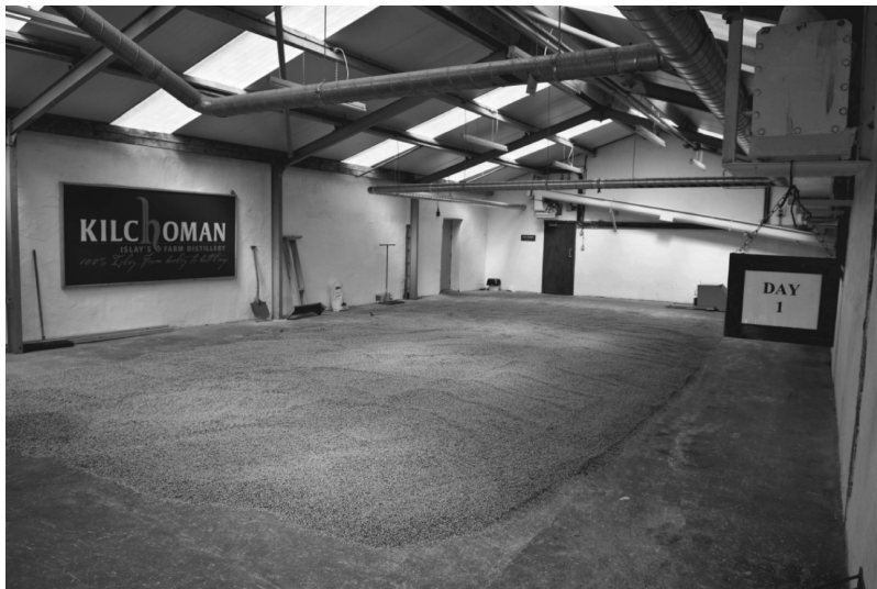
Figure 3.2.5 The malting floor at Kilchoman Distillery, Islay. Photo used by courtesy of Kilchoman Distillery, Scotland
