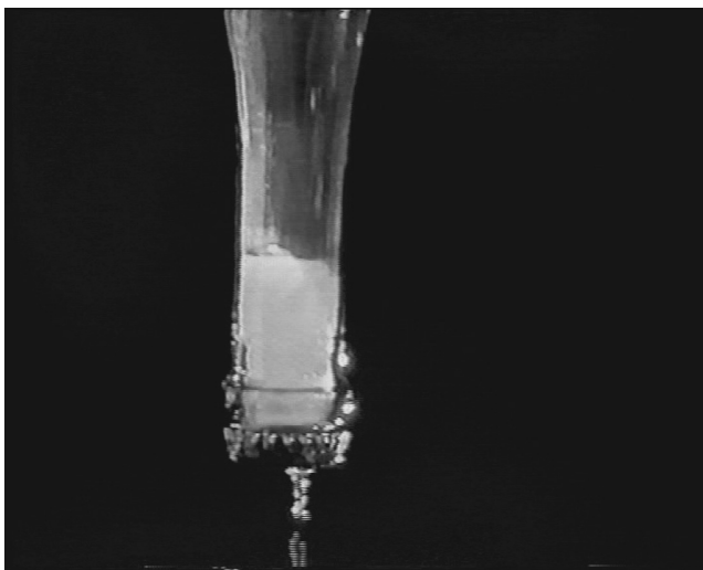
Figure 2.9.21 The yeast plug compacted in the neck of the bottles. Photograph by courtesy of J.C. Le Roux, South Africa
