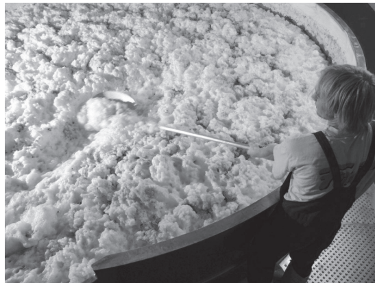
Rousing fermenting wheat beer wort at the Schneider Brewery, Germany. Photo courtesy of G. Schneider & Sohn GmbH.
