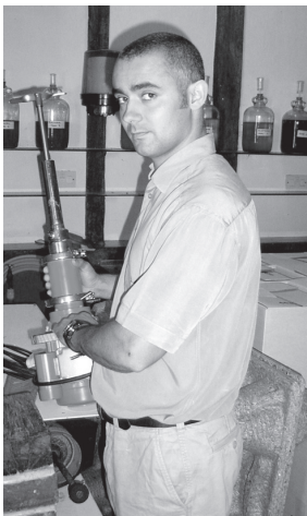
Impeller type fruit macerator at Lurgashall Winery, UK.
