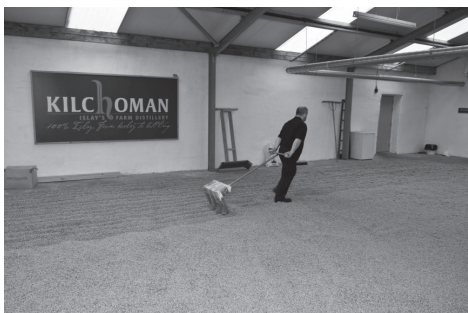
(a) Grubbing the malt on Kilchoman distillery malting floor
