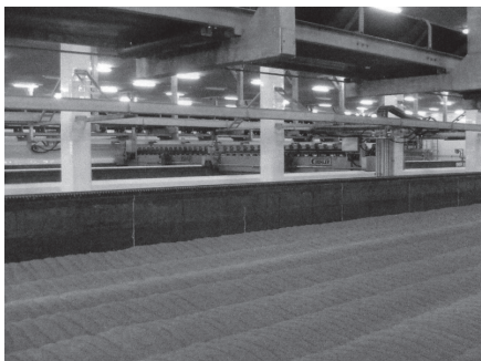
(e) Germbox horizontal germination plant
