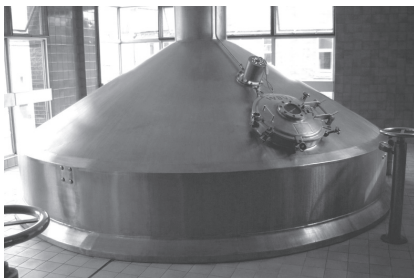
Enclosed kettle with stack at Hardy's and Hanson's brewery.
