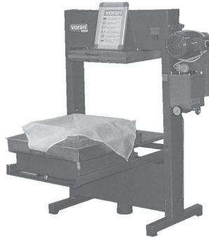
Rack and cloth press. Photograph by courtesy of Vigo Ltd.
