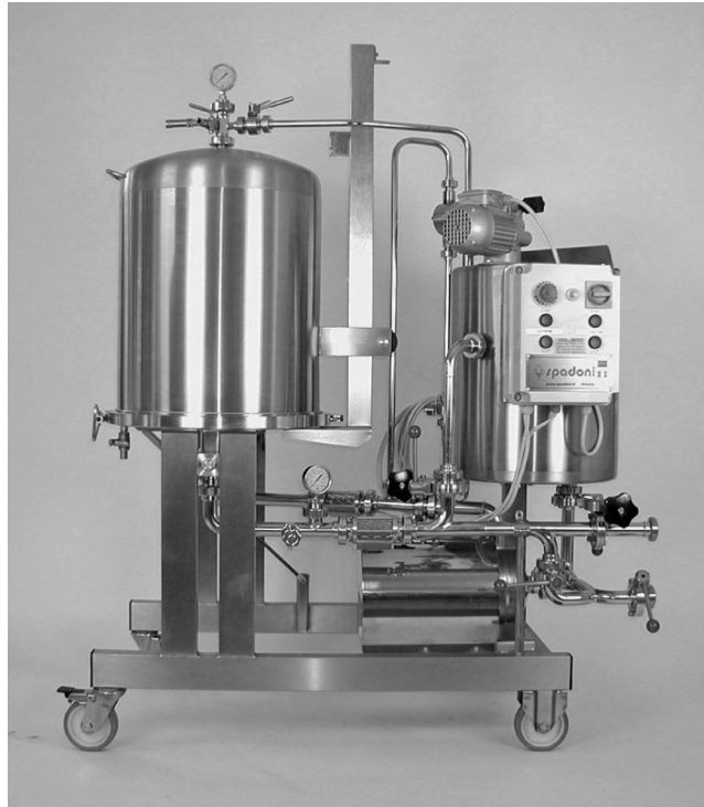
Figure 2.9.27 Earth filtration system. Commonly used to filter cider and beer as well as wine. Photograph by courtesy of Vigo Ltd., UK
