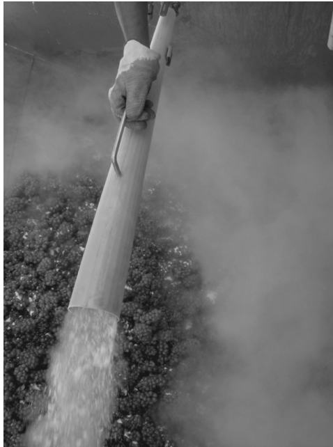
Figure 2.9.6 Spraying dry ice on grapes awaiting processing at KWV, Paarl, South Africa. Photograph courtesy of Paul Gerber
