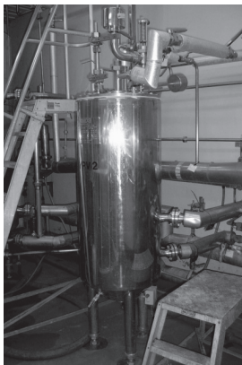
Medium yeast propagation vessel at Belhaven Brewery. Smaller and larger vessels form the complete system.
