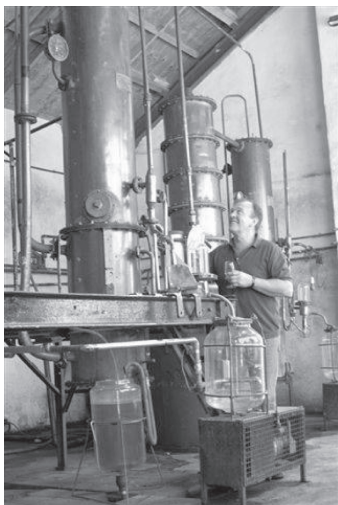
Batch columnar stills at the Somerset distillery, UK. Photograph by courtesy of the Somerset Distillery.
