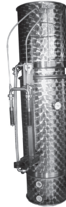
A flash pasteurizer. Photograph used by courtesy of Derek Pritchard, Dunkery Vineyard, UK and KTM.
