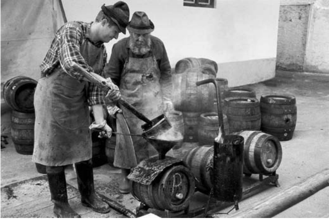
Figure 6.1. “Pitching” a barrel of beer—i.e., coating the interior with an inert waterproof seal that separates the beer from the wood of the barrel. Photo courtesy of the Bavarian Brewers Federation, Munich, Germany.
