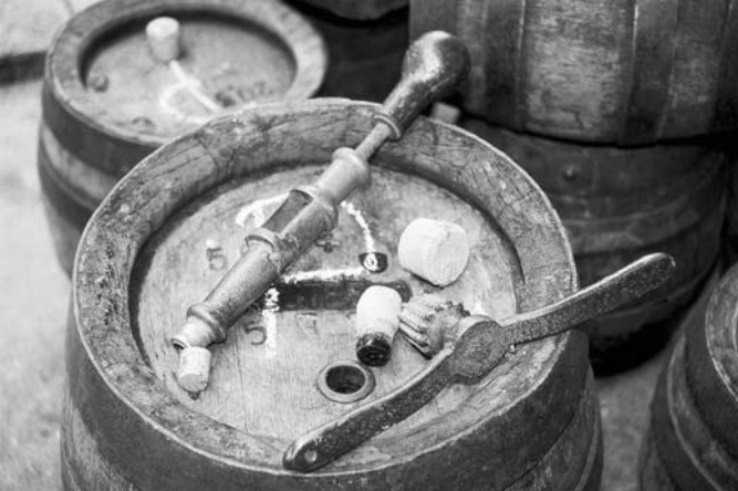
Figure 6.2. A barrel must be provided with a bung hole for a spigot tap. Photo courtesy of the Bavarian Brewers Federation, Munich, Germany.
