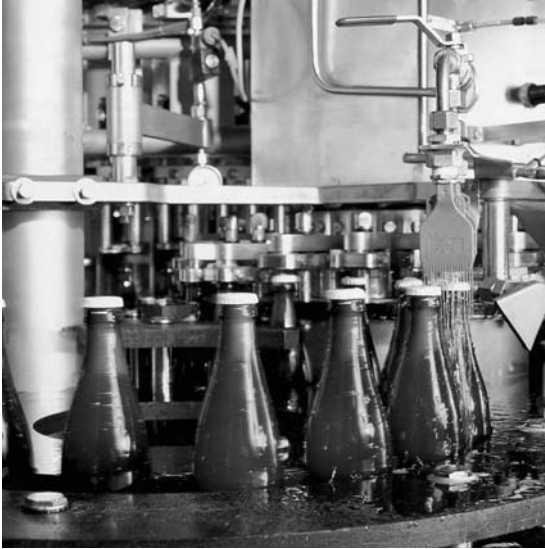
Figure 6.6. Beer bottles being filled and capped. Photo courtesy of the Bavarian Brewers Federation, Munich, Germany.
