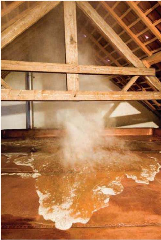
A cool ship at a commercial brewery in Belgium receives wort from the boil kettle the old-fashioned way. The cooling wort is exposed to wild yeast in the bacteria that is in the air, which facilitates fermentation.
