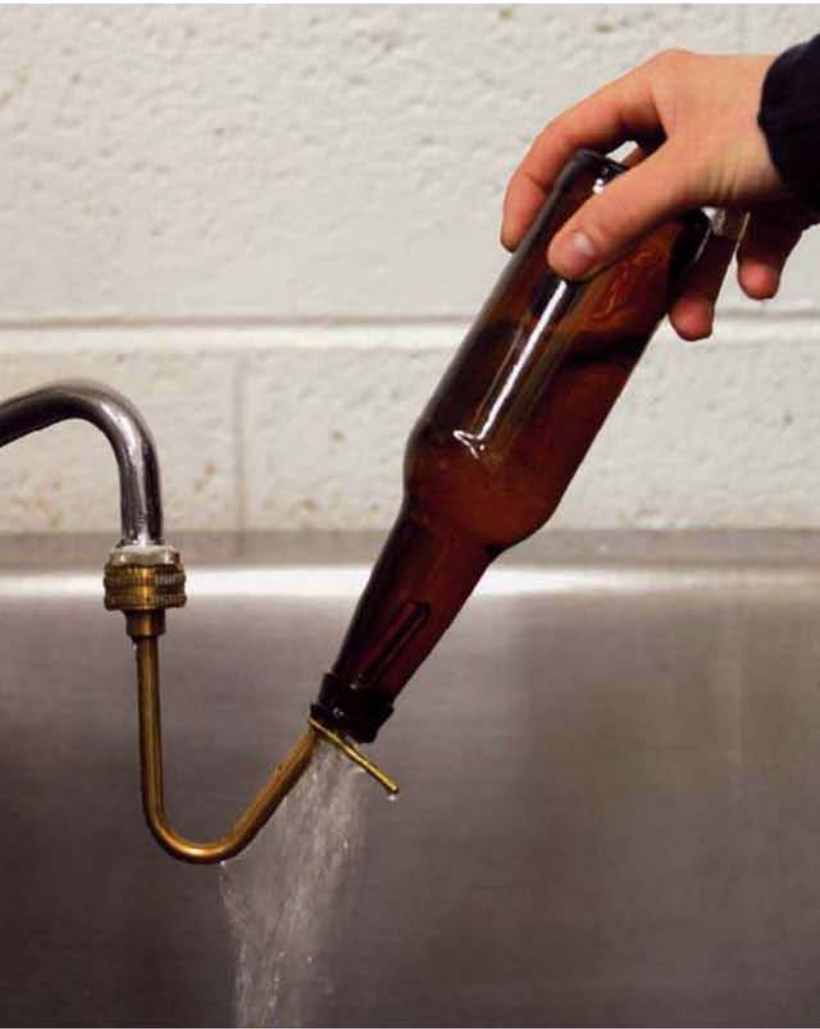
A specially designed bottle rinser is indispensable for sanitizing your bottles.
