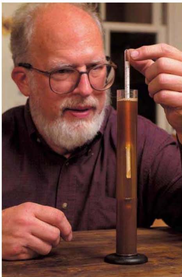
P. Read the hydrometer by bobbing it in a cylinder of beer.
