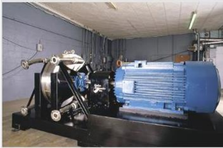
The rotor inside the Hydrosonic Pump™ generates shock waves to provide the energy needed to heat various liquids, such as organic salt used by the petroleum industry.
