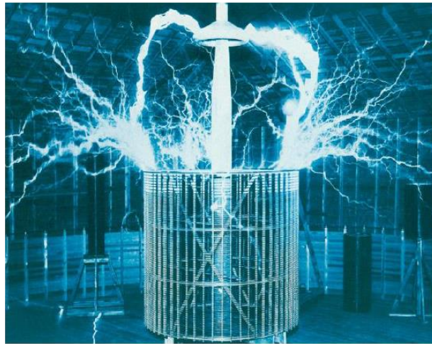
The flame-like discharge of an electrical oscillator giving twelve million volts which measure sixty-five feet across, Colorado Springs Laboratory.
