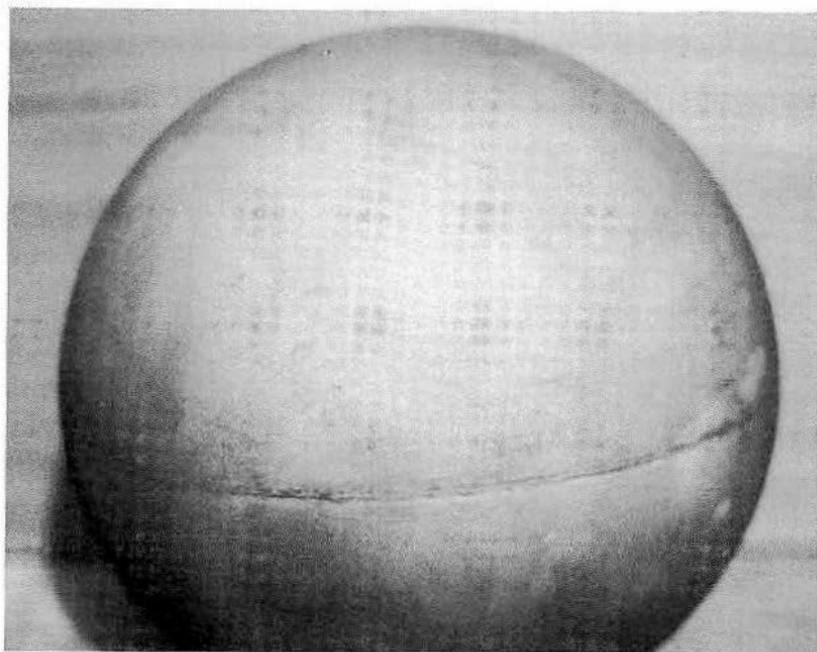
*A twelve inch plastic sphere has been coated with graphite and is ready to be plated.*
