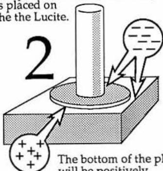
The bottom of the plate will be positively charged. The top of the plate and Lucite block will acquire a negative charge.
