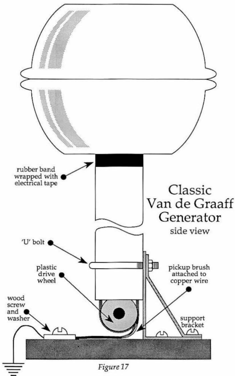
sphere of the proper dimensions. Besides, two bowls allow easy access to the top roller and brushes, and I wanted to test my hunch that almost as much power could be obtained from the bowls if the edges were heavily doped and insulated as could be obtained from a traditional spherical terminal.
