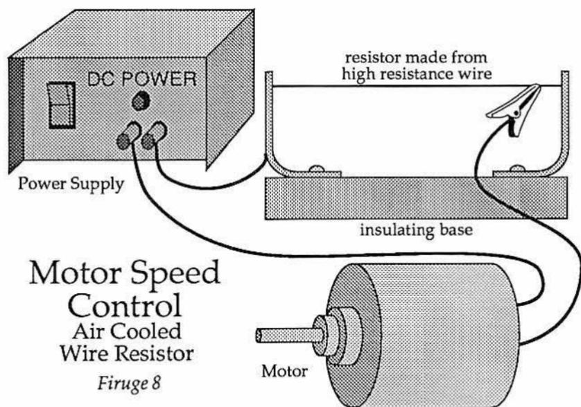
between two copper posts. One side of the wire is tied to a 12v (or similar) power supply. A wire coming from your motor is attached to an alligator clip which can be moved along the wire to increase or decrease the motor speed. This method works extremely well. However, be aware that the wire can become red hot when supplying current to the motor! Make sure to house it safely.
