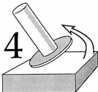
The plate and handle assembly is removed at an angle by lifting one side of the plate away from the block without breaking contact on the other side.
