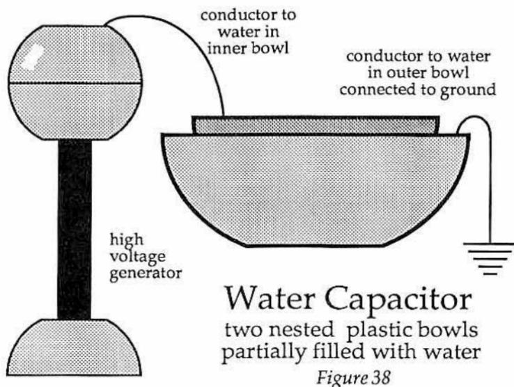
insulated metal trays which were filled partially with water. By connecting these water capacitors in parallel, Tesla could reach very large storage potentials with a minimum of effort.
