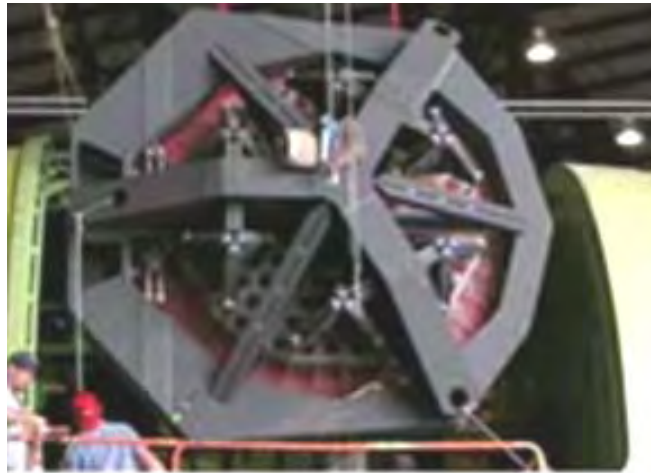
The primary mirror being lifted into the Telescope Assembly inside the plane (July 2003)
