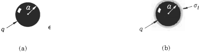
FIG. 8.14 Two methods of calculating the electric field of a charged body surrounded by a dielectric. (a) Direct calculation. (b) Dielectric is replaced by an equivalent charge distribution.
