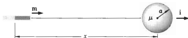
FIG. 14.17 Calculation of the force exerted on a sphere by a magnet.
