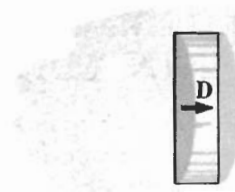
FIG. 8.2 To measure displacement field in a material medium, a coin-shaped cavity or a short cylindrical cavity is used.
