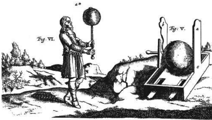
Figure 4.7: Guericke's experiment in which he kept a feather floating above a rubbed sulphur globe, together with his electrical machine.
