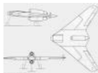
Gotha P 60 (Year: JAN 1945 Speed: 915 Km/h; Altitude: 12.500 m; Motors: BMW 003 )
