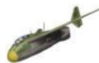
Junkers Ju EF 128 (Year: FEB 1945 Speed.: 990 Km/h; Altitude: 13.700 m; Motors: Heinkel He S 011)
