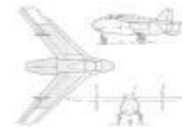
Junkers Ju EF 128 (Year: FEB 1945 Speed.: 990 Km/h; Altitude: 13.700 m; Motors: Heinkel He S 011)
