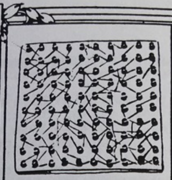
HERE, MR. PERRIGO SAYS, IS HIS SECRET THE ONE HUNDRED LITTLE SPRING COILS OF COPPER WIRE—BREAK UP THE EMBROIDERY WAVES AND CONDUCT THE ELECTRICITY THEY GATHER INTO THE BIG GENERATING COIL. THERE ARE TWO OF THESE PLATES, IDENTICAL IN APPEARANCE, BUT DIFFERENT IN WIRING.
