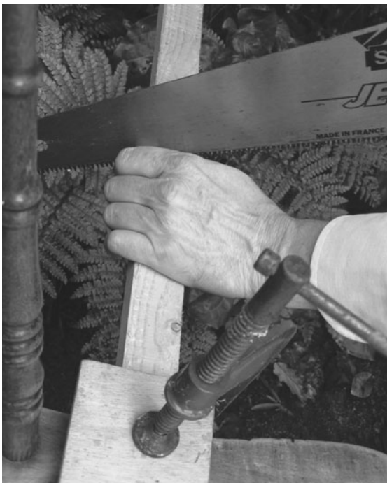
When starting a saw cut, line the last joint of your thumb up parallel to the cutting line, and rest the saw blade against it as a guide. Make the first few passes very gentle, with no downward pressure on the saw.
