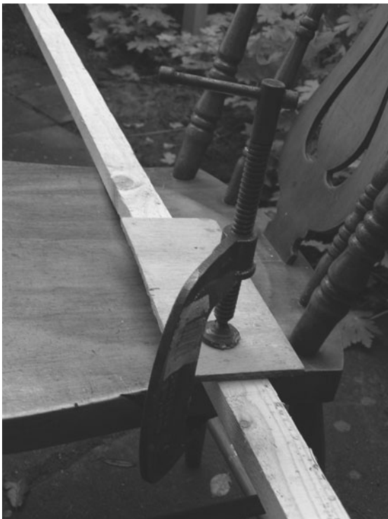
It's essential to clamp the work securely in order to make a clean saw cut.
