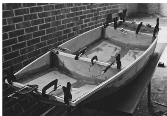
Whenever you take a trip to the hardware store, always buy at least one clamp. They soon accumulate, and it's almost impossible to have too many, as you can see illustrated here with this Mouse.
