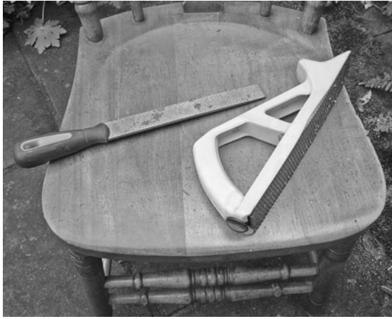
A rasp and a Stanley Surform tool make rounding corners, smoothing curves, and relieving edges easy.
