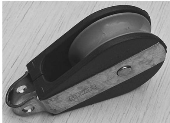
An inexpensive non-roller-bearing block suitable for a main sheet. Blocks like these work fine in small boats—there's no need to buy more expensive models with ratchets or races of bearings.
