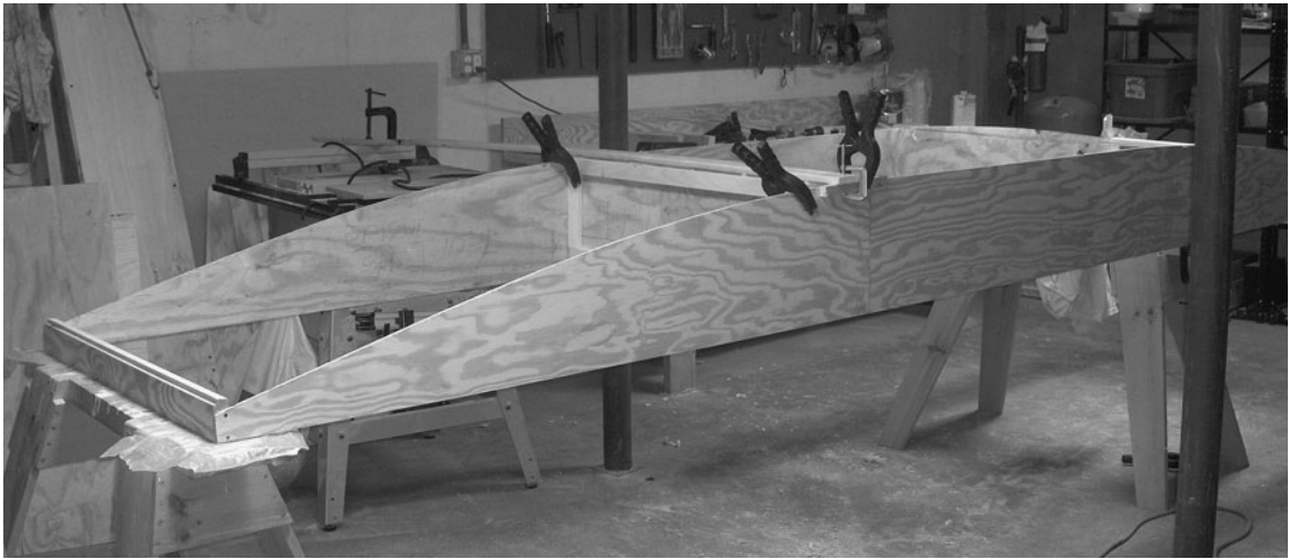
Hull assembly in process. Bow and stern transoms have been glued and ring-nailed to the side panels. The #2 bulkhead is clamped in place; ring nails will be added after the glue sets. A temporary strut has been clamped from the hull to a nearby solid object to counteract a bend in the warped plywood side panels while the glue dries. Note that the bow transom has been left “proud”; it will be planed down to match the curve of the bottom later. (Robert Holtzman)
