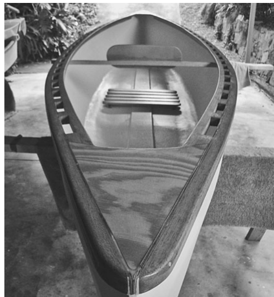
Details of gunwales, gapped inwales, and breasthook, in process (top) and nearly complete (bottom). Note also the seat added by the builder.
