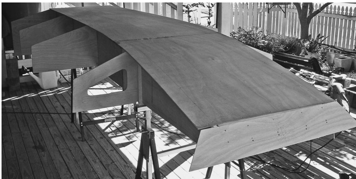
The bottom, previously butt-jointed, is attached to the framework. Note the neatly countersunk holes for the fasteners.
