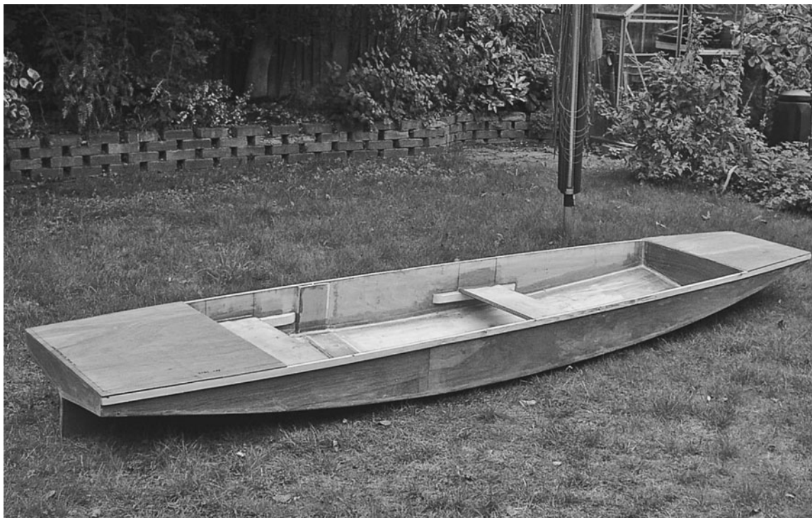
The nearly-finished Cruising Mouse built by Anthony Smith in Chapters 3 and 4. So many of the general construction details are clearly visible without a coat of paint. Note the butt-strapped sides and bottom; the “seat bearers” or cleats supporting the thwarts; the neatly-filleted-and-taped interior seams; and the treatment of the decks and gunwales. (Anthony Smith)
