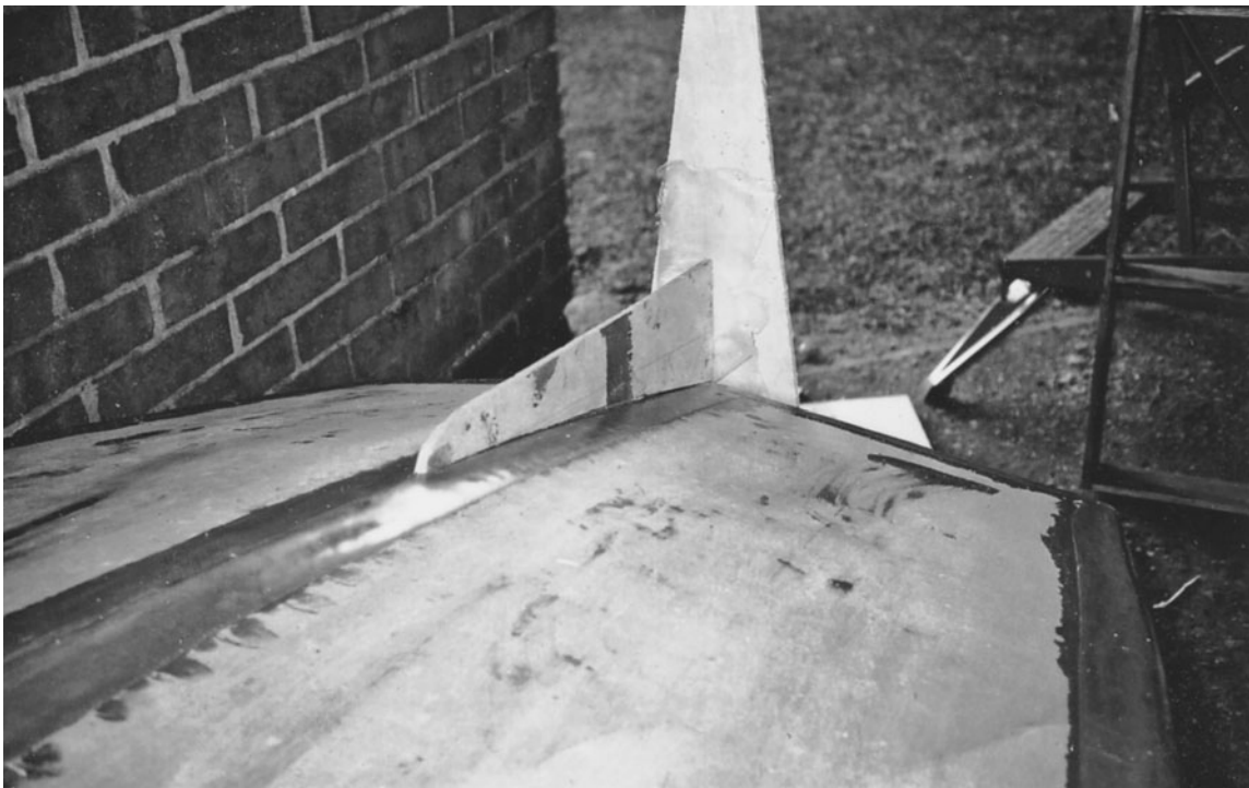
Using a scrap of plywood to hold the skeg of a Mouse upright. Notice that small gap between the skeg and the hull left by the builder? It's not a problem. Fill it with thickened epoxy and fillet and tape the joint on both sides, and it'll be strong enough. This Mouse was built by the author.
