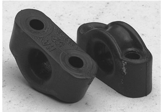
Inexpensive plastic deadeyes can serve a multitude of purposes on small boats, from providing an attachment point for a bow painter, to serving as rudder gudgeons. Make sure you back up the hull panel where these are attached with a reinforcing scrap of plywood—likewise with mounting cleats and such.
