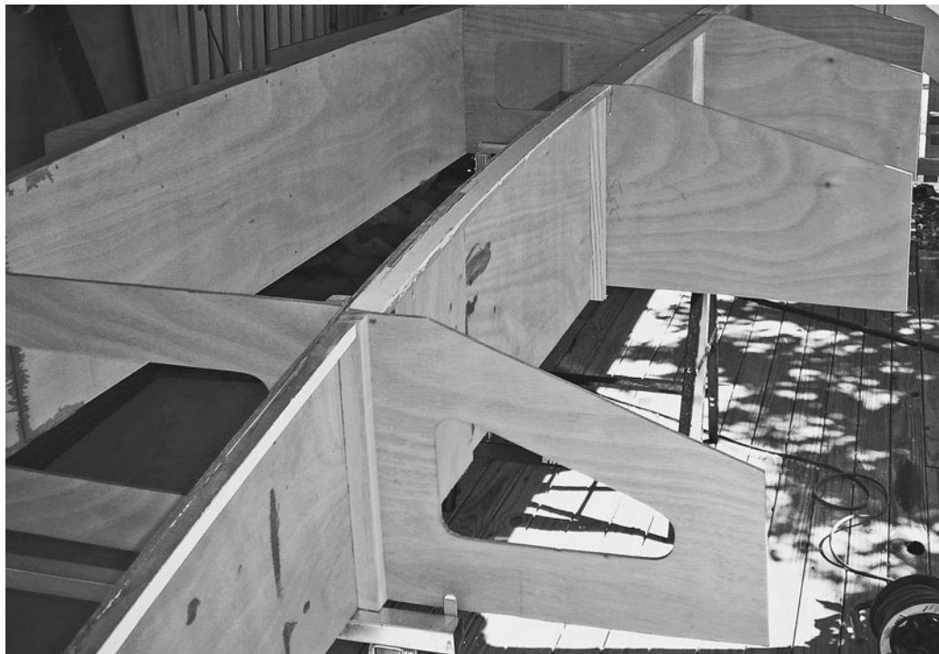
Dogsbody's "egg crate" structure provides a great deal of stiffness and a lot of enclosed buoyancy. Cleats have been added to the bottom edges of the longitudinal members to provide a secure nailing and gluing surface for the bottom. Note also the vertical cleats that hold the transverse members.
