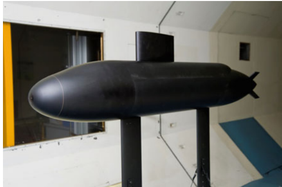
Fig. 4.27 Submarine model being tested for resistance in a wind tunnel (courtesy of DST Group)
