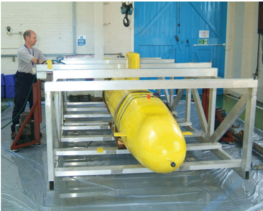
Fig. 3.54 Model being prepared using a compound pendulum to measure inertia (courtesy QinetiQ Limited, © Copyright QinetiQ Limited 2017)
