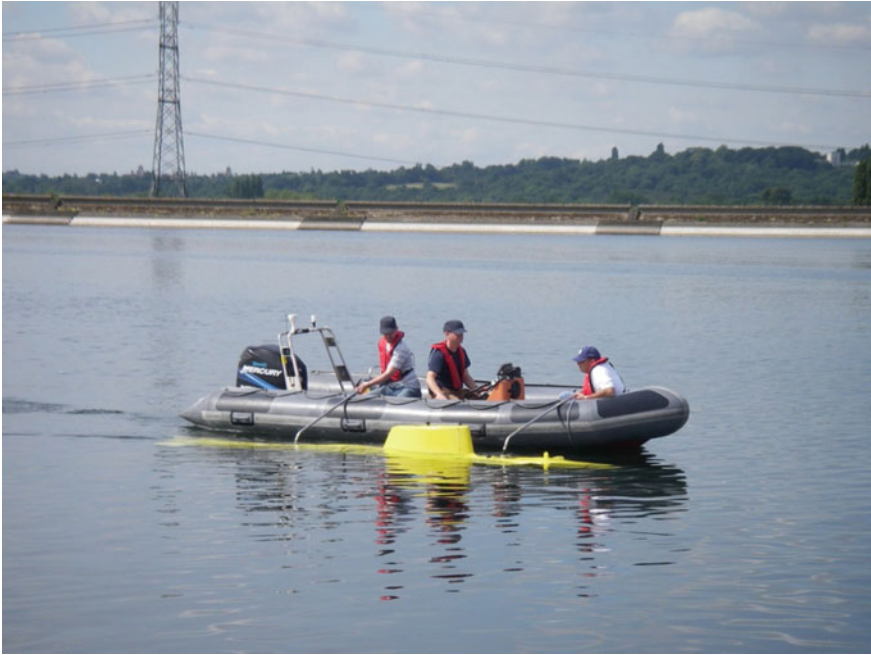
Fig. 3.55 Free running model being recovered by support boat in lake testing facility (courtesy QinetiQ Limited, © Copyright QinetiQ Limited 2017)
