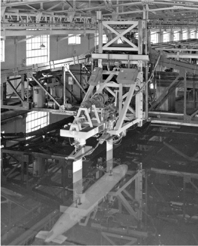
Fig. 3.8 Typical set up for captive model tests using a VPMM (courtesy QinetiQ Limited, © Copyright QinetiQ Limited 2017)
