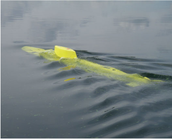
Fig. 4.22 Wave pattern generated by a submarine model with its sail above the surface (courtesy QinetiQ Limited, © Copyright QinetiQ Limited 2017)
