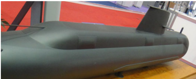
Fig. 4.10 Model showing casing on modern submarine
