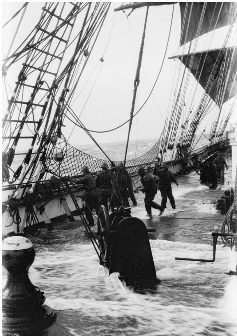
Wet work on the deck. Note the life-net, which prevents the crew from being washed overboard.
