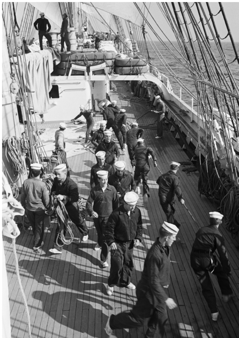
Running an upper halliard along the deck, for a livelier setting of the sail, on the U.S. Coast Guard's training barque Eagle .
