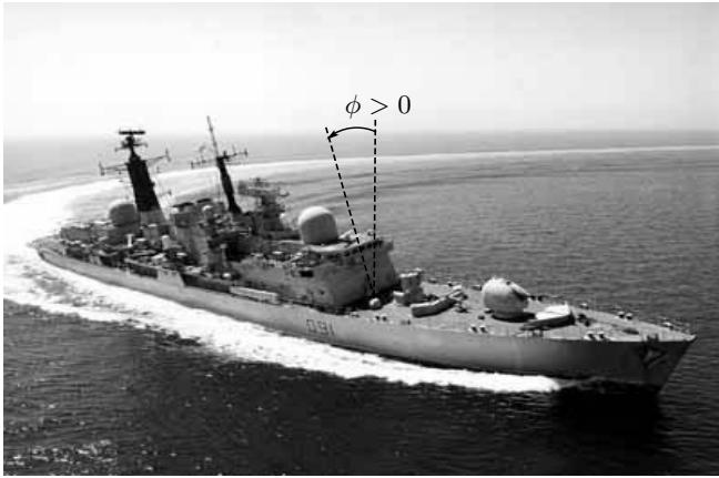
Fig. 8.4. Steady heel angle during a port turn of a Naval vessel. (©Crown Copyright/MOD. Reproduced with the permission of the Controller of Her Majesty's Stationery Office, United Kingdom.)
