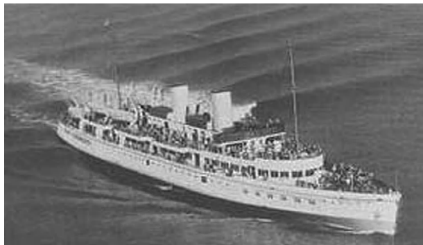
FIGURE 12.4(b) Photograph of the wave pattern developed by a ferry. Source Unknown.
