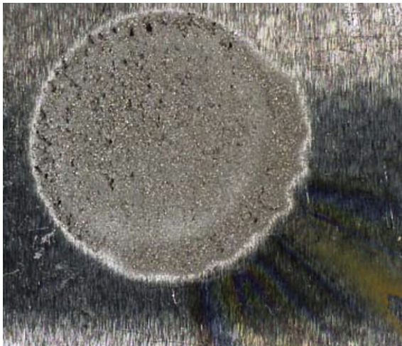
FIGURE 9.37 Oxide induced temper coloring on a mild steel specimen subjected to cavitation erosion attack.
