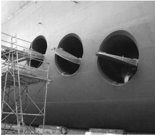
FIGURE 14.13 Doors fitted to a set of transverse propulsion unit openings.
