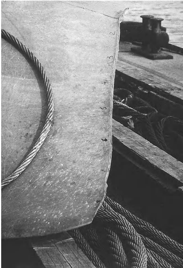
FIGURE 19.4 Propeller blade failure.
