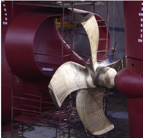
FIGURE 13.6 CLT Propeller fitted to a tanker with a wake equalizing duct mounted on the ship ahead of the CLT Propeller. Courtesy Sistemar
