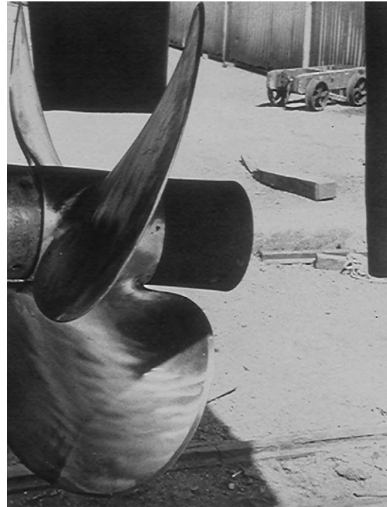
FIGURE 22.19 Truncated fairwater cone fitted to a high-speed patrol vessel.
